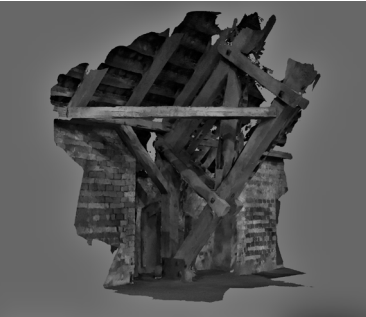
A 3d pointcloud scan of a fragment of a lower part of the truss captured on site for 3d model reference
