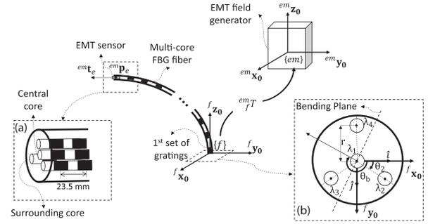
Fig. 1. Relation between EMT coordinate frame  $\{em\}$  and the FBG local coordinate frame  $\{f\}$  that is coincidentally fixed with the 1st set of gratings is shown in this figure. A side and a cross-section view of the multi-core FBG fiber can be seen in (a) and (b), respectively. The angle of the bending plane and the angle of the 2nd core with respect to the  $x$ -axis are denoted as  $\theta_b$  and  $\theta_2$  in (b), respectively.
