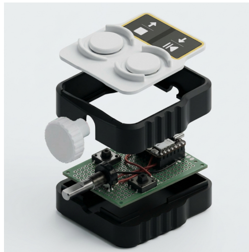
Figure 47: Exploded view of the remote control.
