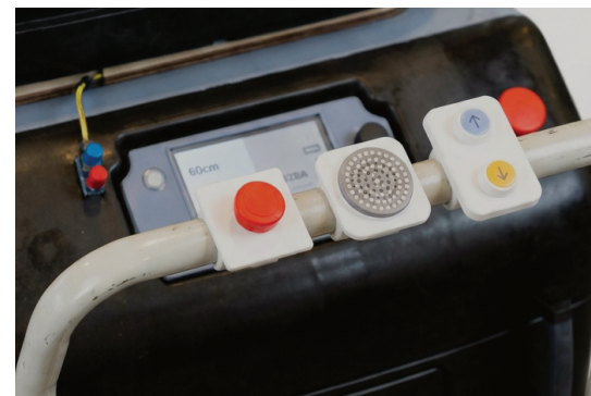
Figure 25: Mockup push button, microphone and display.
