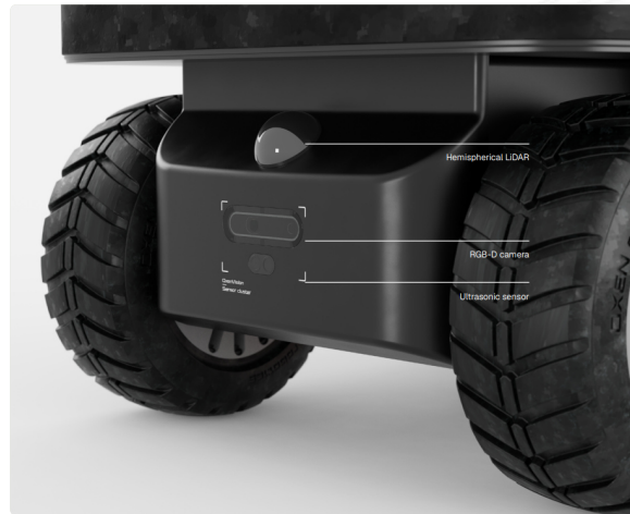
Figure 3: Drivetrain and sensors of prototype, by van Zoest [30]
