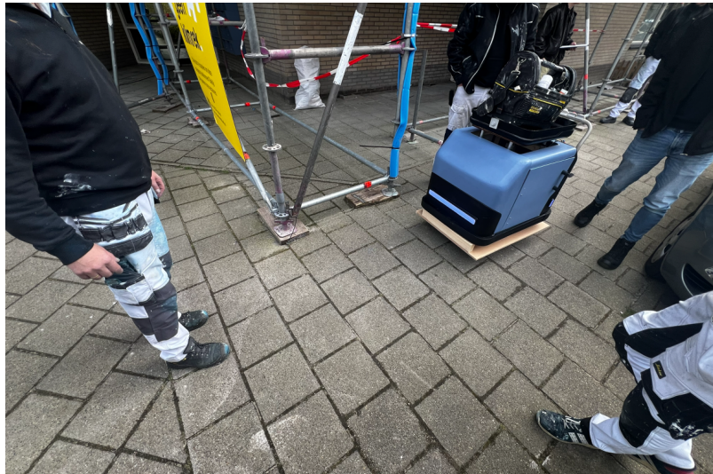
Figure 28: Prototype on cart being used in the field test
