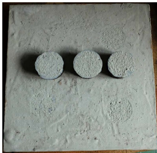
Fig. 6. Adhesion specimen after testing.
