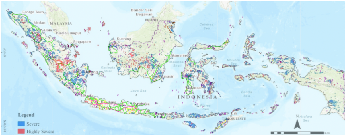
Figure 10.1: Spatial distribution of degraded lands suitable for bioenergy crop cultivation (Source: Jaung et al., 2018). The blue and red patches represent areas of severe, and highly severe degradation. This data is superimposed on the DGNREEC's OneMap which shows the electricity grid infrastructure, and diesel plants, which are shown by purple lightning bolts (DGNREEC, 2020).
