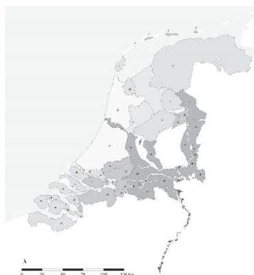
Figure 1: The flood exceedance probability of the Dike ring levee systems. (Source: Author, 2020) (Data source: Rijkswaterstaat, 2010.)
