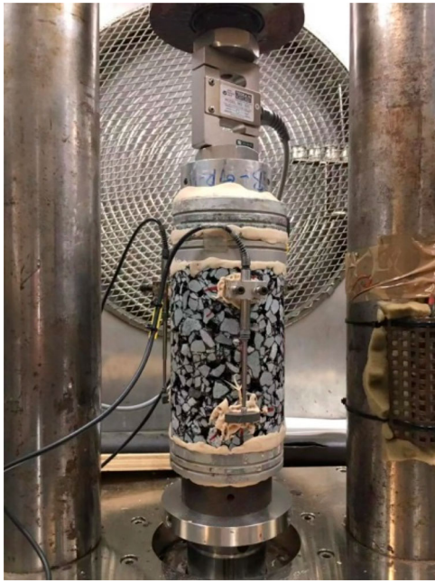
Figure 8. Setup for the uniaxial cyclic compressive test.
