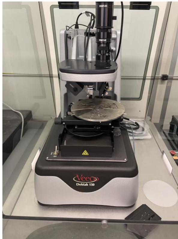
Figure 3.7: The interior of the Dektak profilometer, the sample is to be placed on the silver coloured disc and has to be manually put into position beneath the red needle.
