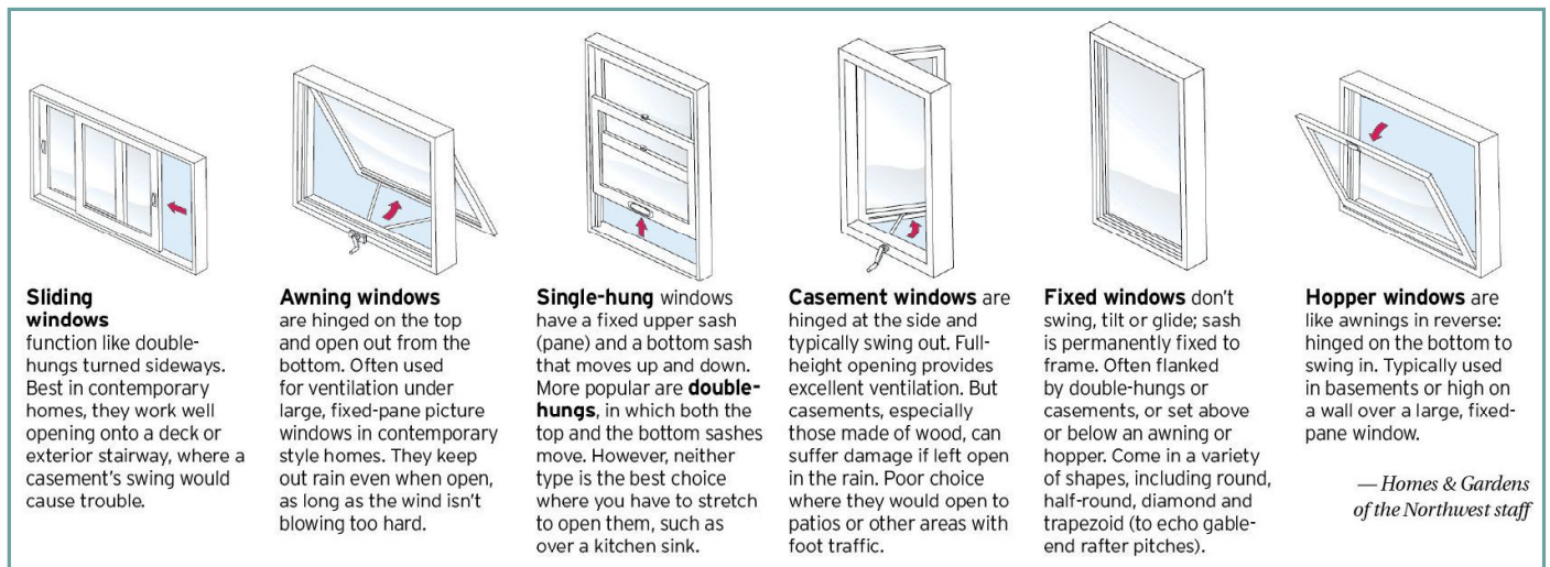
Figure 78; Know your window styles: Sliding, awning, single-hung, double-hung, casement, fixed and hopper (Oregonian, 2012).
