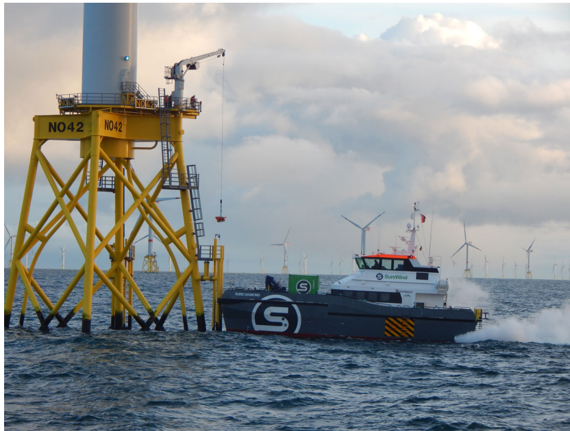
Figure 1.2: A crew transport vessel positioning itself to a wind turbine (Taken from [16])
