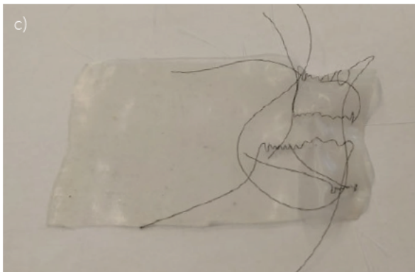
Figure 9.4 Connection of SMA wire to Dragon Skin silicone with: a) Tesa extra power tape b) Aluminium tape and c) machine stitching.
