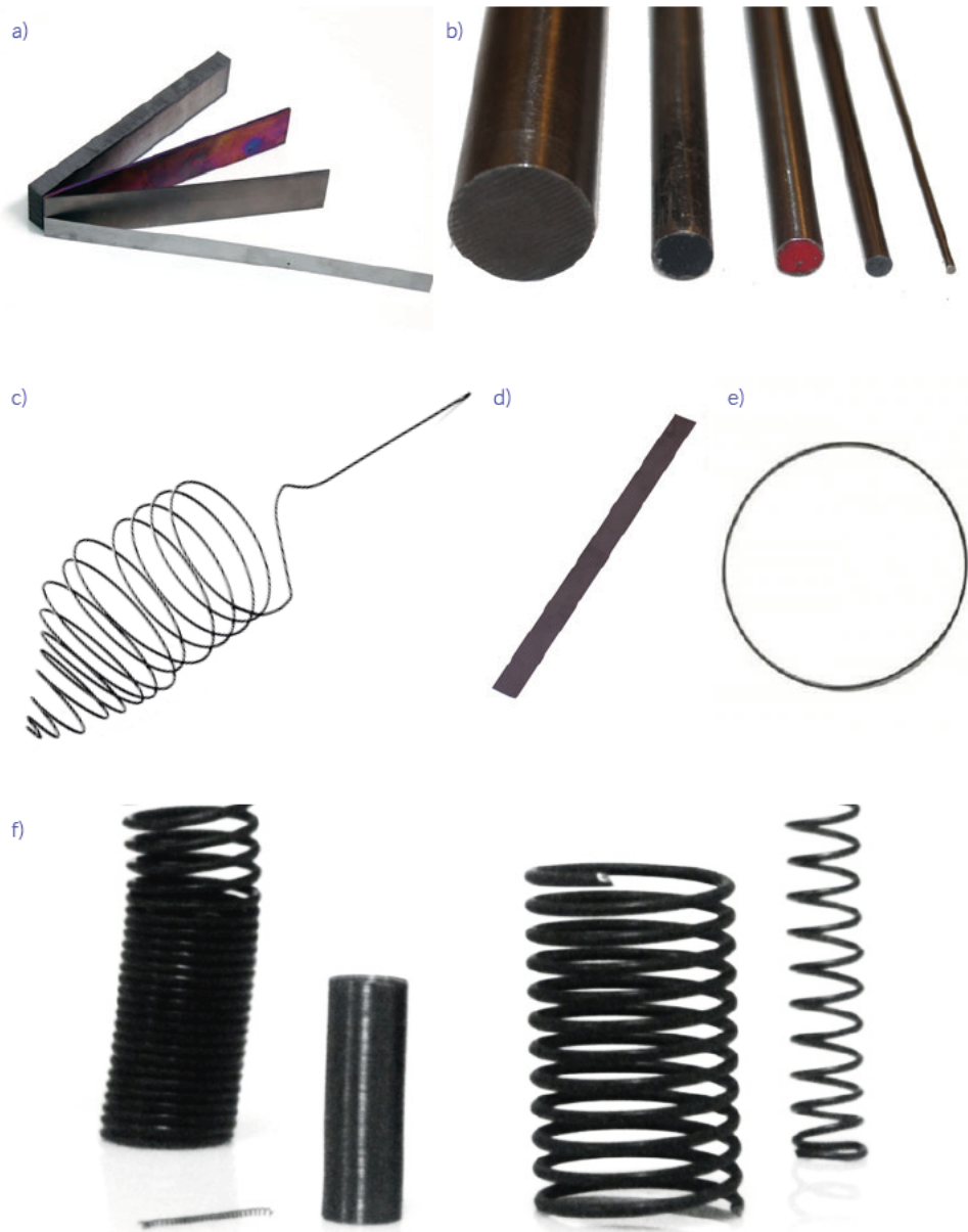
Figure 3.3 Shape memory Alloy manufactured to different configurations: a) plate b) rod c) wire d) flat wire e) welded loop f) springs with different wire diameter and mean diameter.
