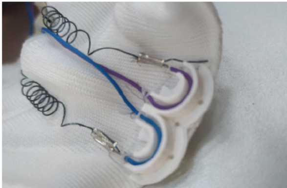
Figure 12.7 Wire holder sewn inside the material structure.
