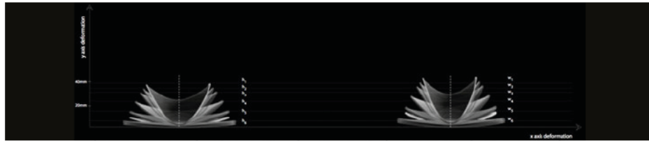
Figure 7.3 Sample curvature change by incremental change (0.5mm) of height (left) and width (right) of the pattern print (Papakonstantinou, 2015).
