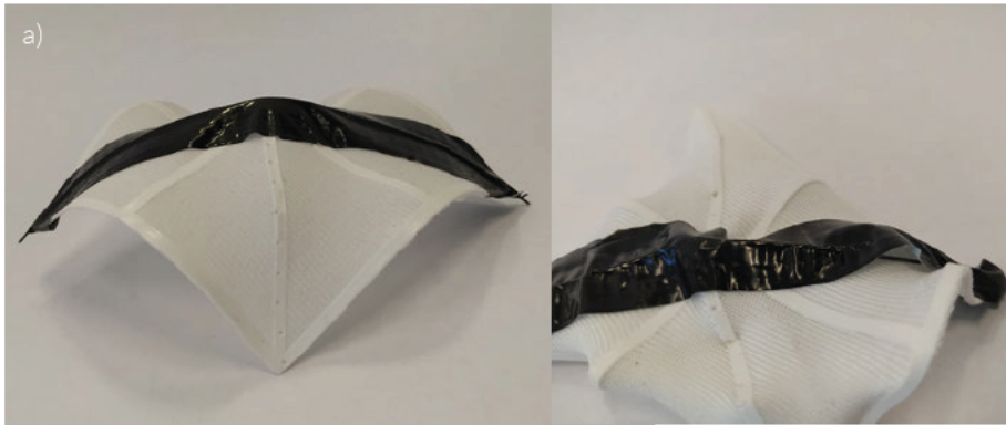
Figure 9.2 Connection of SMA wire to the 4D printed structure with: a) Tesa extra power tape b) Aluminium tape c) the reshaping of the PLA along the SMA wire.
