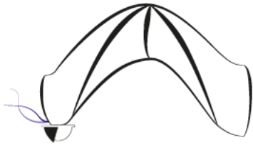
Filament material 1: PLA Friction Foot: Big Configuration: Friction foot at electrical wires, 0°
