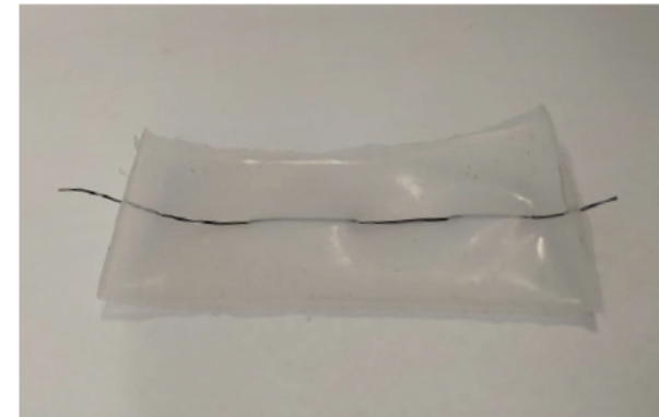
Figure 9.5 Connection of SMA wire to Dragon Skin Silicone by: a) weaving the SMA inside the material and b) by first attaching the SMA wire inside the mold before the silicone is casted which results in an c) embedded sample
