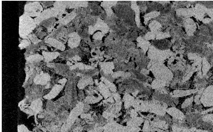
FIGURE 6.24: Micro CT scan of limestone core, before LSF.
