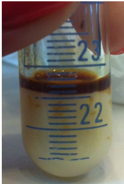
FIGURE 7.5: Sample of the effluent during both oil and water production, 2000 ppm NaCl, 50 °C, limestone core.
