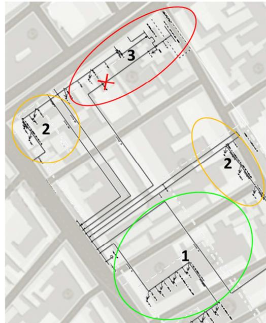
**Figure B Hypothetical guideline to be created by network operators. Guideline shows capacity of grid branches to deal with additional load of charging stations, where 1. indicates no problems, 2. indicates that a limited capacity increase is possible and 3. indicates that reinforcements are required when installing charging stations.**
