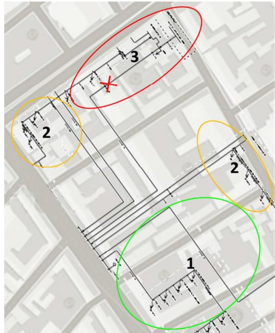
**Figure 41 Hypothetical guideline to be created by network operators. Guideline shows capacity of grid branches to deal with additional load of charging stations, where 1. indicates no problems, 2. indicates that a limited capacity increase is possible and 3. indicates that reinforcements are required when installing charging stations.**
