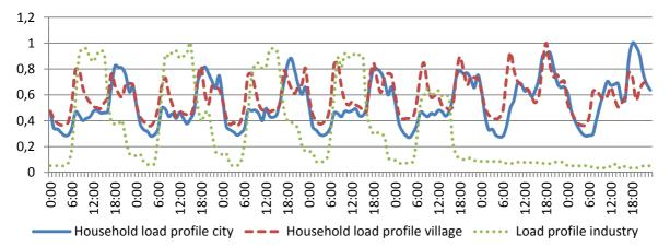
Figure 12 An average load profile of a household in a city or village, and an average load profile for industry [Vision network analysis, 2011].
