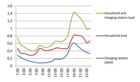
Figure 14 Charging and household load, individual and combined profiles for an average day. The load peaks occur at about the same time [Verzijlbergh, 2011].
