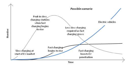
Figure 16 A possible charging scenario of TNO and Innopay, where fast charging becomes the main charging facility [Boekema et.al., 2010]. The scenario merely describes the concept, not the time frame or expected number of vehicles, thus scales the axes in the figure are undefined.
