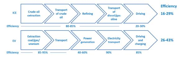
Figure 6 Well-to-wheel efficiency of ICE and electric vehicle [Knigge, 2011].
