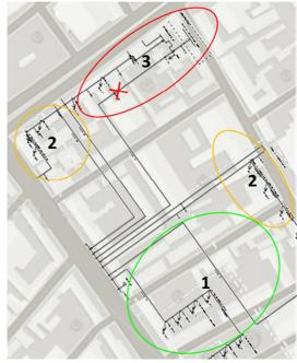
Figure 37 Hypothetical guideline to be created by network operators. Guideline shows capacity of grid branches to deal with additional load of charging stations.
