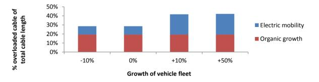
Figure 24 Case 4: Impact of a smaller or larger total vehicle fleet, assuming 100% electric vehicle adoption. A small increase of 10% of the total vehicle fleet shows a large increase in overloaded grid components.
