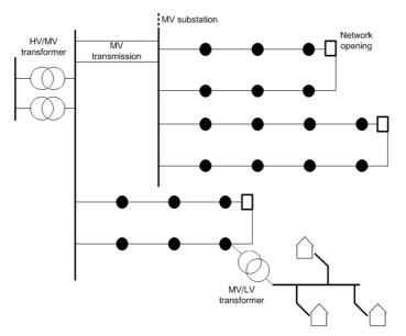
Figure 8 Network structure, showing a grid from a high voltage to medium voltage transformer to a low voltage household network [Adjusted from Grond, 2011].
