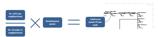
Figure 20 Steps for determining the additional power due to electric mobility. This additional power is included in the grid model.
