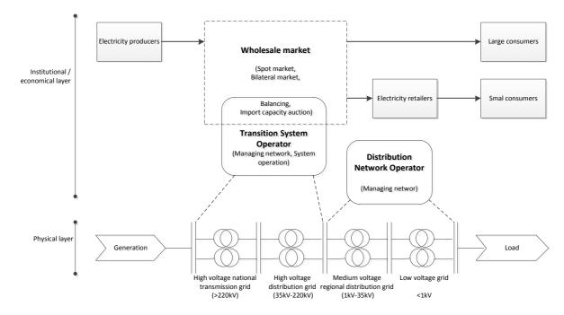
Figure 7 The Dutch power system, displaying the physical electricity grid with generation and load, and the institutions and markets involved in the electricity system [based on de Vries et.al., 2009; Karatay et.al., 2010].
