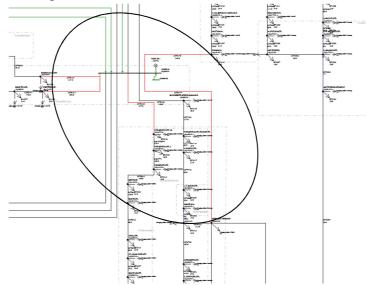
Figure 22 Screenshot of Utrecht sub-model after grid impact calculations for case 2. The red lines in the circle show the cables which are loaded above 100%. These overloaded cables are located at the beginning of branches.
