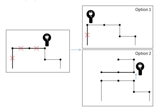
Figure 30 Two options to change the location of high power charging stations based on grid capacity. In the first option the charging station is located towards the beginning of the grid branch thereby limiting the amount of grid components to be reinforced. In the second option the charging station is connected to a nearby grid branch with sufficient capacity.
