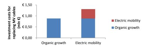
Figure 29 Investment costs for replacing medium voltage cables in the Utrecht sub-grid, investments costs for grid reinforcements rise up to €1,3 million.
