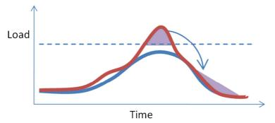
Figure 15 Load shaving showing the smart charging concept. Load at the peak can be displaced to off-peak demand hours.
