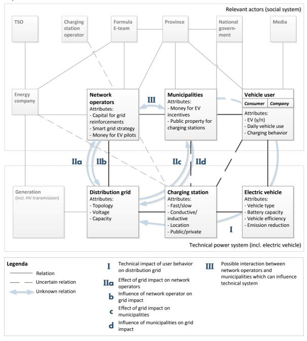
Figure 18 System diagram displaying the decomposition of the technical power system and the relevant actors. The colour of the blocks and arrows display whether the component is in (black) or outside (grey) the project scope.
