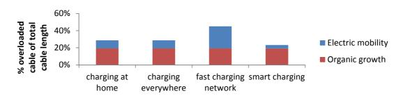
Figure 26 Case 6: Impact of different charging scenarios. Fast charging can have a large impact on the grid. Smart charging reduces the impact.
