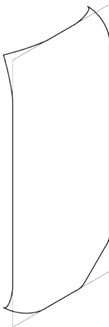
Figure 88-Corner bending movement scheme.
