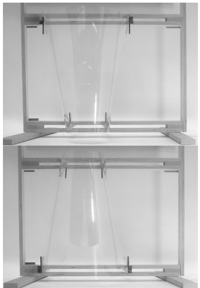
Figure 82-Asymetric movement. Different radius on the top and bottom edge.
