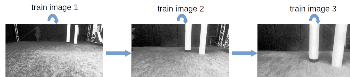
Figure 8.5: Scene familiarity based neural network training procedure. Image 1 is shown, after which the weights are adapted. Next, image 2 is presented to the network and the weights adapted, and so on.
