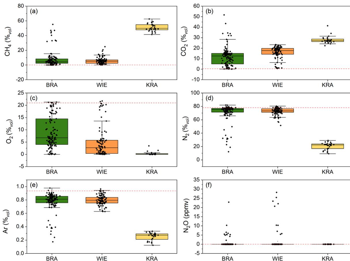
Fig. 1. Composition of landfill gas from pilots Braambergen (BRA), Wieringermeer (WIE) and Kragge (KRA). Box = 25th-75th percentile, line = mean, whiskers = 10th-90th percentile. The red dotted line presents expected atmospheric concentrations.
