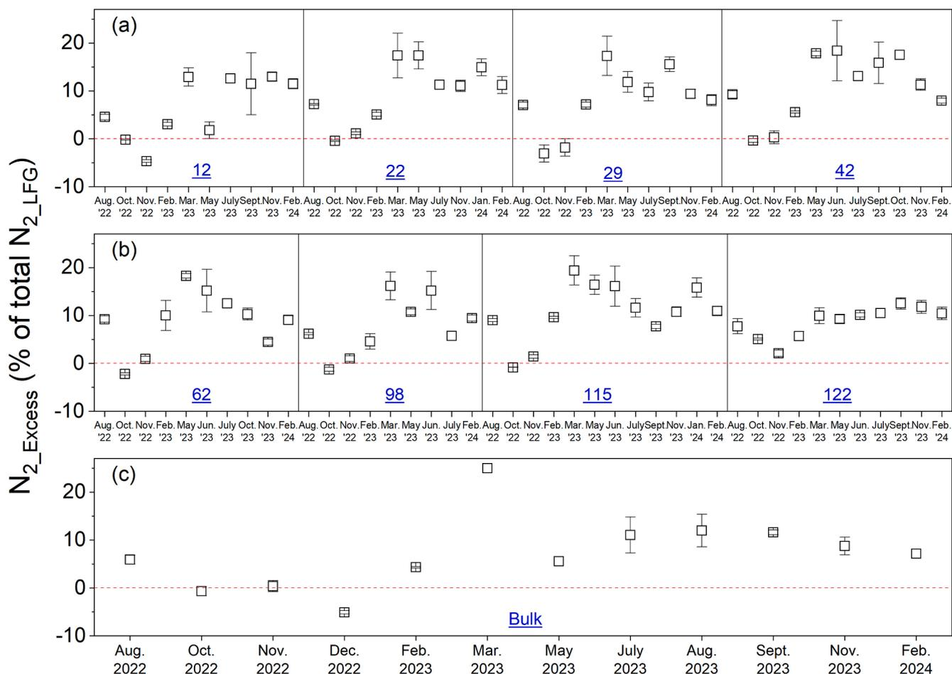
Fig. 5. Spatial and temporal differences of mean  $N_{2\_Excess}$  (% of the total  $N_{2\_LFG}$ ) in landfill gas (Eq. 3) from Wieringermeer (WIE). Blue underlined text = sample ID (for sampling location see Table S2 in Supporting Information). Error bars = standard errors.
