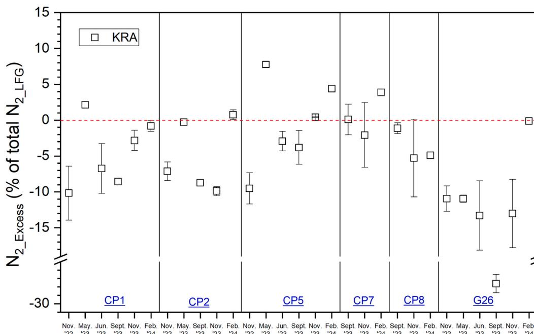
Fig. 6. Spatial and temporal differences of mean  $N_{2\_Excess}$  (% of the total  $N_{2\_LFG}$ ) in landfill gas (Eq. 3) from Kragge (KRA). Blue underlined text = sample ID (for sampling location see Table S2 in Supporting Information). Error bars = standard errors.
