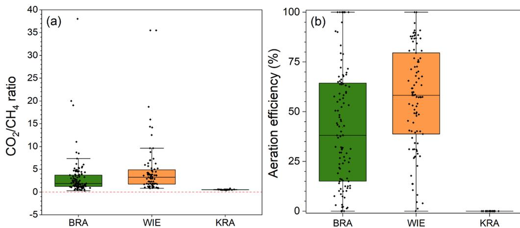
Fig. 2. (a) Ratio of  $\text{CO}_2$  to  $\text{CH}_4$ ; (b) aeration efficiency (Eq. 1) in landfill gas from pilots Braambergen (BRA), Wieringermeer (WIE) and Kragge (KRA). The red dotted line represents expected ambient concentrations.
