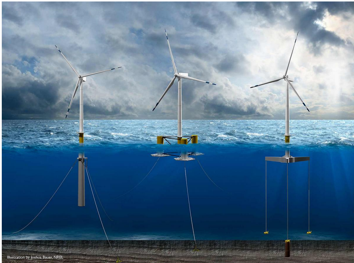
Figure 1.1: Classifications for three floating wind foundations. Left a spar, middle a semi-submersible and right a tension-leg platform (Bauer, 2017).
