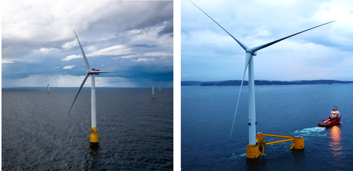
Figure 1.5: Upscaled FOWTs, left the 6 MW Hywind Scotland spar by Equinor (2017) and right the 8.3 MW WindFloat Atlantic semi-submersible by Principle Power (2019).
