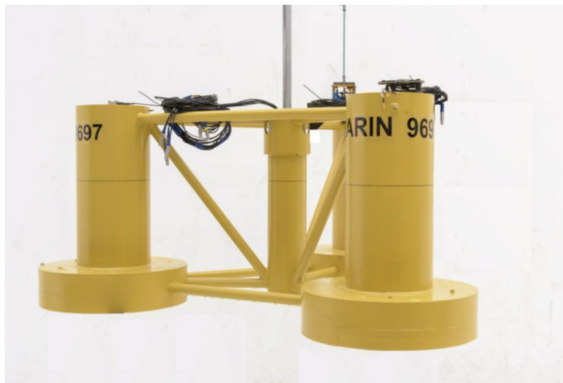
Figure 5-9: OC6-DeepCwind floating platform, used in the experimental test.
