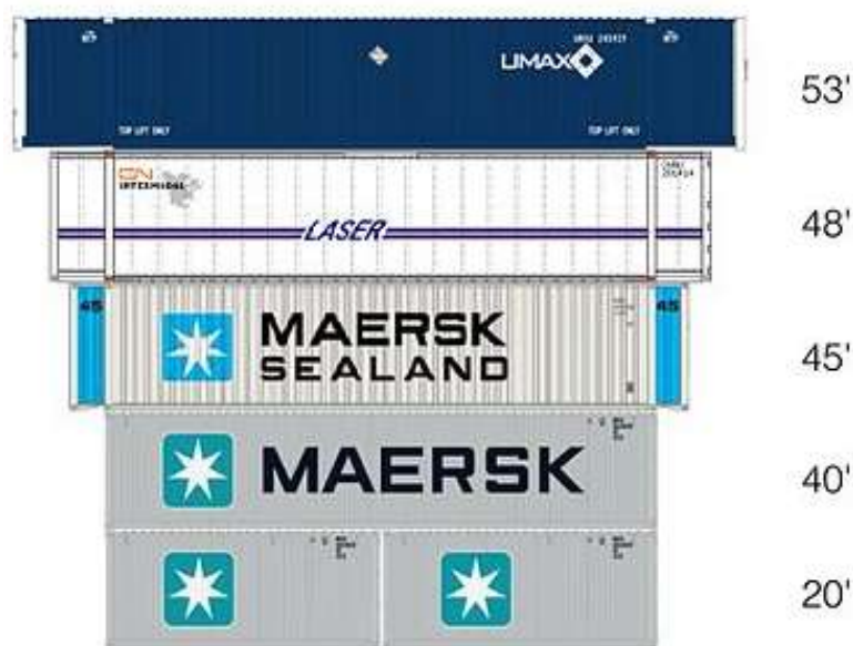
Figure 4: Twenty-foot equivalent unit 3
