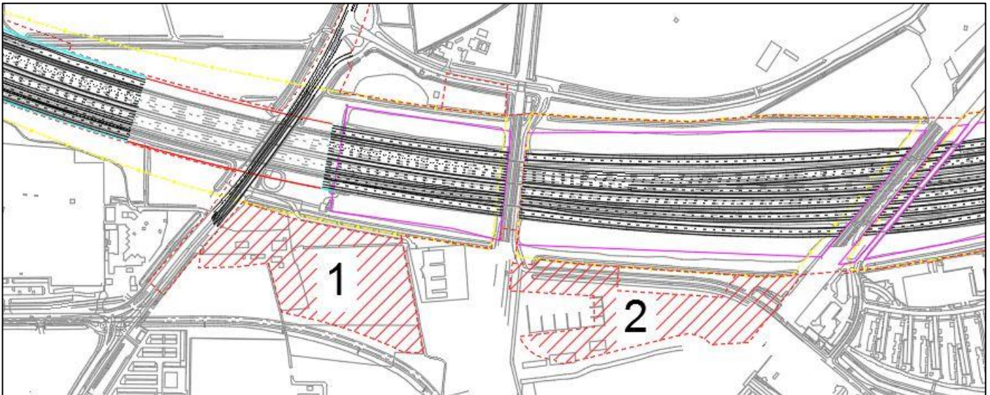
Figure 5.3: A digital 2D overview of Figure 5.2 with the two appointed construction sites, the new intended situation [40].
