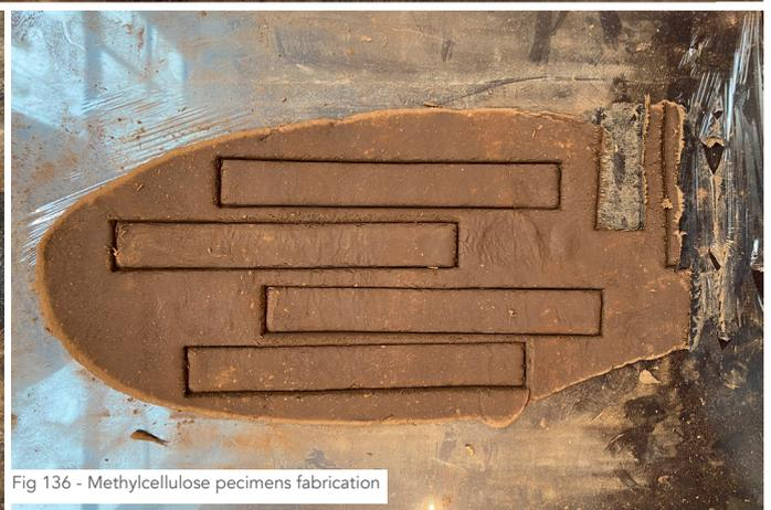
Fig 136 - Methylcellulose pecimens fabrication
