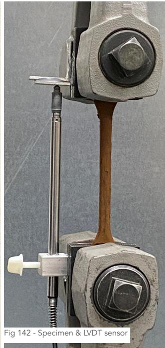
Fig 142 - Specimen & LVDT sensor
