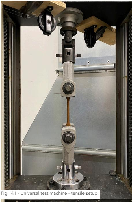
Fig 141 - Universal test machine - tensile setup
