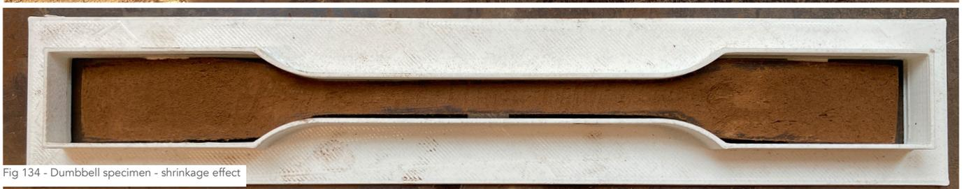
Fig 134 - Dumbbell specimen - shrinkage effect
