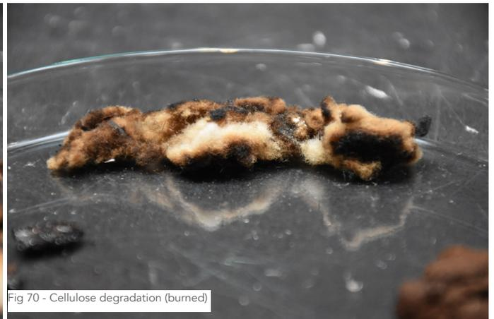
Fig 70 - Cellulose degradation (burned)
