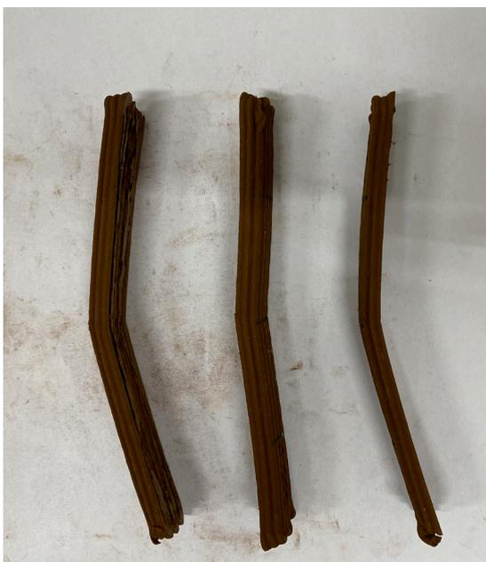
Fig 165 - MC extruded beam specimens - after
