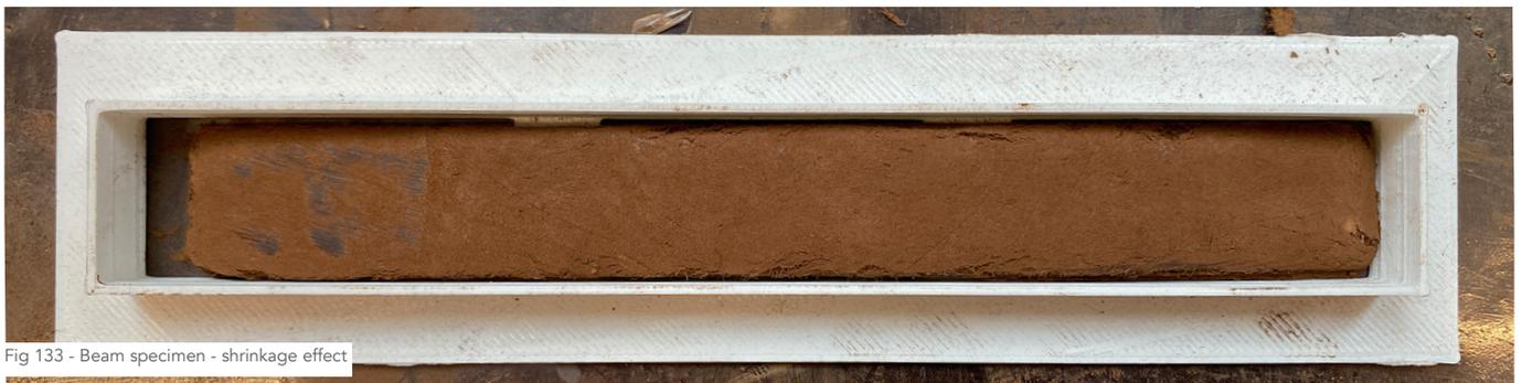
Fig 133 - Beam specimen - shrinkage effect
