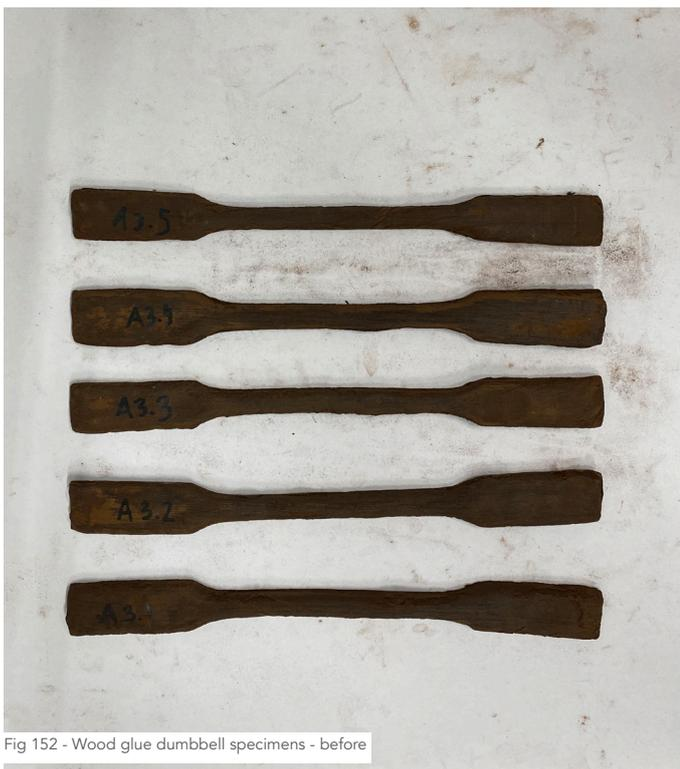
Fig 152 - Wood glue dumbbell specimens - before
