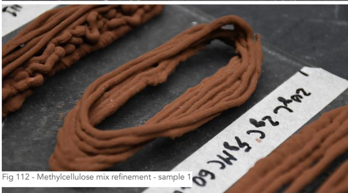
Fig 112 - Methylcellulose mix refinement - sample 1
