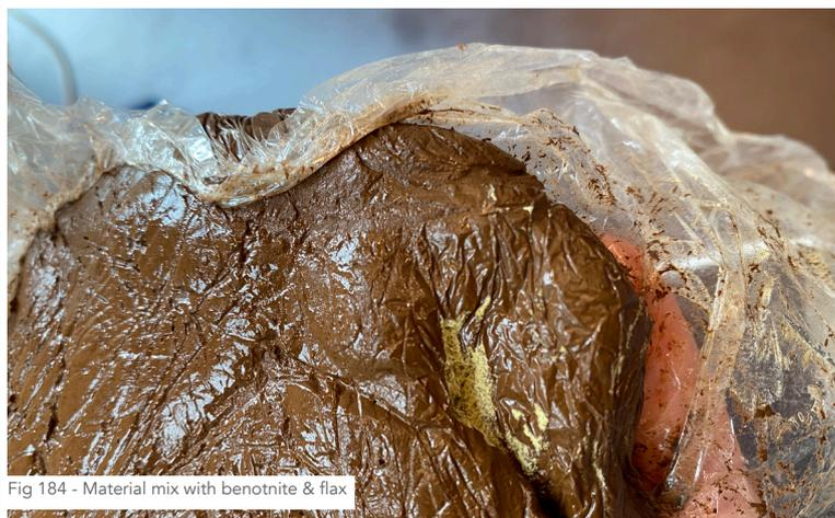
Fig 184 - Material mix with bentonite & flax
