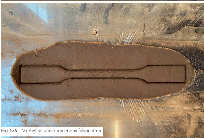
Fig 135 - Methylcellulose pecimens fabrication
