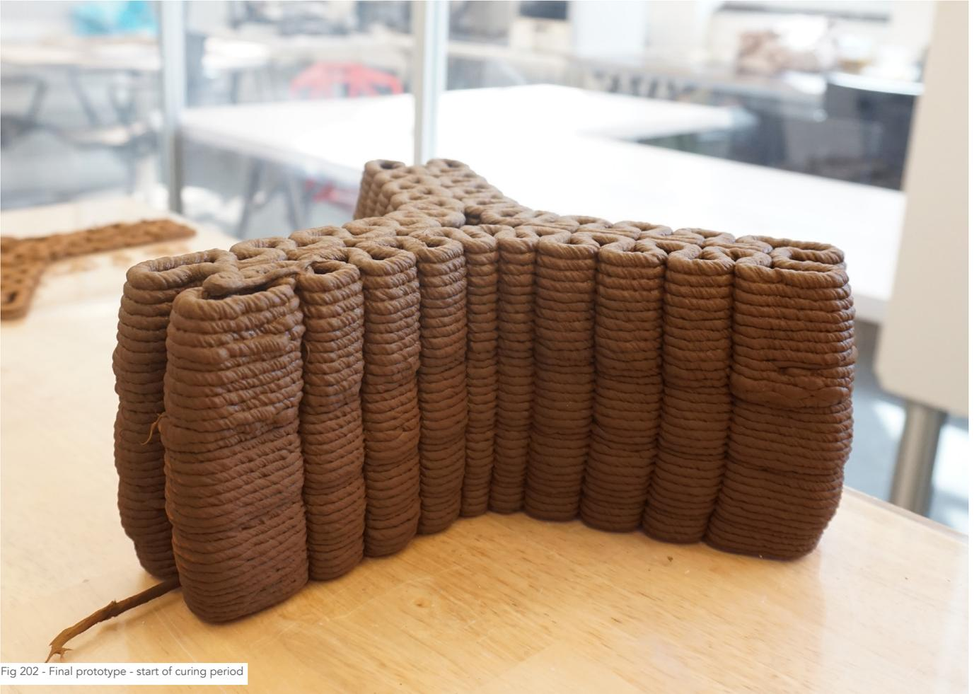
Fig 202 - Final prototype - start of curing period
