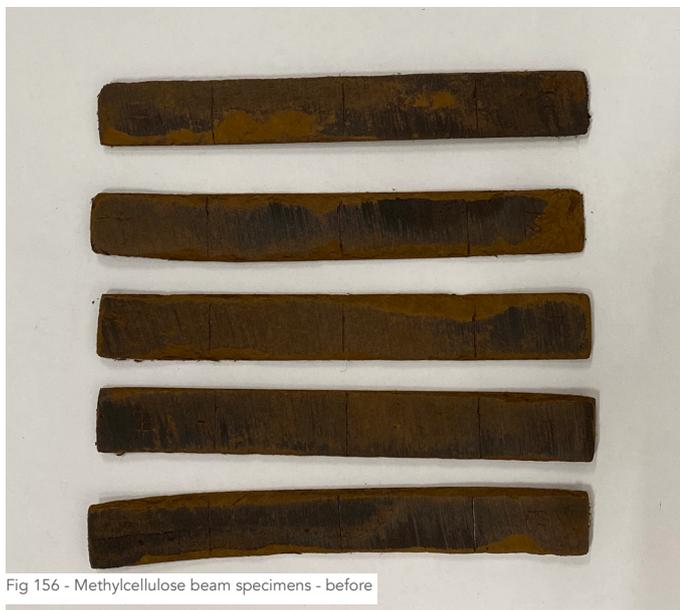
Fig 156 - Methylcellulose beam specimens - before
