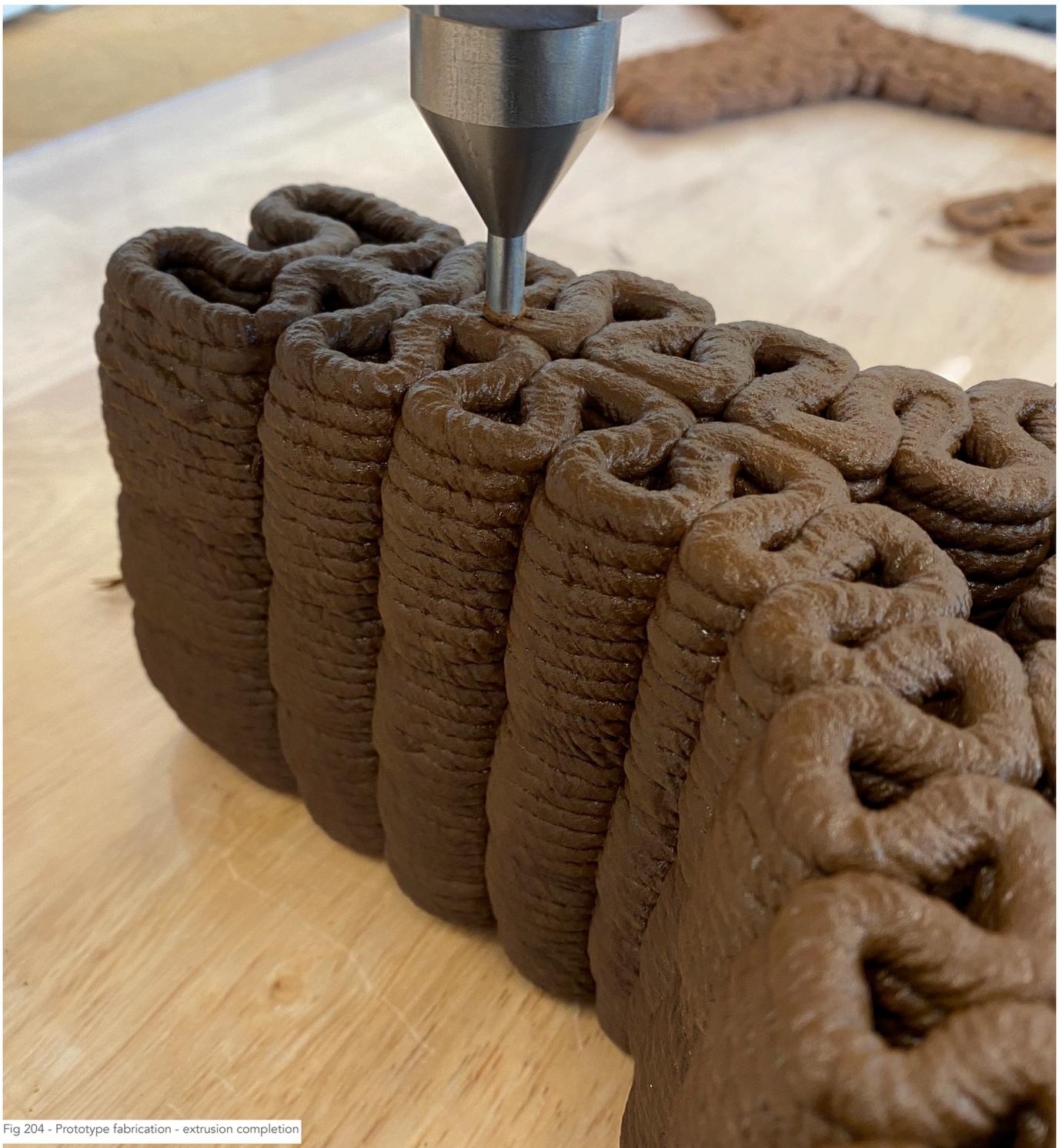
Fig 204 - Prototype fabrication - extrusion completion
