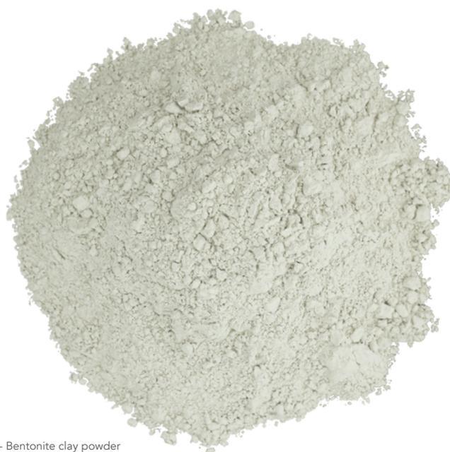
Fig 183 - Bentonite clay powder
