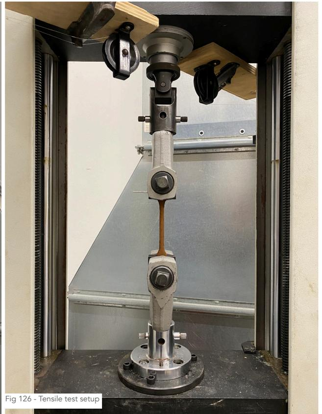
Fig 126 - Tensile test setup
