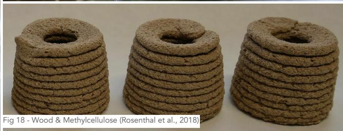
Fig 18 - Wood & Methylcellulose (Rosenthal et al., 2018)
