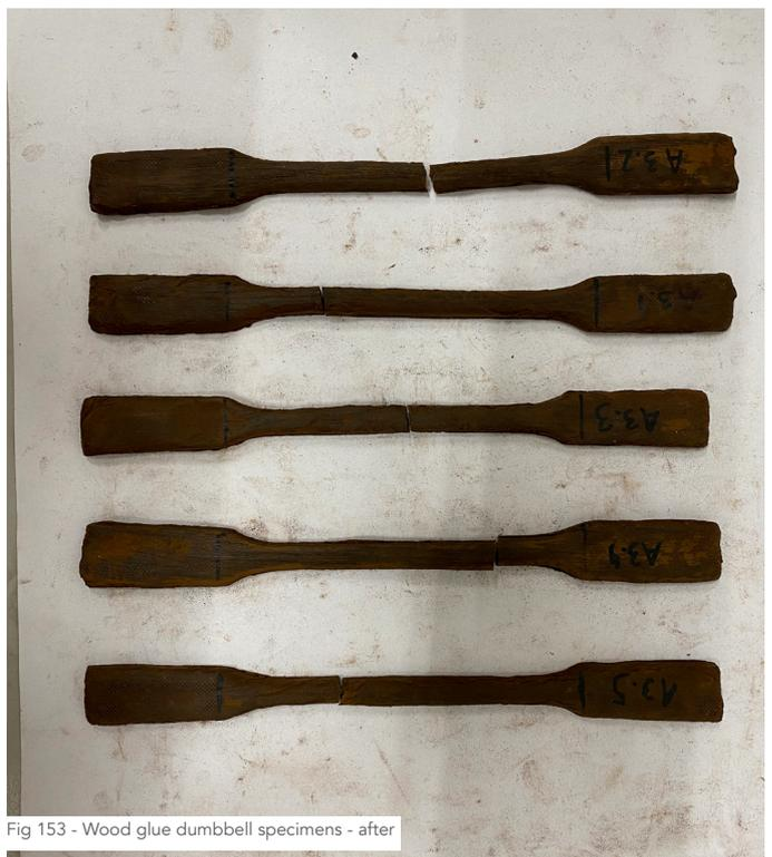
Fig 153 - Wood glue dumbbell specimens - after
