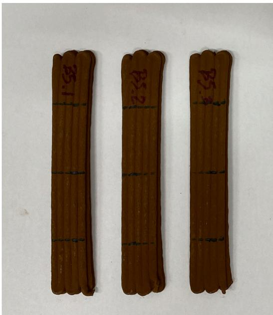
Fig 163 - MC extruded beam specimens - before
