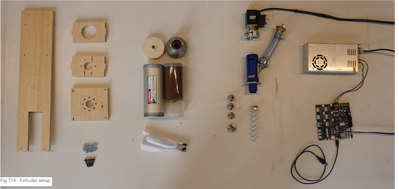
Fig 114 - Extruder setup
