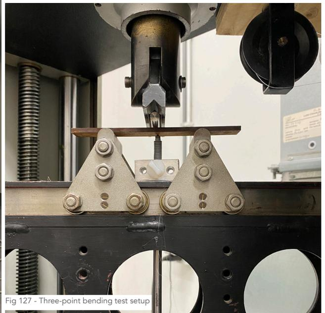
Fig 127 - Three-point bending test setup
