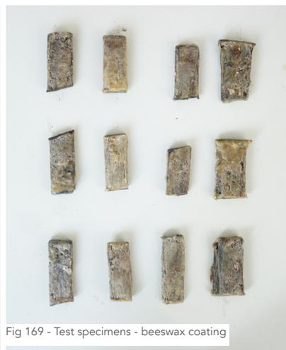
Fig 169 - Test specimens - beeswax coating
