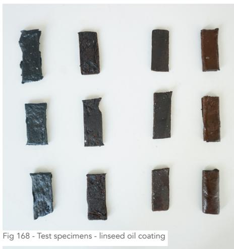
Fig 168 - Test specimens - linseed oil coating
