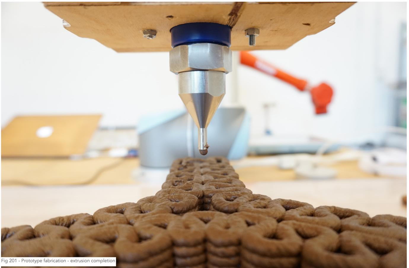
Fig 201 - Prototype fabrication - extrusion completion
