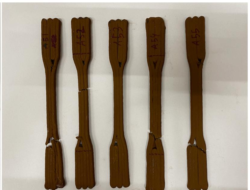
Fig 166 - MC extruded dumbbell specimens - after
