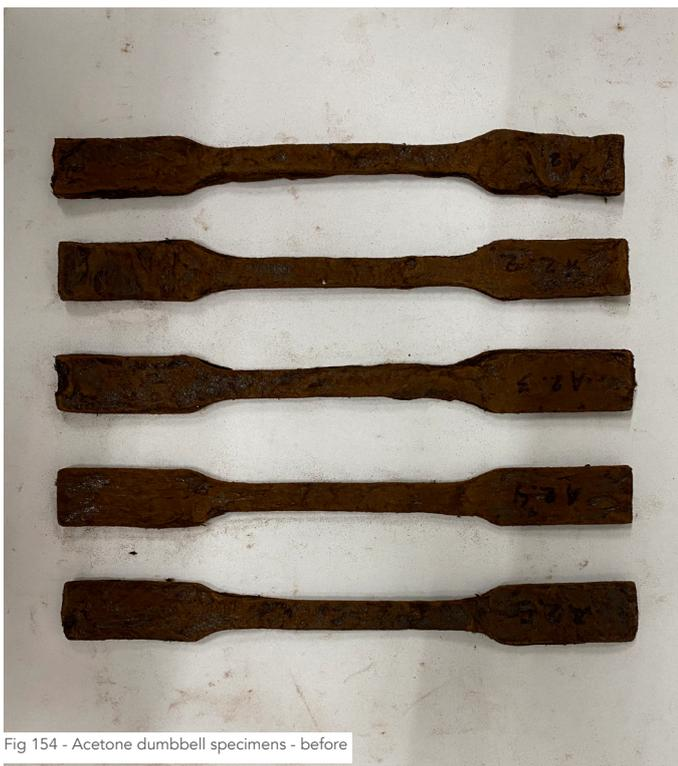
Fig 154 - Acetone dumbbell specimens - before
