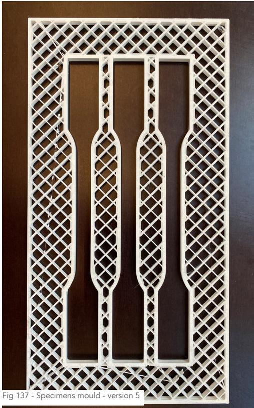
Fig 137 - Specimens mould - version 5
