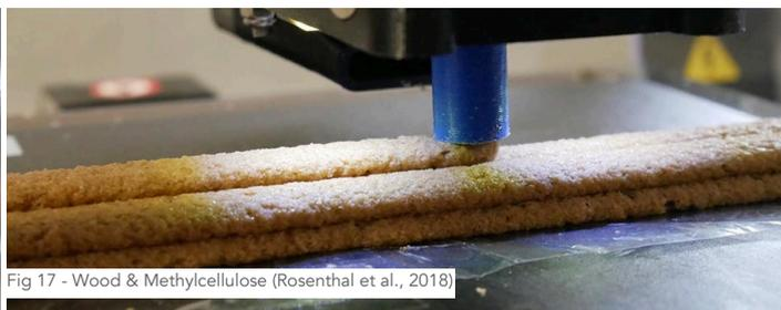
Fig 17 - Wood & Methylcellulose (Rosenthal et al., 2018)
