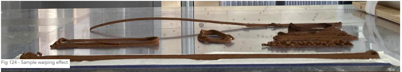
Curing conditions collaborated with the deformations. Samples dried from top to bottom due to uneven distribution of heat and ventilation of the environment. The ideal hardening process would be done on a mesh, elevated from the surface to create a circular air flow in a full-controlled environment in terms of humidity, temperature and ventilation.
