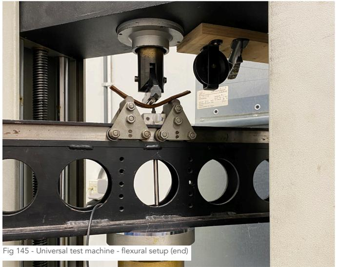
Fig 145 - Universal test machine - flexural setup (end)
