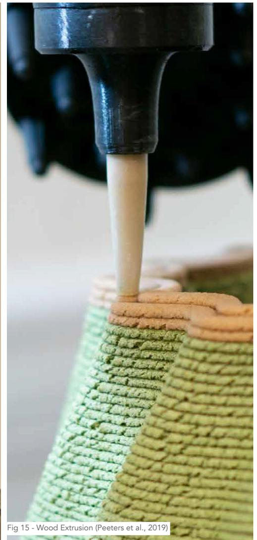
Fig 15 - Wood Extrusion (Peeters et al., 2019)
