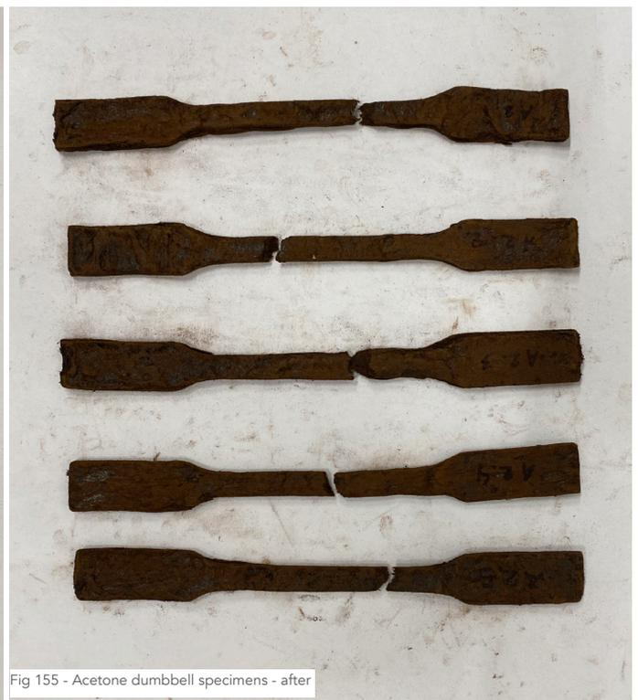
Fig 155 - Acetone dumbbell specimens - after
