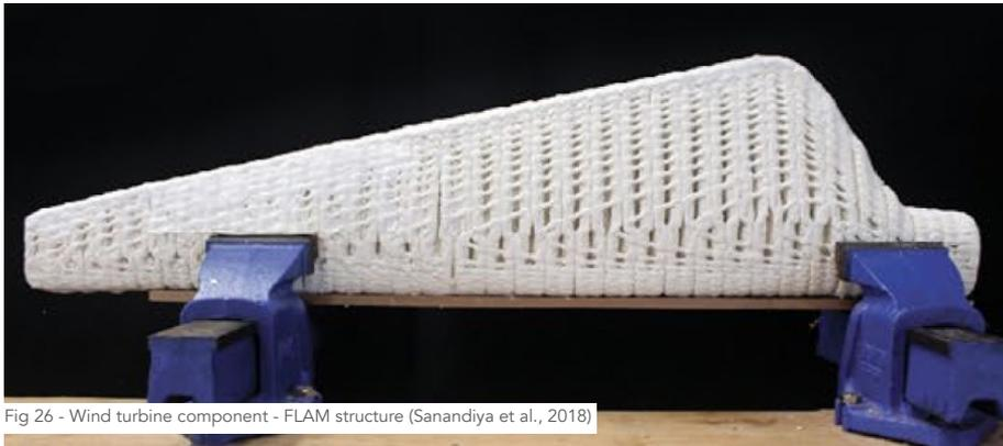
Fig 26 - Wind turbine component - FLAM structure (Sanandiyaya et al., 2018)
