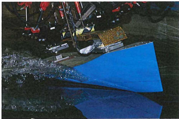
Figure 3: Model Concept 2 mounted under 6 DOF oscillator
