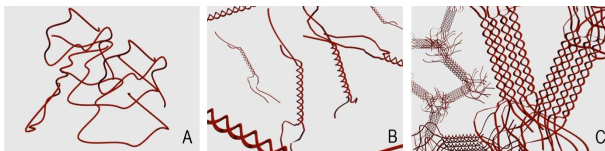
Figure 19 Gelation principle gellan gum. A: Random coils, B: Double helix formation, C: Junction zone assembly, retrieved from [50]
