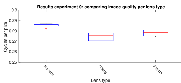
Figure 3.1: Difference in sharpness between images without a lens and with the glass- and the pmma lenses.
