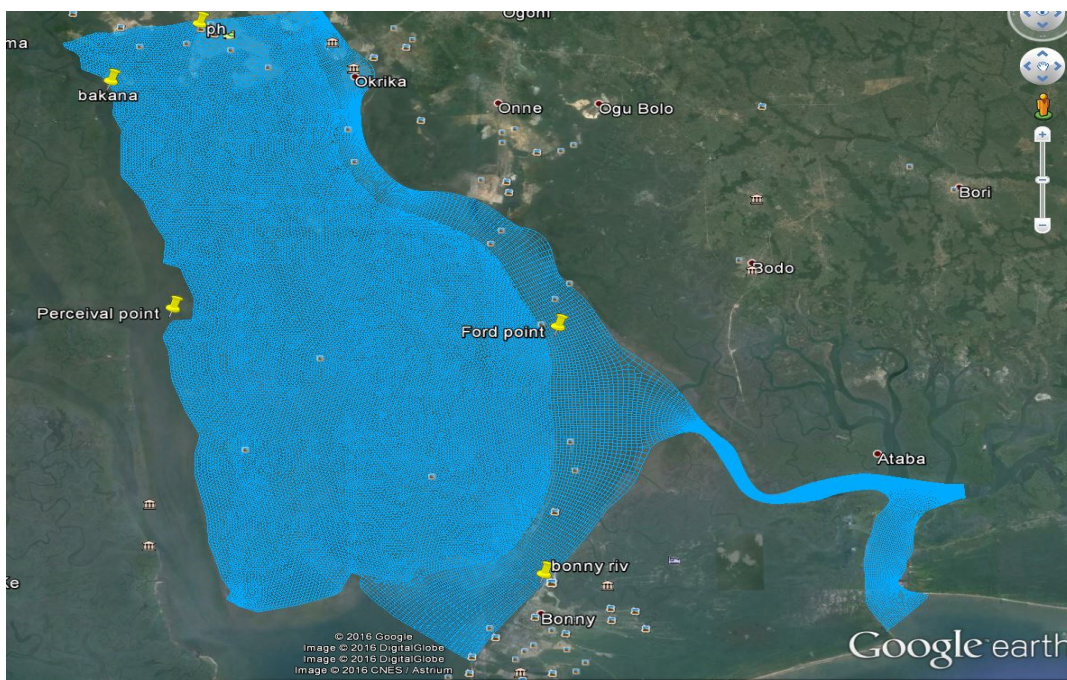
Figure 4.11. Unstructured grid created for Bonny - New Calabar River opened on Google earth image of the Niger delta. Yellow points show tide gauge locations.
