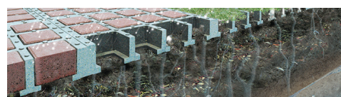
Figure 3.38 - TTE Infiltration system
