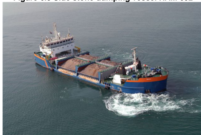
Figure 6.5 Side stone dumping vessel HAM 602
