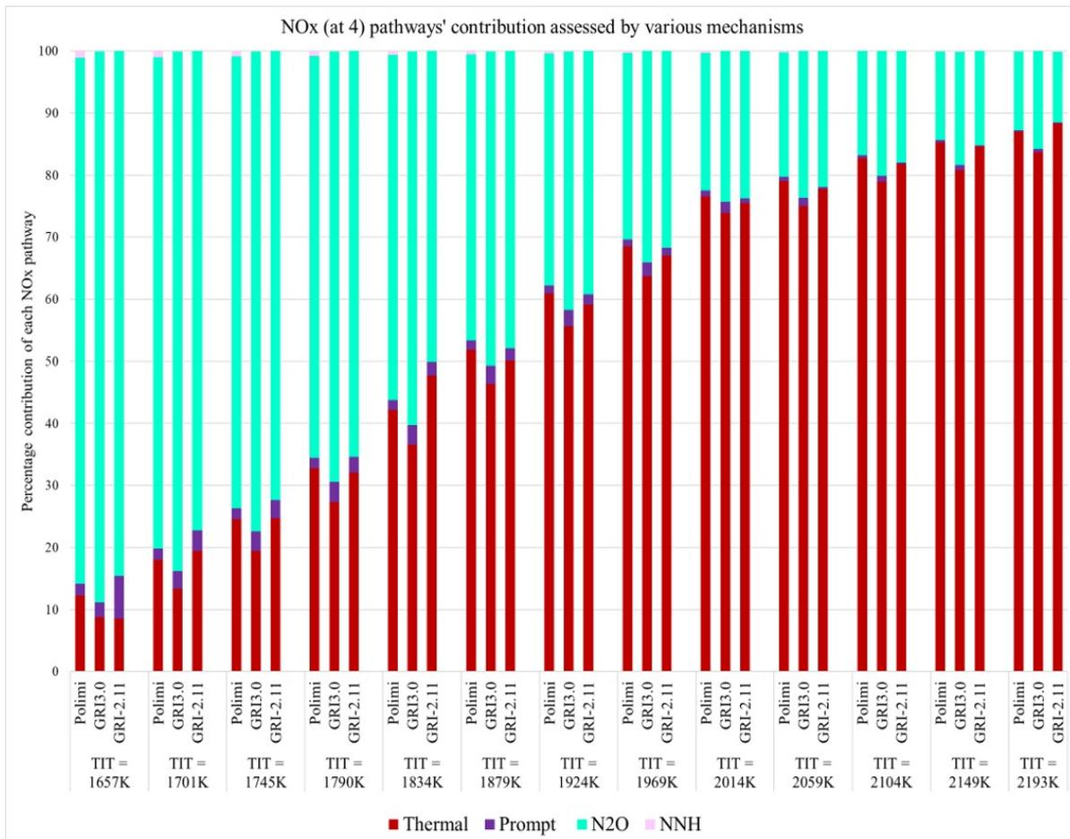
**Figure 4.20:** Relative contribution of NOx pathways at the combustor exit/stator inlet with TIT, as estimated by three different mechanisms
