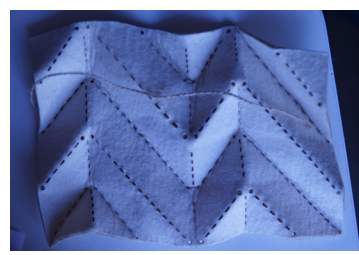
fig.x: 3mm felt cut in two ways (left two) and five mm felt, cut and measured to determine shrinking of the surface with the applied folds (right two)
