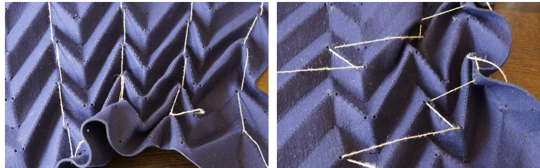
Fig.x: The vertical strings (left), made the screen easier to fold and caused less stress on the screen than the diagonal strings (right). However folding with both systems was difficult and cause too much stress to the screen that it influenced the feeling of reliability of the screen
