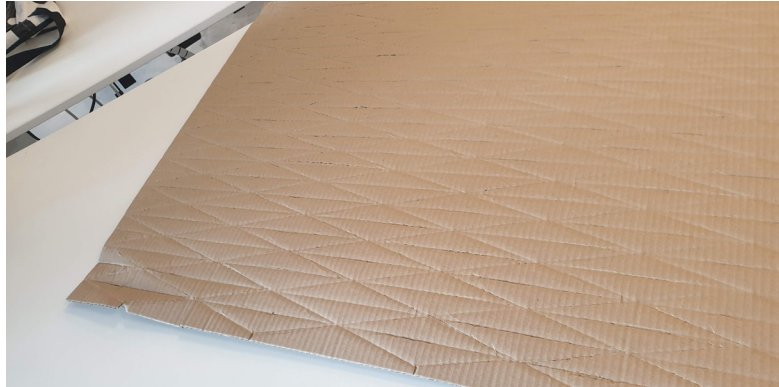
fig.x: cutting cardboard could not provide the needed flexibility to bend over and over.
