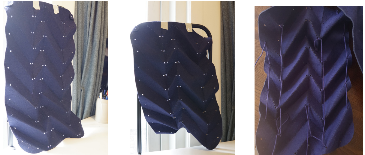
Fig.x: Left: the strap system. Right the vertical string system. The weight of the screen means that the strap system alone could not provide the desired textural quality, which the string systems could deliver.
