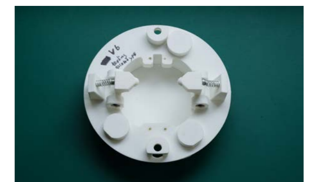
V6. Prototype used in first locking mechanism tests
