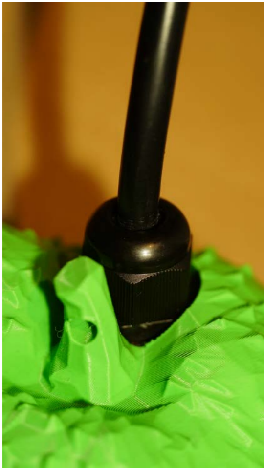
Figure 71 - Cable through cable gland
