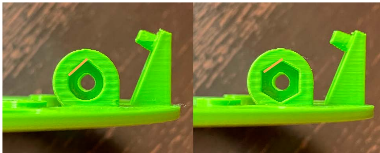
Figure Q4. Teardrop shape and angled top of the nut insert for supportless printability
