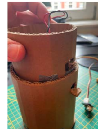
Click bottom onto top over the latch mechanism of the solenoid
