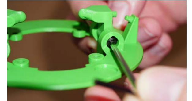
Screw the latch in place, repeat for the other latch at the other side of the top circle. Make sure not to screw it too tight as the latch needs to move freely.
