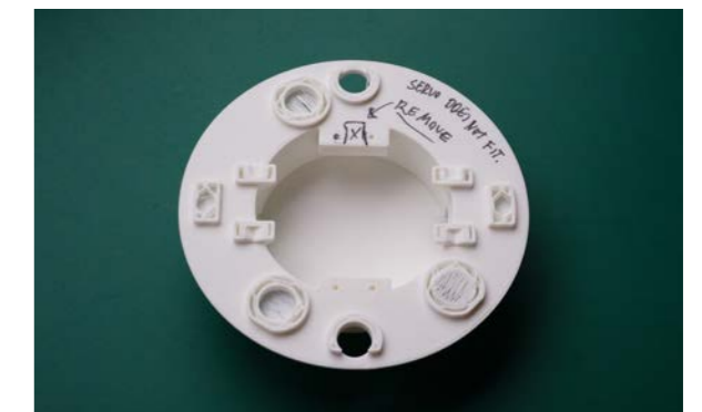
V4. Adding magnets (failed print), servo did not fit
