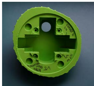
V10. Print orientation & small fitting optimisations
