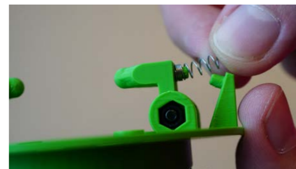
Attach the spring as shown between the latch and top circle
