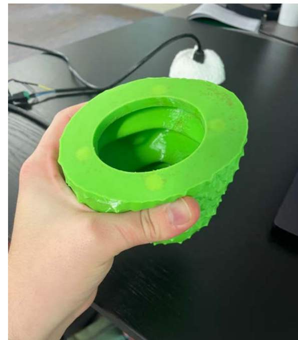
85A with 3 perimeters squished. This prototype feels softer compared to 95A – it is placed relatively in the middle of both options.
