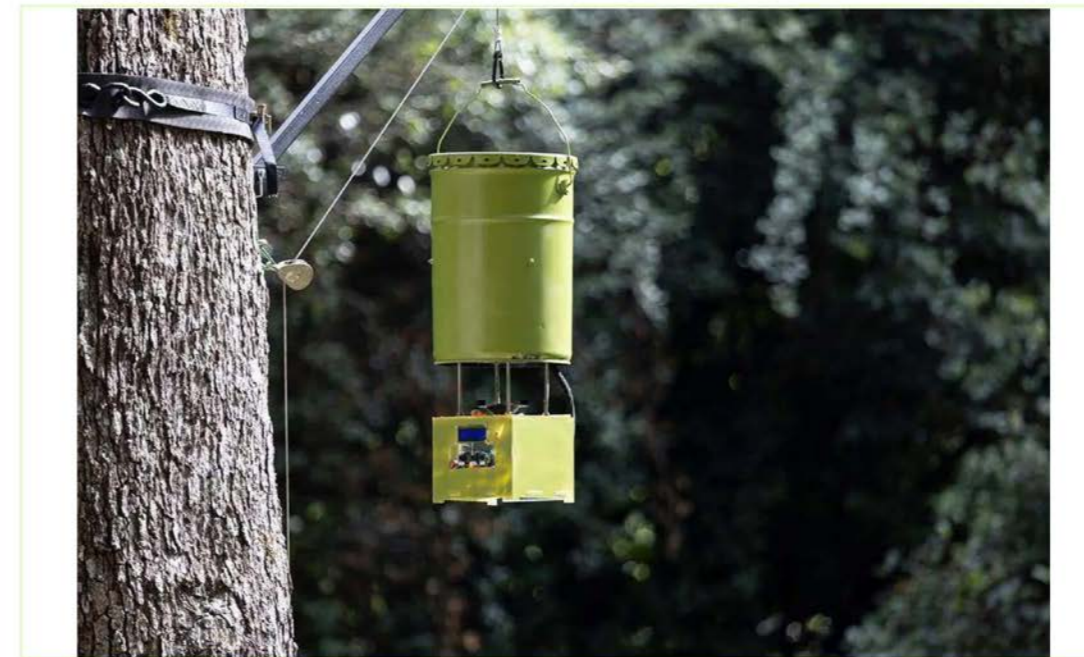
image / figure 2 An automatic food scattering device for Gorillas by Georgia Tech students which slings fruits everywhere
