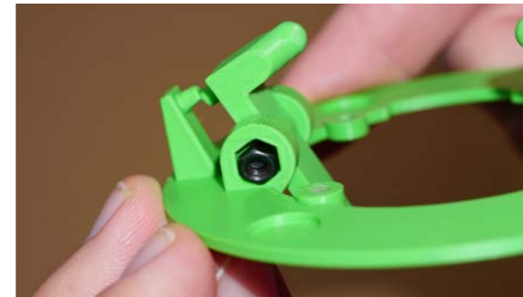
Attach a M3 nut to the other side
