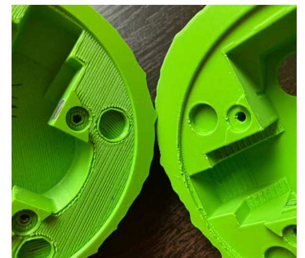
Figure Q7. Differences printing flat with supports (left) or 45 degrees angled with tree supports
