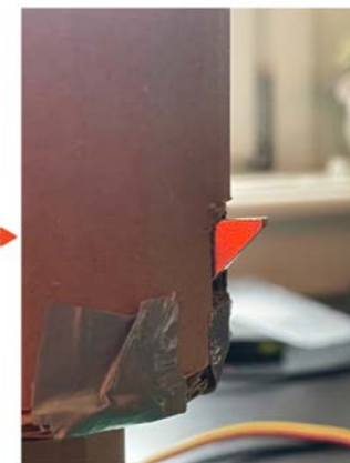
The latch sticking out holds the bottom
