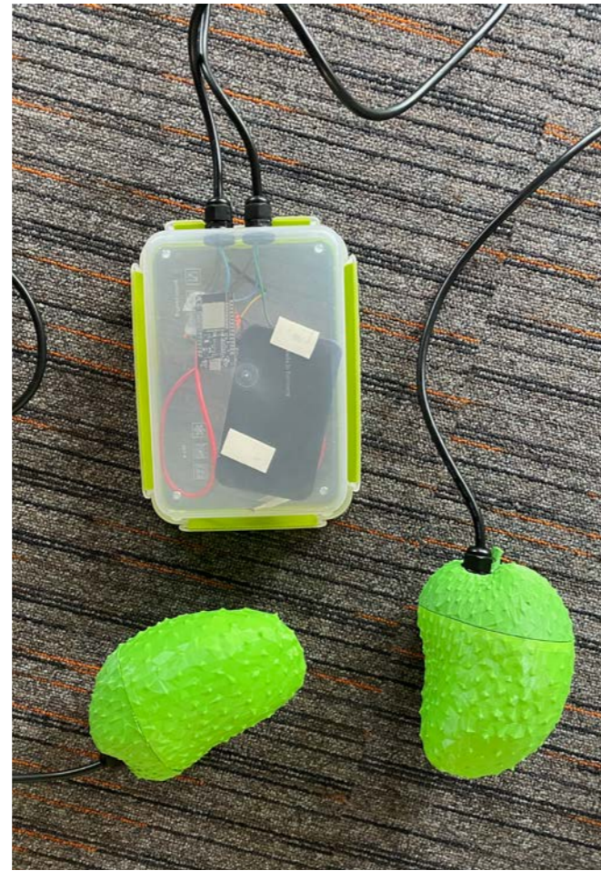
Figure 72 - Two soursop prototypes connected to an esp32 and power bank
