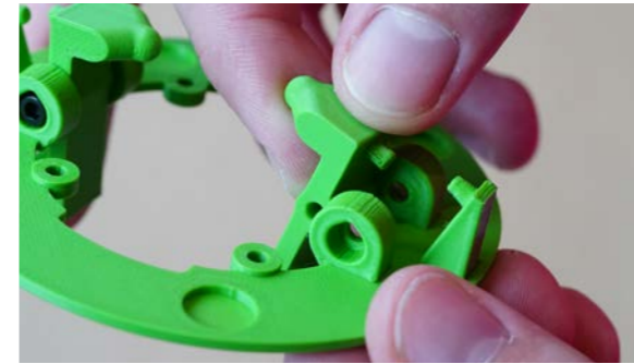
Insert the latch on the top circle
