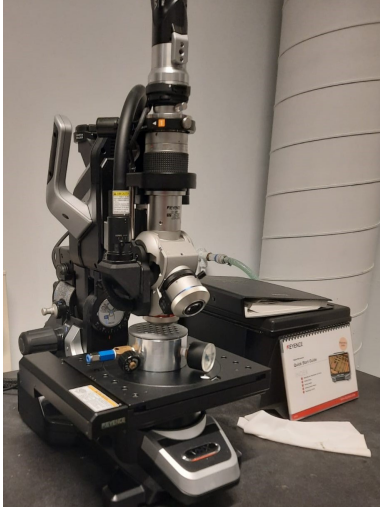
Figure 6.1: Experiment 1: Setup to visually determine the deformation. The microscope used is a Keyence VHX-6000 [59].
