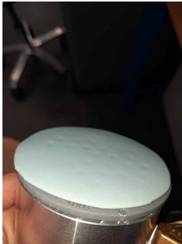
Figure H.7: Image representation of the discrepancies in the sealing performance of the suction cups. Applied pre-load » 50 N.
