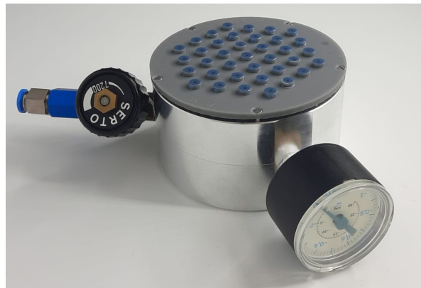
Figure 5.2: Final production sample of the end-effector.
