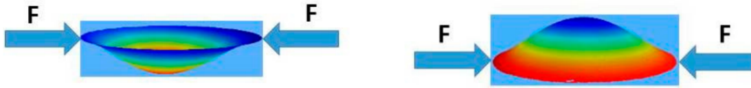
Figure 3.5: Actuation of a bi-stable membrane to its two states. The edges of the membranes are mounted and thus apply a reaction force unto the membrane [31]. (a) Membrane state during laminate release. (b) Membrane state during laminate pick-up.
