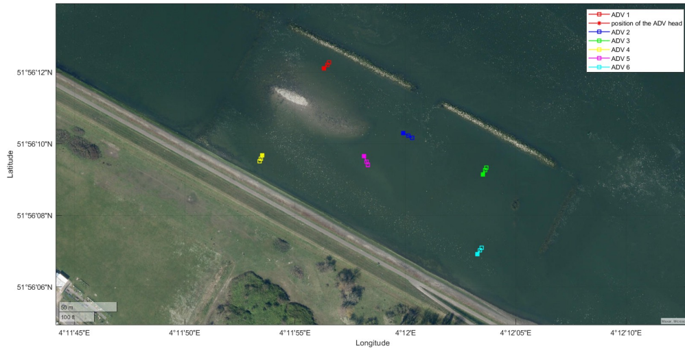
Figure 3.6: Final placement of the ADVs and the direction of the head.
