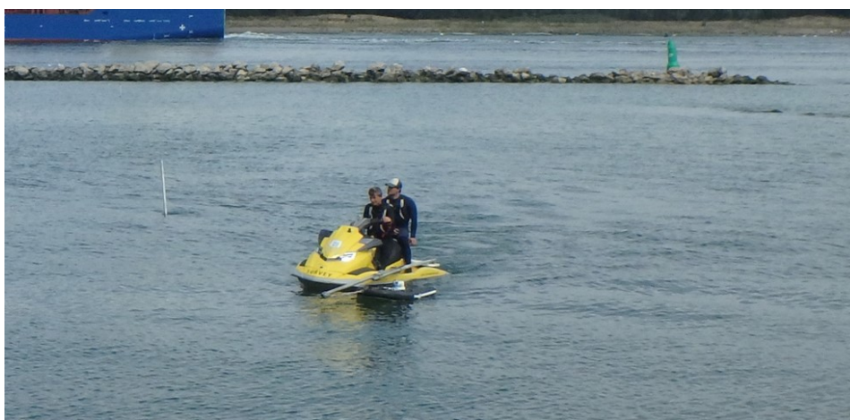
Figure 3.11: Jet ski with the attached ADCP and floating board.
