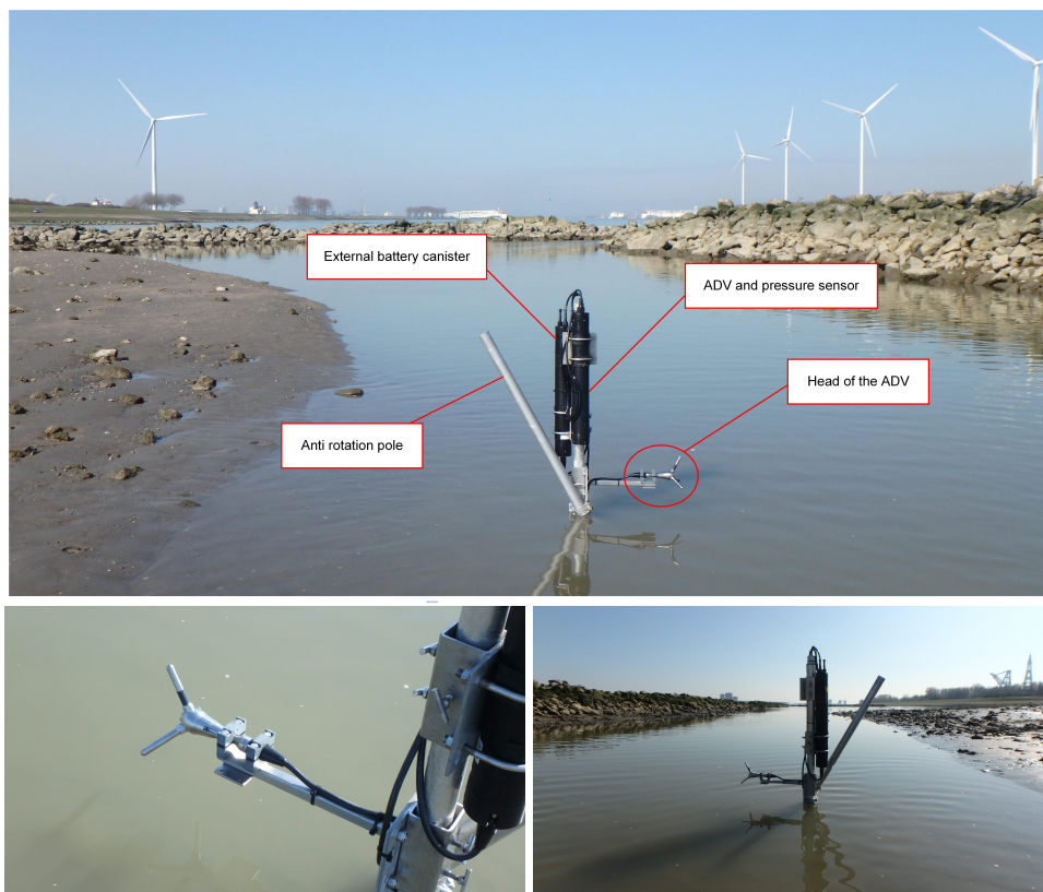
Figure 3.7: Setup of the ADV 1. The setup is made of scaffolding tubes and connector claps.
