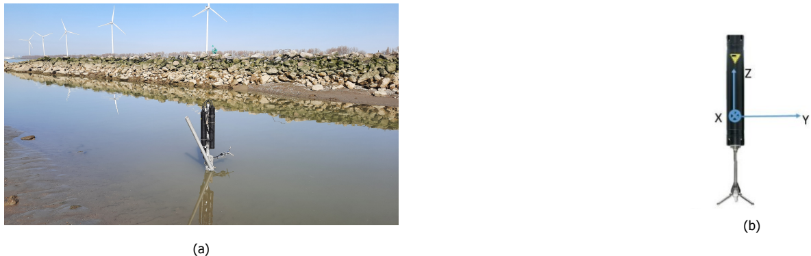
Figure 3.3: Photo of an ADV in the groyne area. (a) ADV with with battery canister mounted on a pole in the groyne area. (b) Coordinate system used by the ADV ( The Comprehensive Manual for Velocimeters , 2019).
