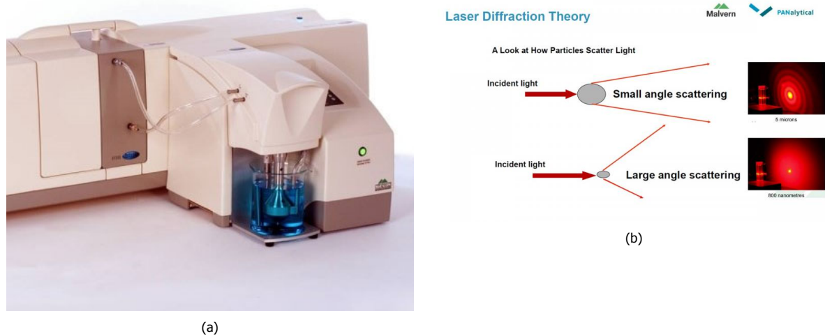
Figure 3.14: (a) The Malvern Mastersizer 2000 setup used for the experiment. (b) The principle of the method used to identify the different particle sizes ( Mastersizer 2000 User Manual, 2007 ).
