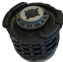
FIGURE 1.2: A rubber vibration isolator removed from the assembly.
