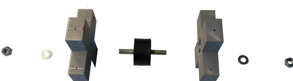
FIGURE 4.1: Exploded view from the assembled **AIB** system with from left to right: nut-washer-transmission simulator-ruber isolator-transmission simulator-washer-nut.
