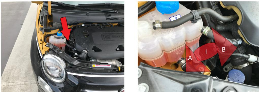
FIGURE 1.1: Location of rubber vibration damper in the vehicle. On the right: A is the chassis frame, B the engine subframe and I the isolator.
