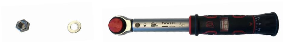
FIGURE 4.3: Materials to fasten transmission simulator to the vibration isolator. From left to right: Nut, washer and calibrated torque wrench.
