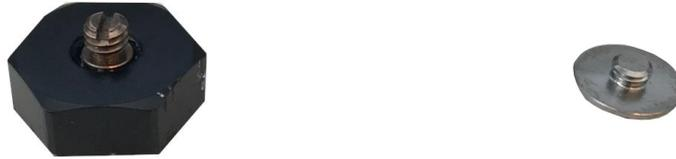
FIGURE 4.21: Left: A sensor mount of type 1. Right: A sensor mount of type 2, used in the measurement campaigns for this thesis
