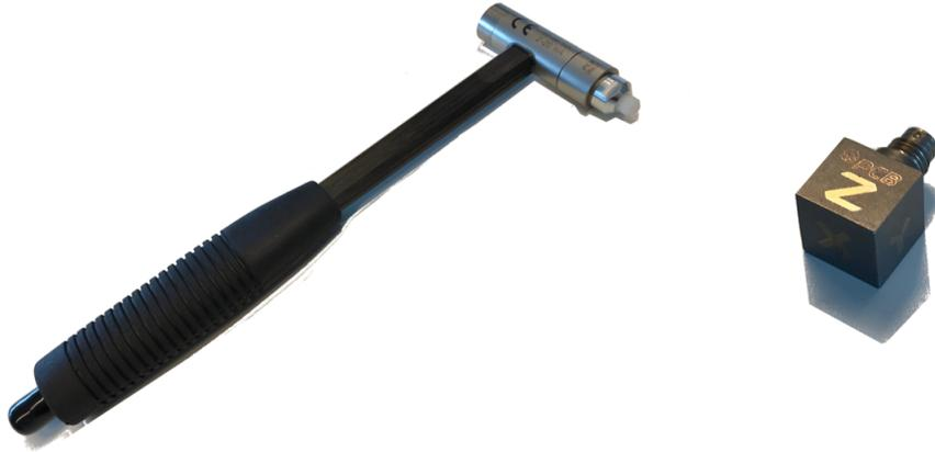
FIGURE 2.3: Left: an impact hammer with a load cell on the tip. Right: An accelerometer suited for adhering to a test structure.
