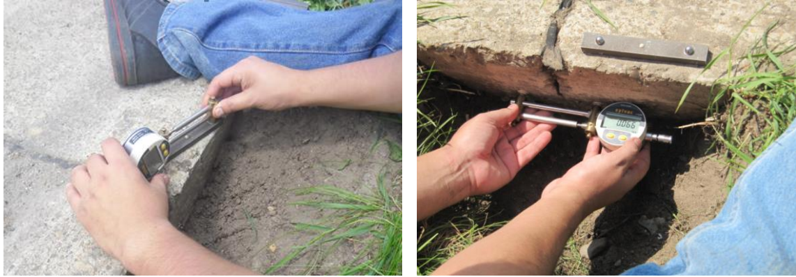
Fig. 5.3.2. Measurements with LVDT and invar bar.
