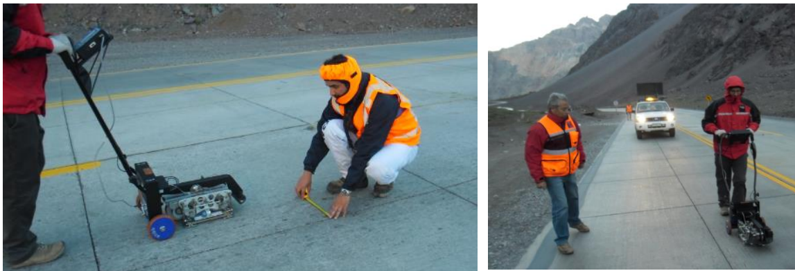
Fig.7.6.1. Measurements performed with the WP. Checking the track position (left) and measurements with safety assistance (right)
