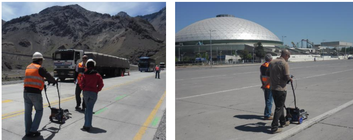
Fig. 7.6.2. Measurements performed with WP at Route 60 Ch (left) and Santiago city (right)
