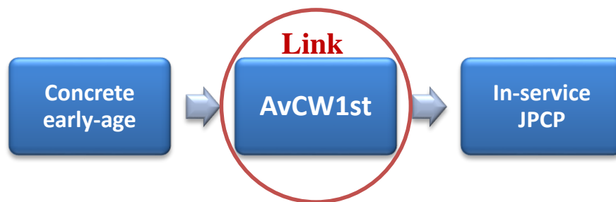
Fig. 5.4.2. Intended use of the model of the early-age concrete behavior in the present research.
