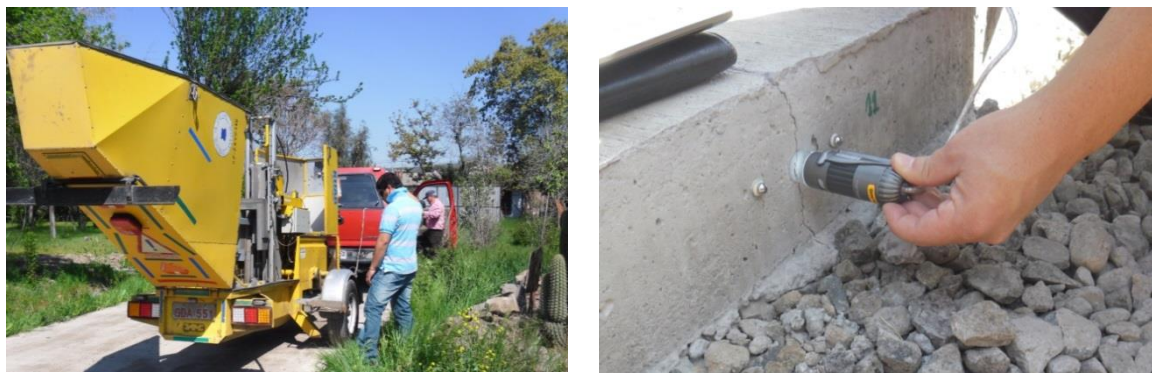
Fig. 6.4.3. Measurements of LTE with FWD (left) and crack width with microscope (right)
