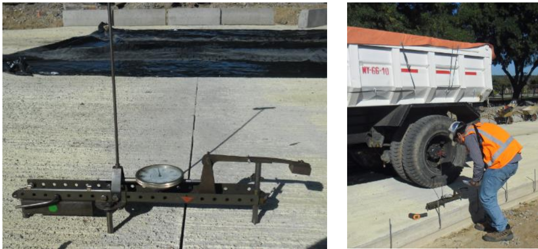
Fig 6.4.6. Faultimeter position on a joint (left) and reading of the gauge (right).
