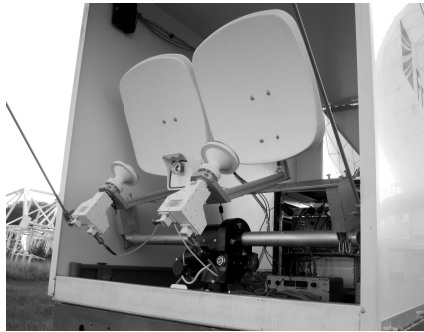
Figure 4.2: LabRaDor radar system of Fraunhofer FHR used during the experimental measurement campaign.
