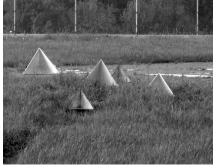
Figure 4.1: Five corner reflectors used during the experimental measurement campaign.
