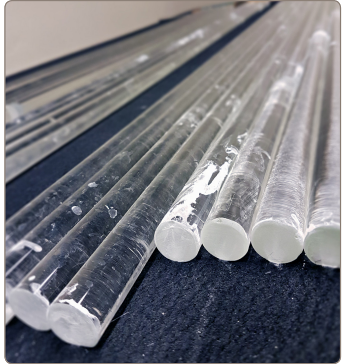
Figure 45: Rods cut and sanded
