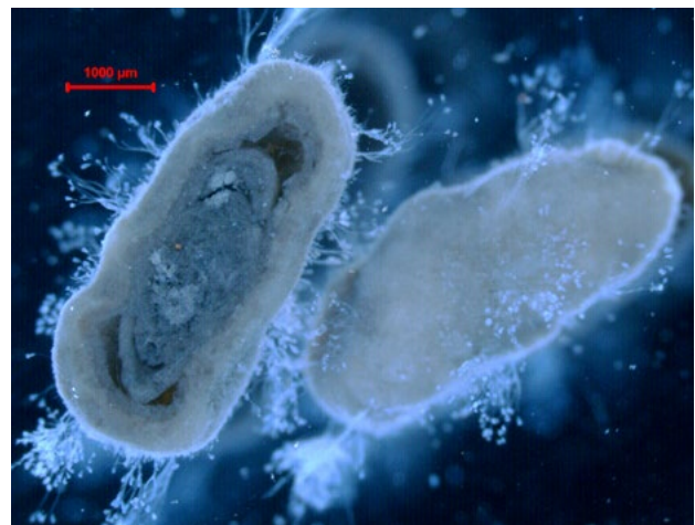
Fig. 10 Microscopic pictures of sieved granules ( > 2 mm) from Utrecht (top) and Garmerwolde (below). Organic material (e.g., little leaves, sand grains, twigs, seeds) was found inside that could have functioned as seeding material. Bars indicate 1000 \mu\text{m} .
