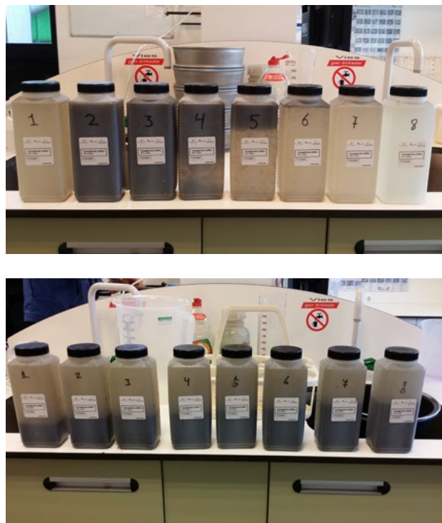
Fig. 23 Excess sludge samples during dry weather conditions (above) and rain events (below) showed differences in sludge content and sludge distribution over the bottles.
