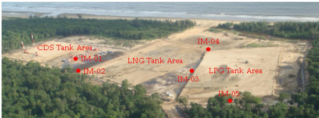
Figure 67 – Site overview during construction inclusive the location of the inclinometers
