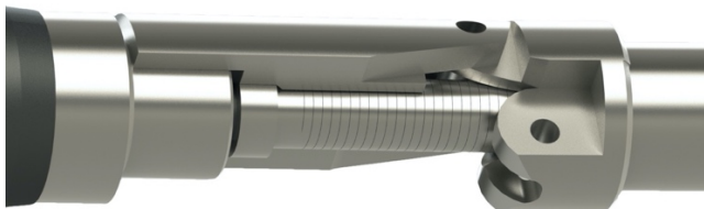
Figure 24, Stainless steel overtube. A cross section of the SATA tip base component containing an overtube of 2 mm in diameter and a length of ~10 mm. The component is not fixed but held in place by the screw component of the tip (SS base), the SATA tip base and both sliders. This ensures that the modularity is retained and cleaning is accessible. Furthermore, the component can easily be replaced when necessary.
