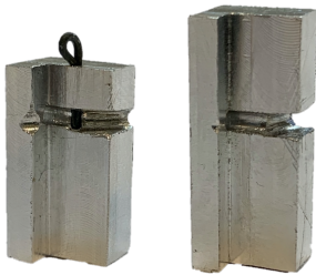
Figure 18, Aluminium 'angle blocks'. Left: 45 degrees angle at slider High side with hinge axis pin. Right: 70 degrees angle at slider low and H hinge side. There is no interference of the hinge pin while steering in this direction.
