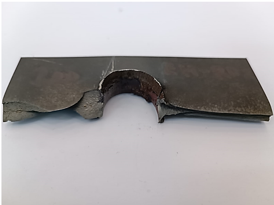
Figure 2.9: Close up of perforation cross section post fracture, courtesy of TNO
