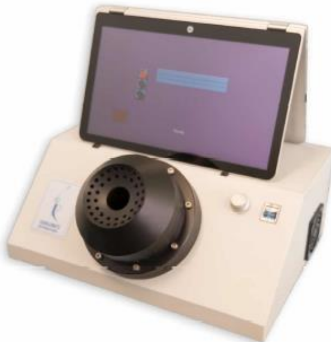
image / figure 2 Self-Administered Computerized Olfactory Testing System (SCOTS) (Sensonics International [2], 2024)
