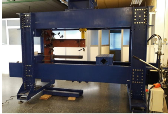
Fig. 7 Assembly of the beams to be carried out the tests in the laboratory press
