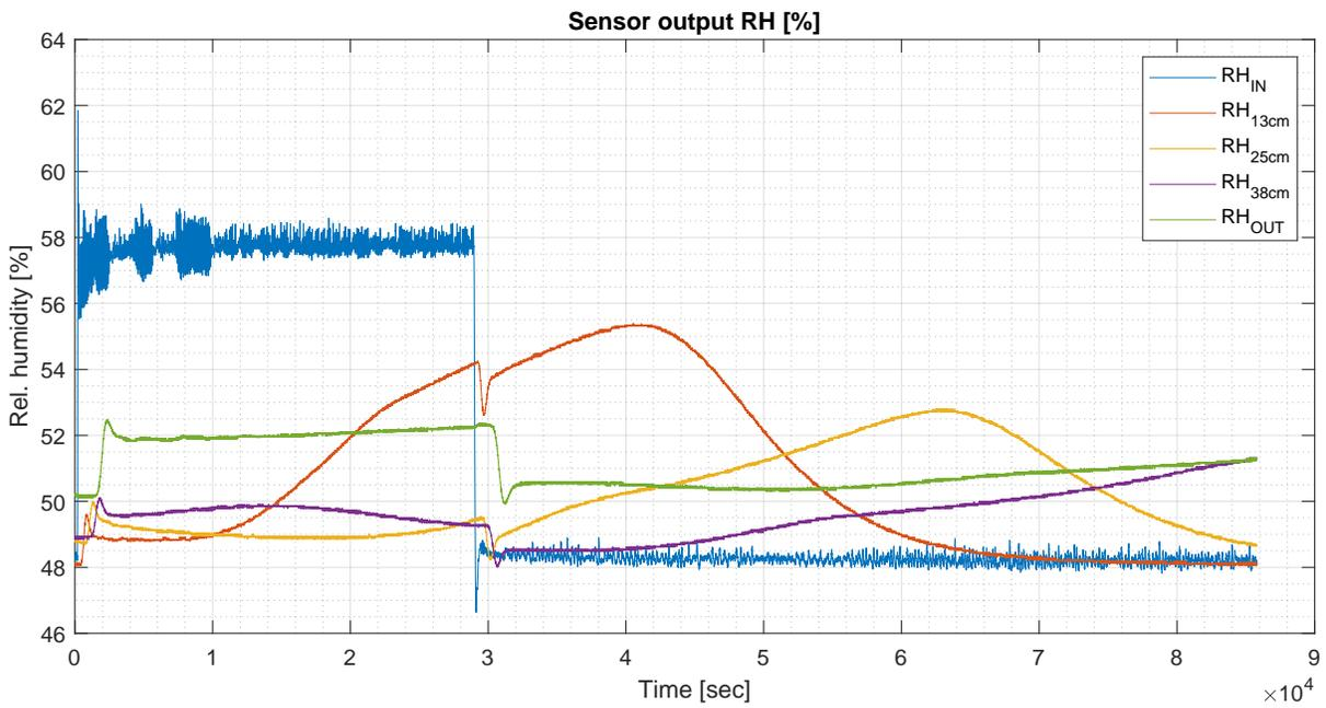
Figure 3.21: Relative humidity measurements in Run 5, cycle 2.
