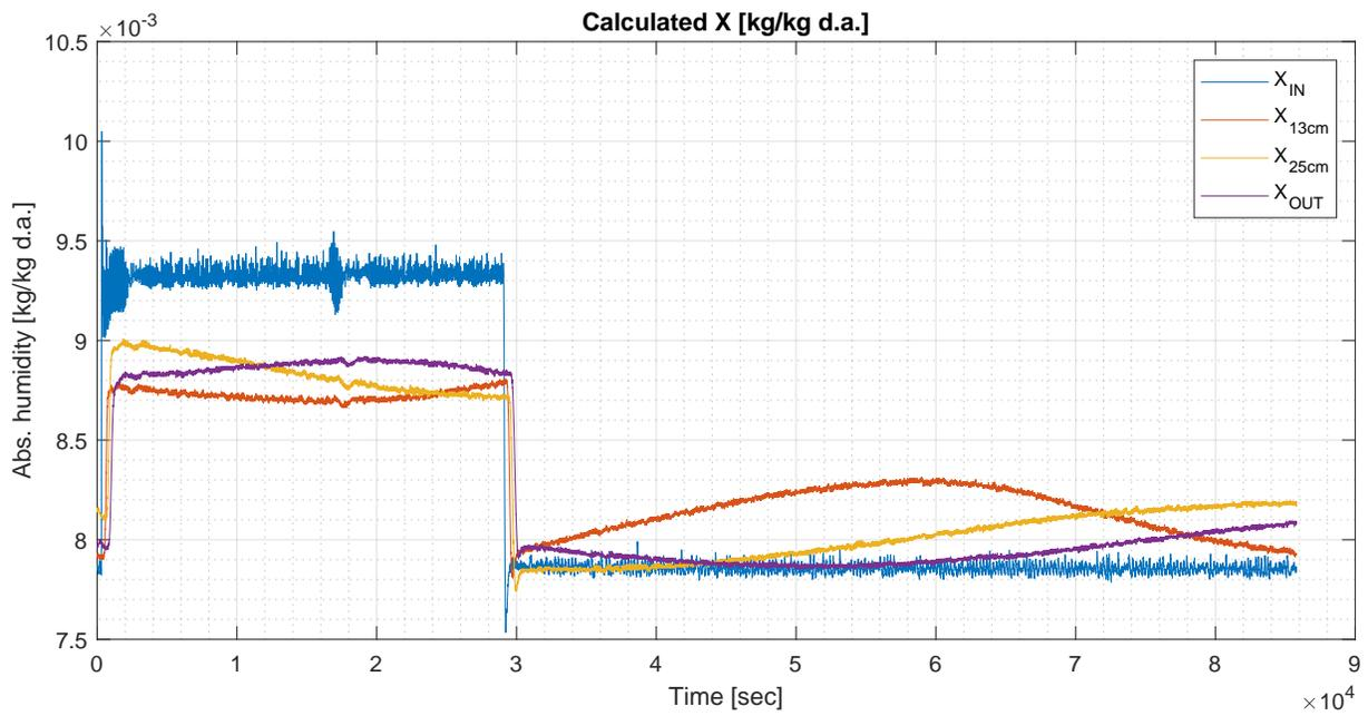
Figure 3.34: Absolute humidity calculated from RH and T in Run 6, cycle 2.
