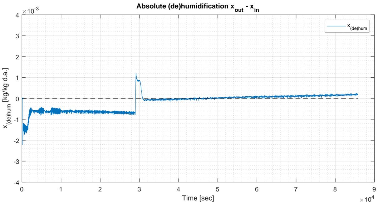
Figure 4.6: Absolute (de)-humidification of air in Run 5, cycle 2.
