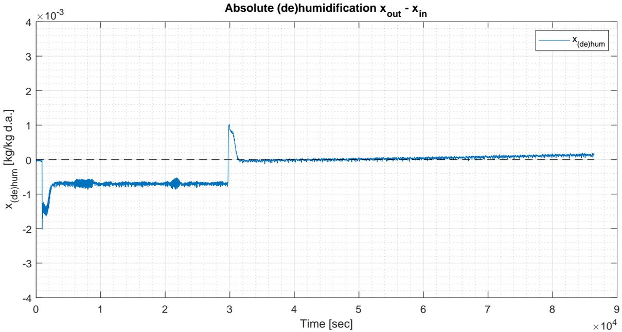
Figure 4.14: Absolute (de)-humidification of air in Run 8, cycle 1.
