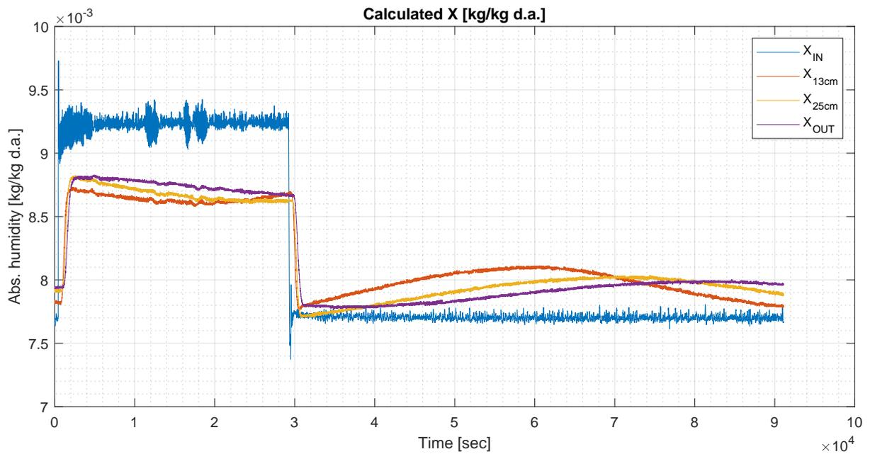
Figure 3.62: Absolute humidity calculated from RH and T in Run 8, cycle 3.
