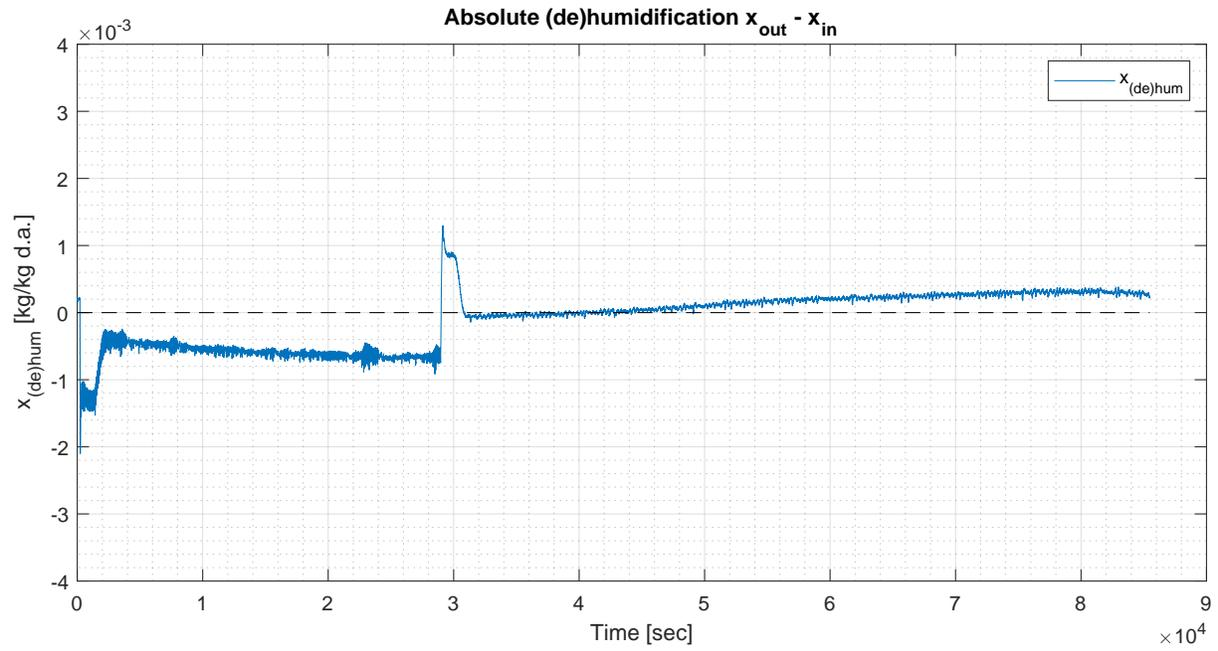
Figure 4.7: Absolute (de)-humidification of air in Run 5, cycle 3.
