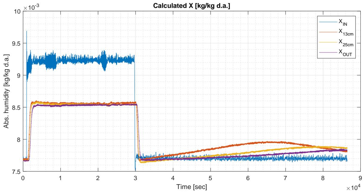
Figure 3.54: Absolute humidity calculated from RH and T in Run 8, cycle 1.
