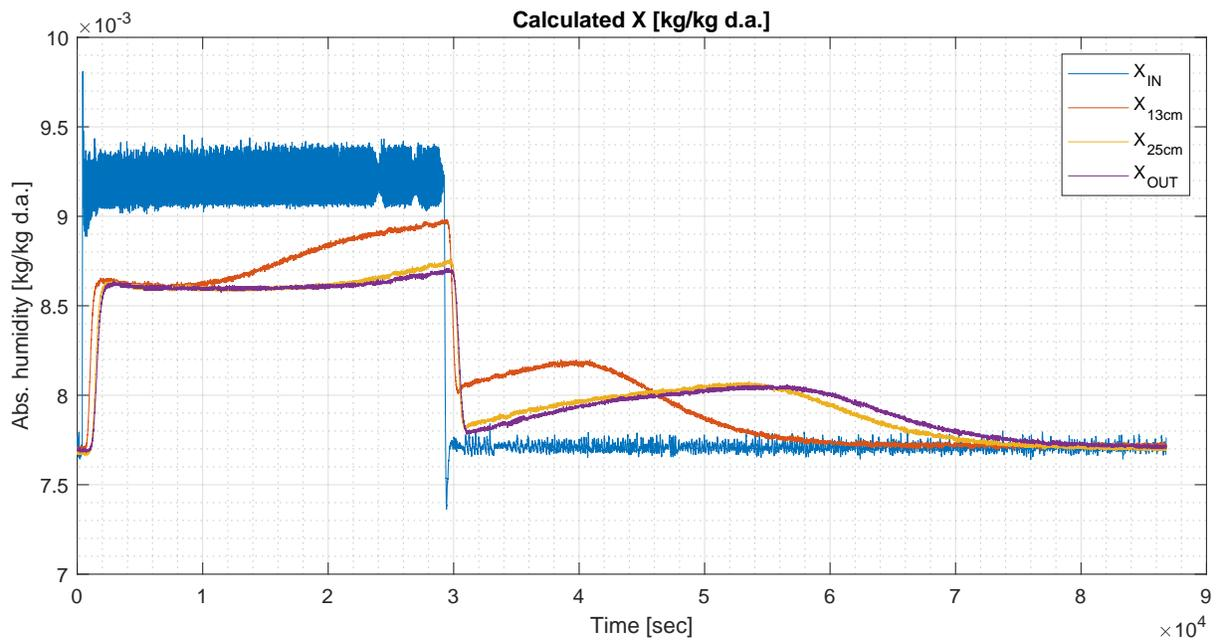
Figure 3.42: Absolute humidity calculated from RH and T in Run 7, cycle 1.
