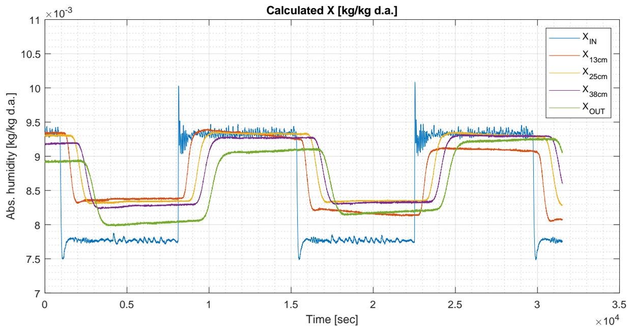
Figure 2.6: Absolute humidity calculated from RH and T in Run B.
