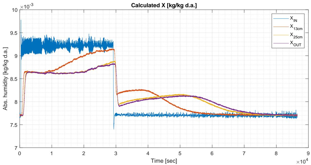
Figure 3.46: Absolute humidity calculated from RH and T in Run 7, cycle 2.
