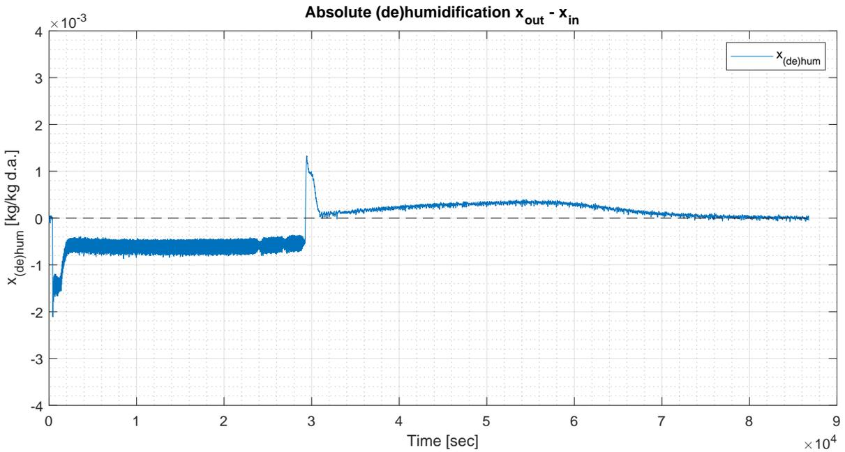
Figure 4.11: Absolute (de)-humidification of air in Run 7, cycle 1.
