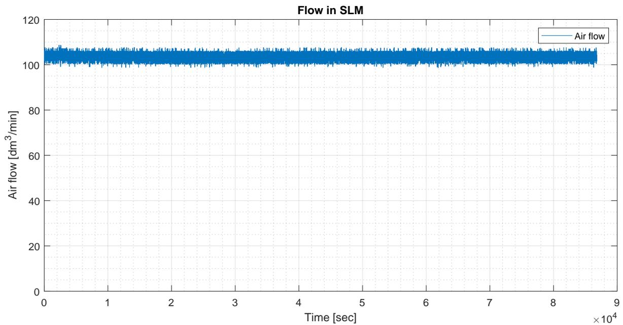
Figure 3.44: Flow measurements from RH and T in Run 7, cycle 1.
