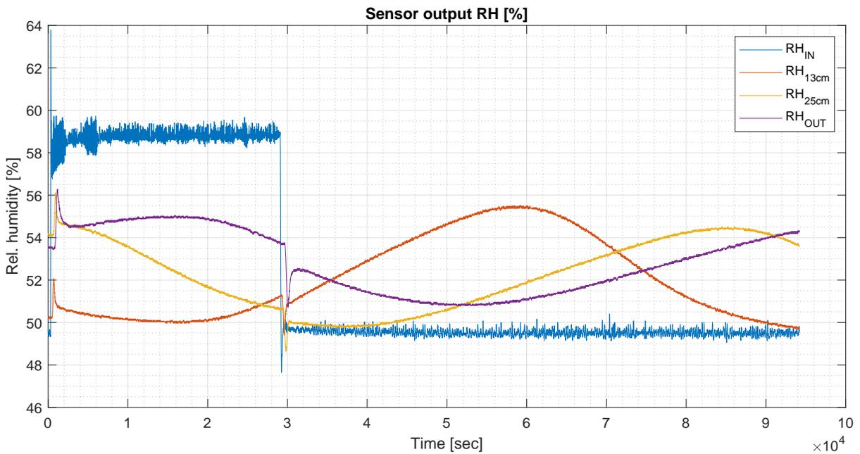
Figure 3.37: Relative humidity measurements in Run 6, cycle 3.
