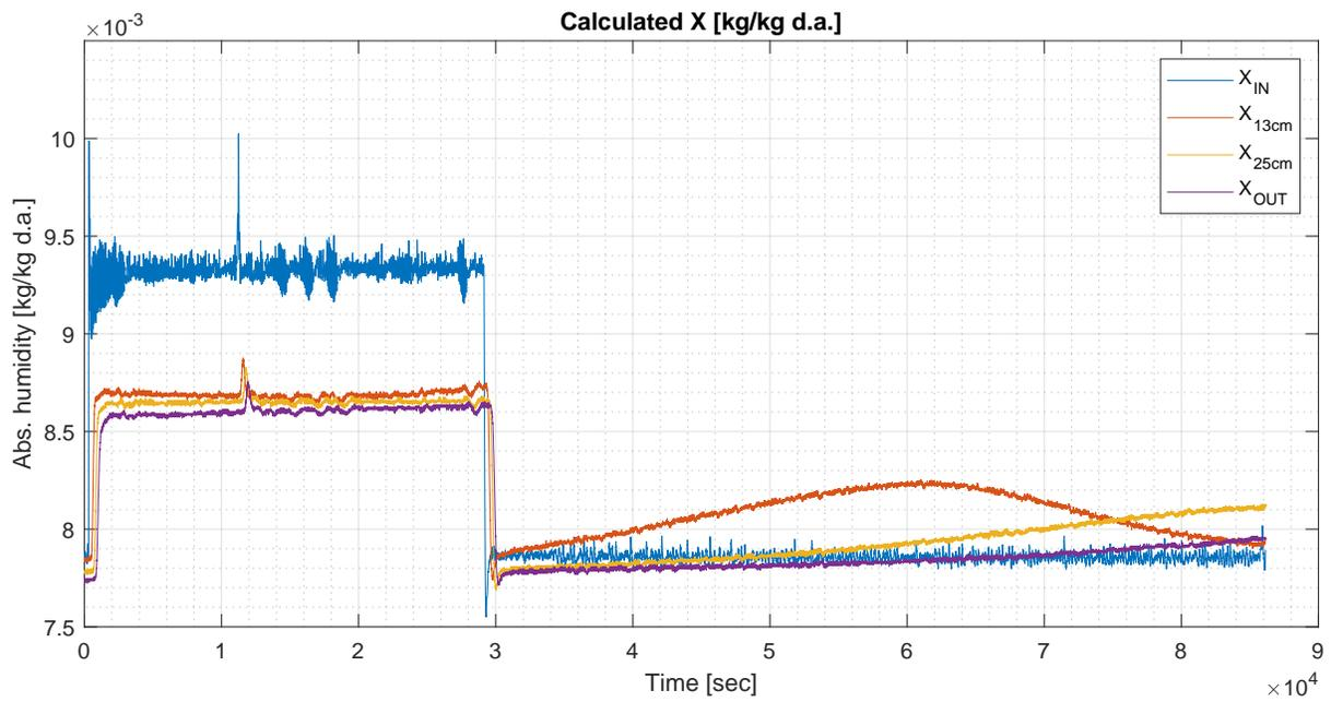
Figure 3.30: Absolute humidity calculated from RH and T in Run 6, cycle 1.
