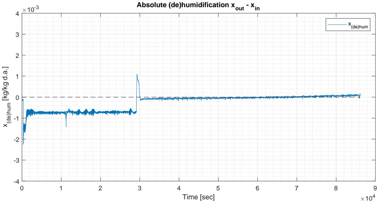
Figure 4.8: Absolute (de)-humidification of air in Run 6, cycle 1.
