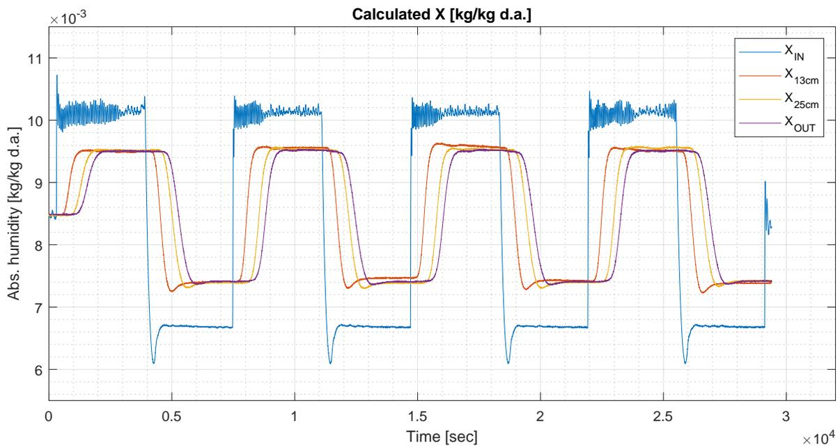
Figure 3.10: Absolute humidity calculated from RH and T in Run 3.
