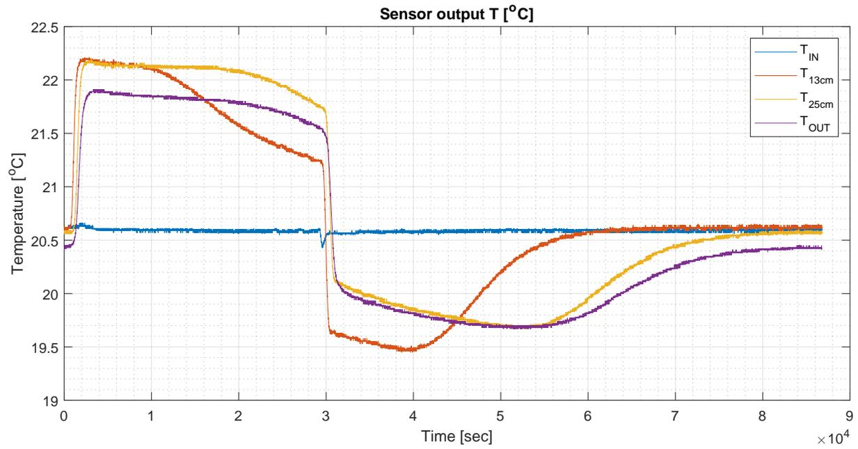
Figure 3.43: Temperature measurements in Run 7, cycle 1.
