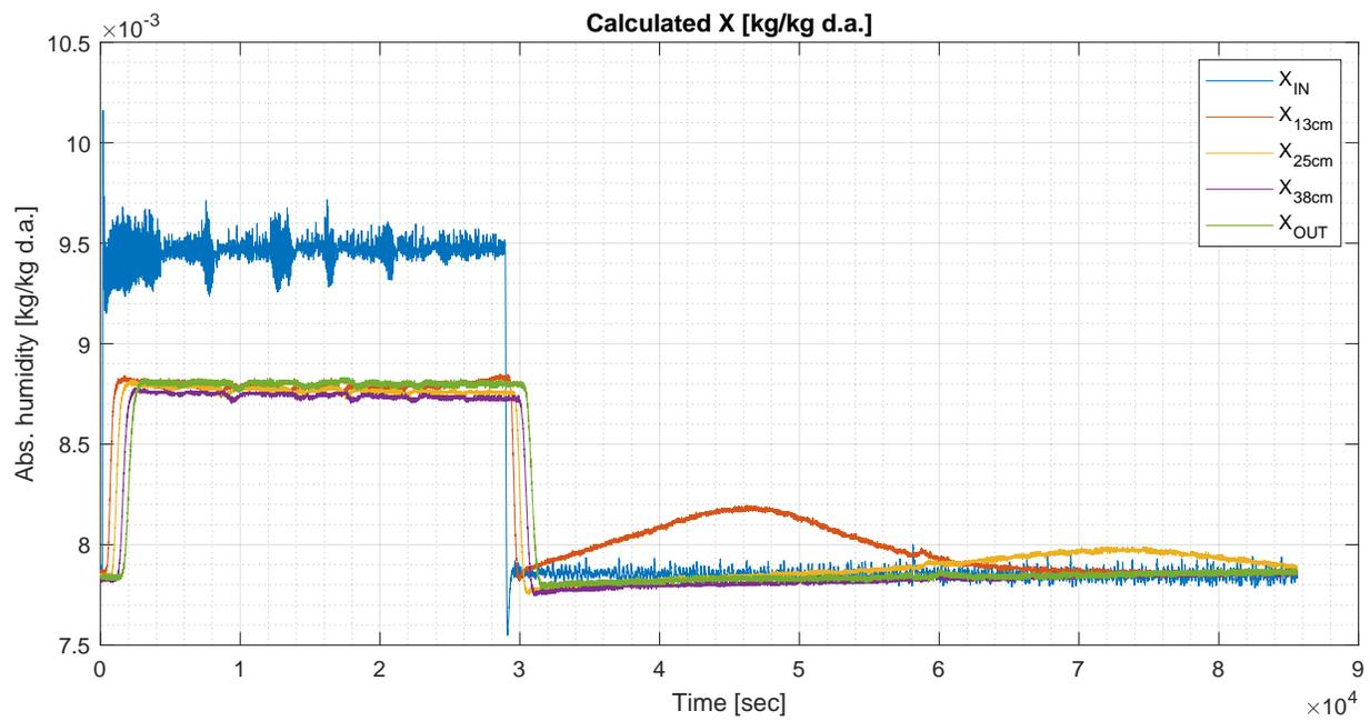
Figure 3.18: Absolute humidity calculated from RH and T in Run 5, cycle 1.
