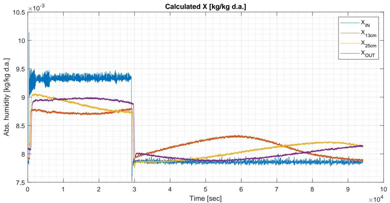
Figure 3.38: Absolute humidity calculated from RH and T in Run 6, cycle 3.
