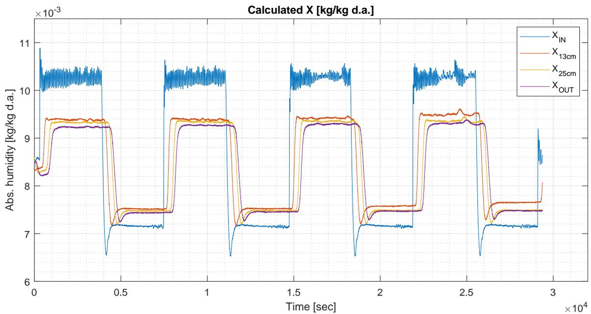
Figure 2.14: Absolute humidity calculated from RH and T in Run D.
