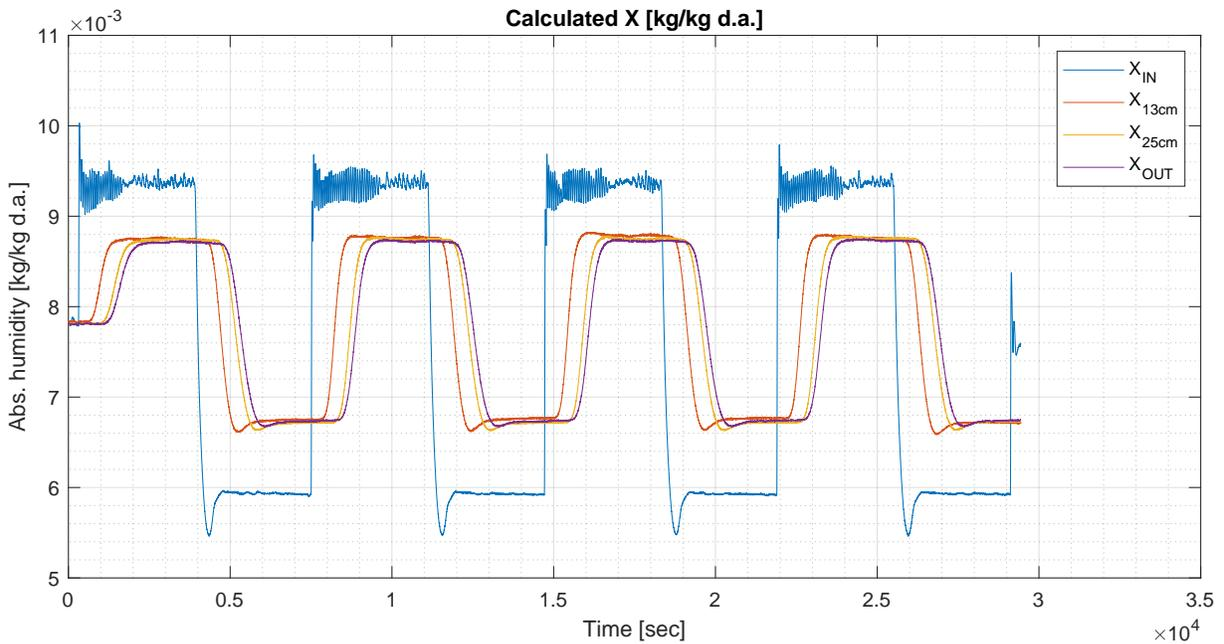
Figure 3.2: Absolute humidity calculated from RH and T in Run 1.
