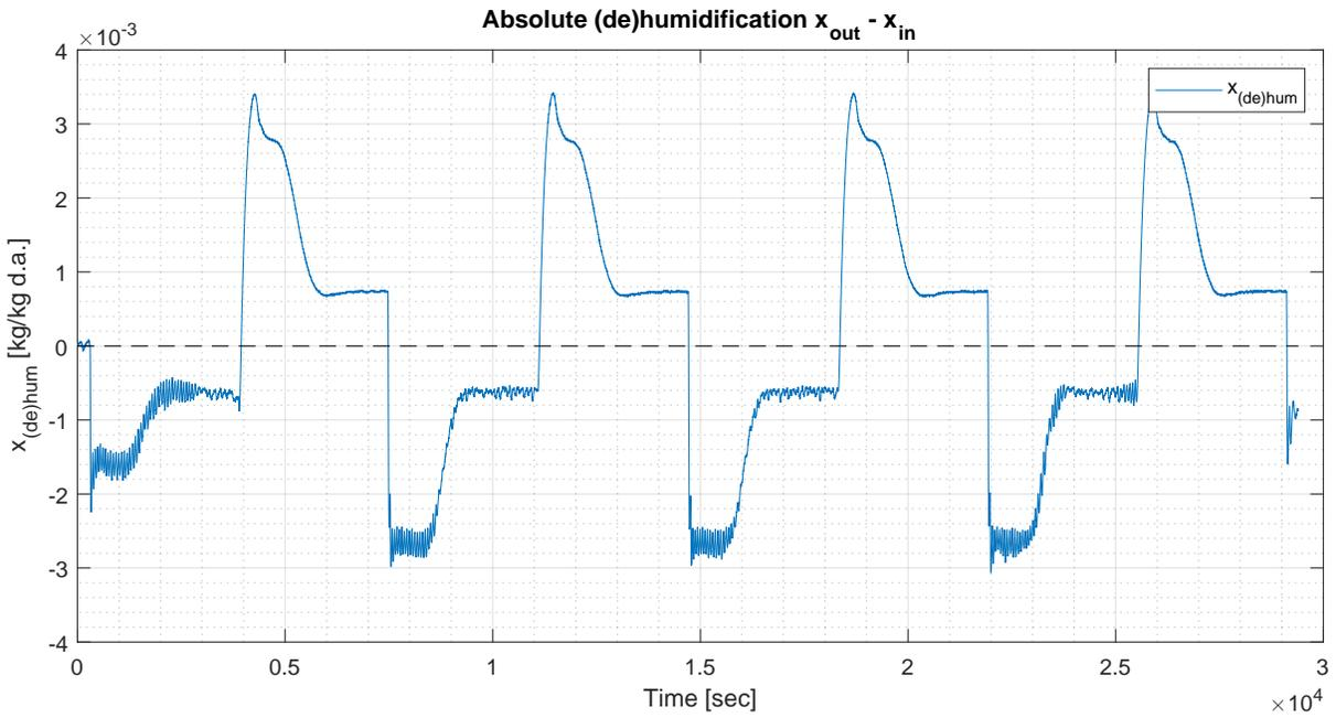
Figure 4.3: Absolute (de)-humidification of air in Run 3.
