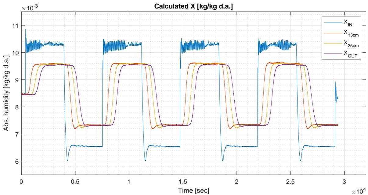
Figure 3.14: Absolute humidity calculated from RH and T in Run 4.
