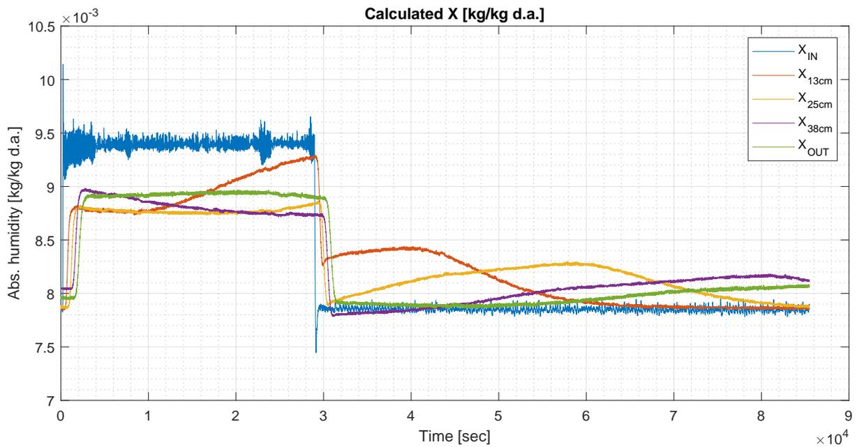
Figure 3.26: Absolute humidity calculated from RH and T in Run 5, cycle 3.
