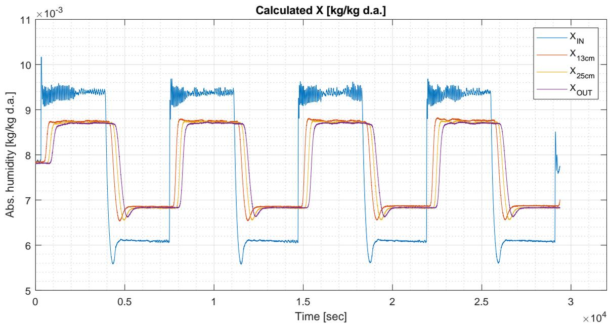
Figure 3.6: Absolute humidity calculated from RH and T in Run 2.
