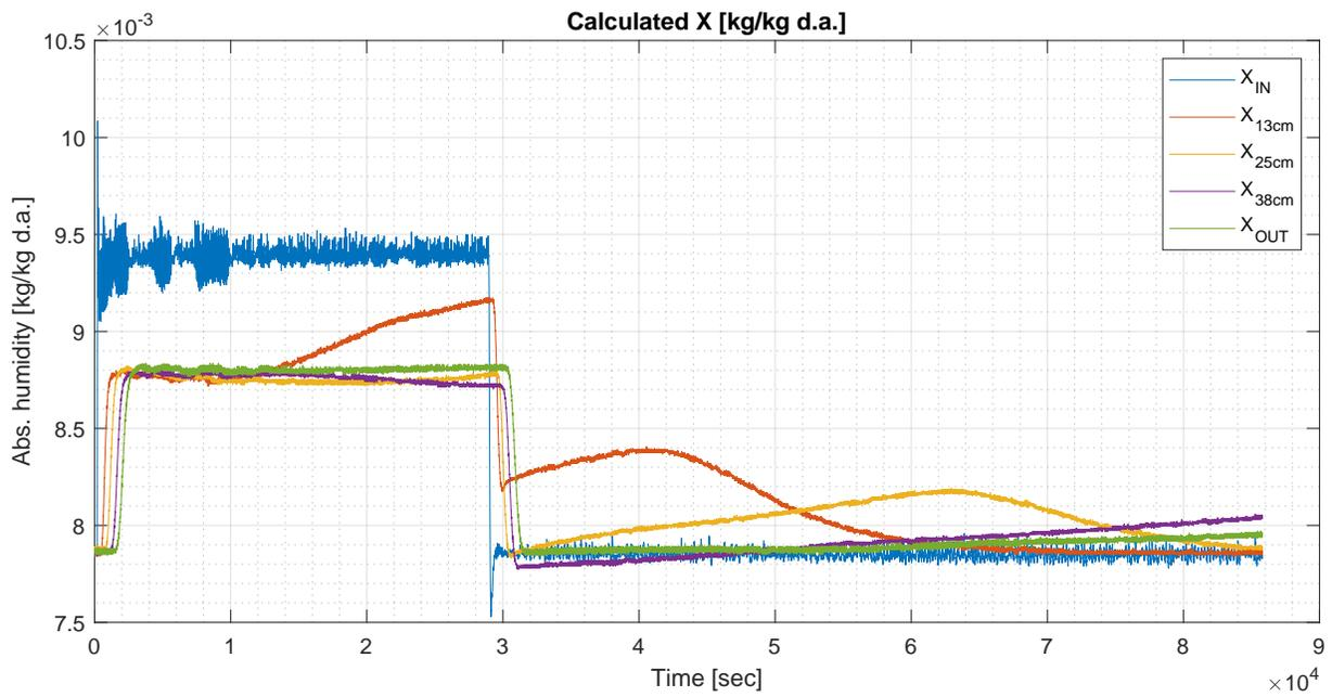
Figure 3.22: Absolute humidity calculated from RH and T in Run 5, cycle 2.
