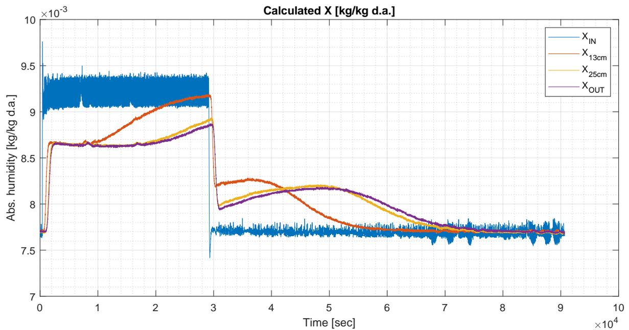
Figure 3.50: Absolute humidity calculated from RH and T in Run 7, cycle 3.
