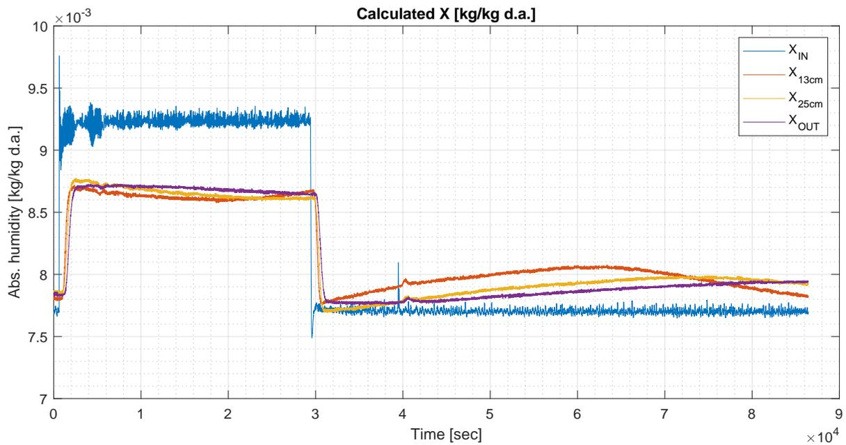
Figure 3.58: Absolute humidity calculated from RH and T in Run 8, cycle 2.
