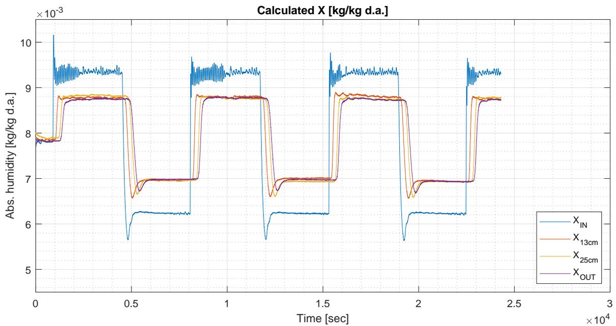
Figure 2.10: Absolute humidity calculated from RH and T in Run C.
