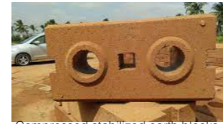
Compressed stabilized earth blocks
