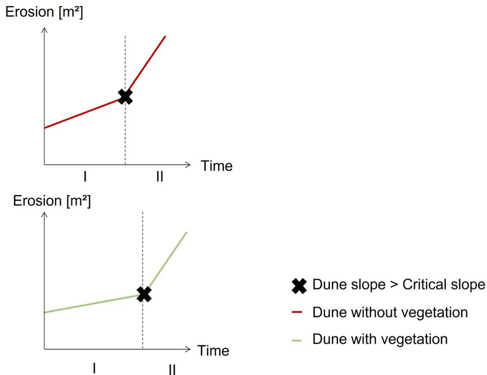
Figure 2.11: Concept of collision regime over time in relation to erosion volume- and dune vegetation
