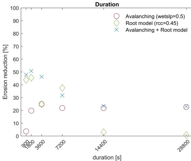
**Figure 7.5:** Reduction erosion volumes for dunes with the application of a higher critical angle in the avalanching module and the root model for dunes exposed to a different storm duration. A longer duration results in all cases in more erosion (not illustrated in this figure). Until a certain point, the impact of the avalanching module increases with rising wave height. Root model impact decreases with increasing wave height. Both approaches together reinforce each other.
