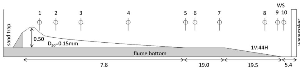
Figure D.1: Set-up wave flume experiment Bryant. Not to scale (source: Bryant et al. [2019])
