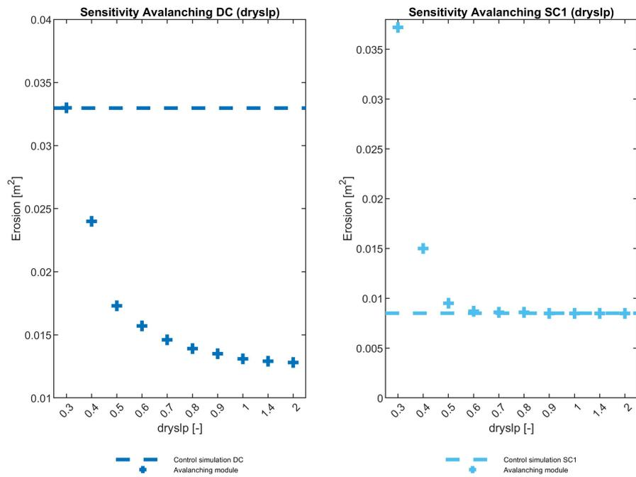
Figure 4.21: Sensitivity critical dry slope in the avalanching module for Bryant DC (left) and SC1 (right) case. The sensitivity pattern is similar. A higher *dryslp* results in a smaller absolute erosion volume. Note: the y axes are different
