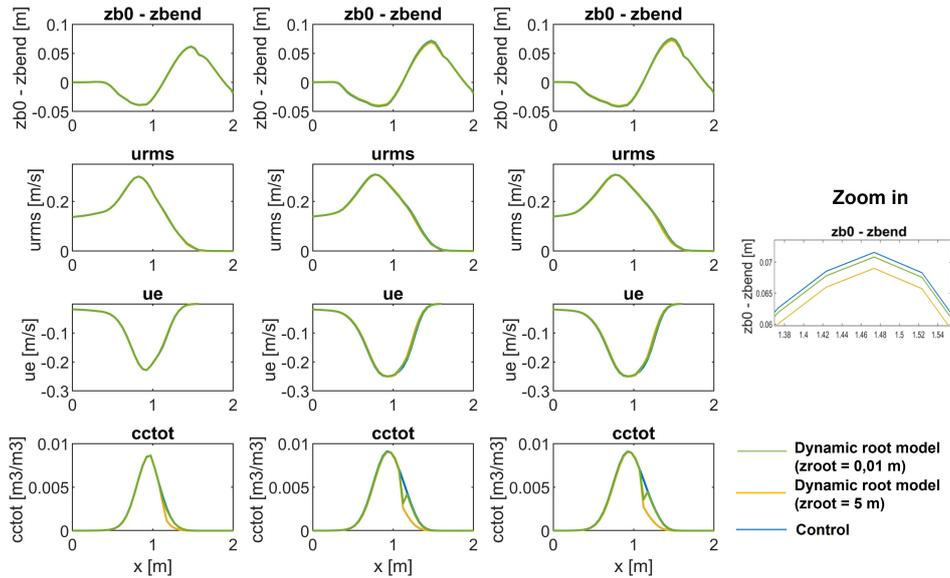
**Figure 4.15:** Dynamic root model takes into account deposition and erosion of the dune. The erosion of the dune in the dynamic root model. When erosion depth = rooting depth ( $zroot$ ), the effect of the root model decreases (yellow line).
