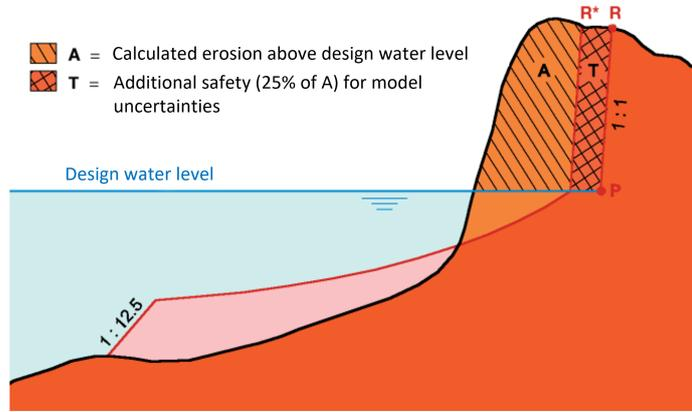
Figure 2.6: Calculation storm erosion profile (source: ENW [2007])
