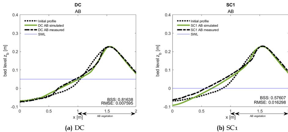
Figure 4.7: Profiles of Bryant DC (left) and SC1 (right) simulation with above and belowground vegetation
