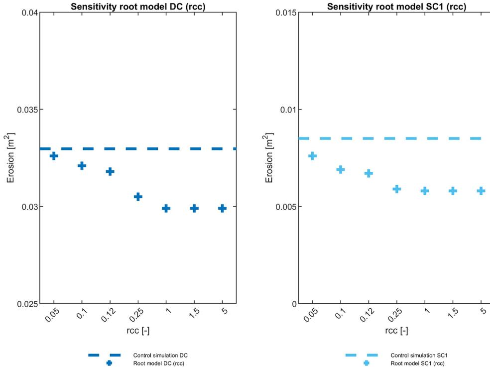
Figure 4.12: Sensitivity root cohesion coefficient (*rcc*) parameter constant root model for Bryant DC and SC1 case. A higher *rcc* results in a reduction in erosion volume to a certain extent. Note: the y axes are different
