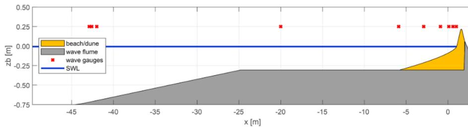
Figure 3.8: XBeach model set-up Bryant experiments. Data for profile evolution is available for  $0 < x < 2$  m. Source: Schweiger and Schuettrumpf [2021a]
