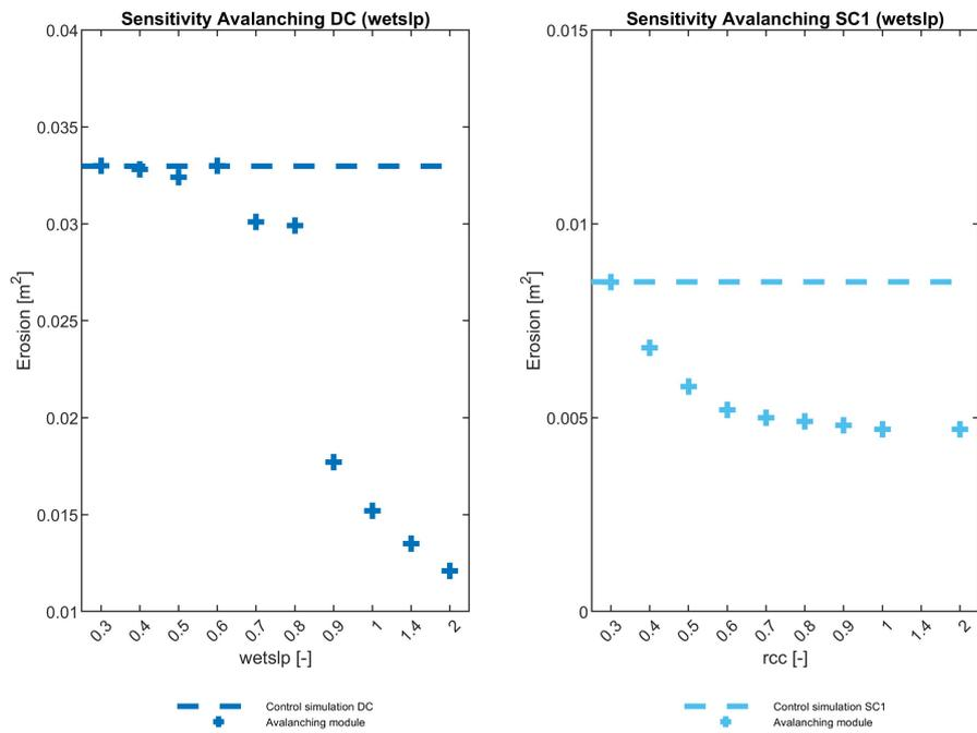
Figure 4.18: Sensitivity critical wet slope in the avalanching module for Bryant DC (left) and SC1 (right) case. A higher *wetslp* results in lower absolute erosion volumes. For the DC case, a jump can be observed between a *wetslp* of 0.9 and 1. A higher *wetslp* in the SC1 case results in a gradual erosion reduction. Note: the y-axes are different.
