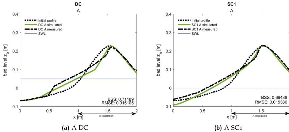
Figure 4.5: Profiles of Bryant DC (left) and SC1 (right) simulation with aboveground vegetation
