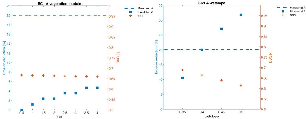
Figure G.2: SC1 A relation reduction in erosion, BSS and value of Cd for the vegetation module/value of wetslope of the avalanching module. A higher Cd and wetslope result in more erosion reduction and a lower BSS
