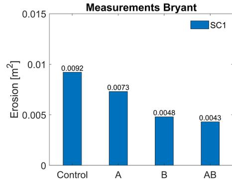
Figure D.4: Eroded volume SC1 Bryant measurements
