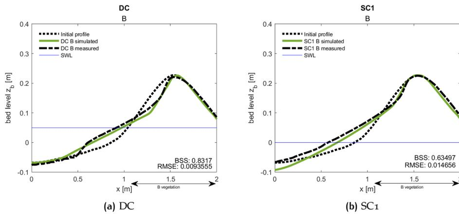
Figure 4.6: Profiles of Bryant DC (left) and SC1 (right) simulation with belowground vegetation
