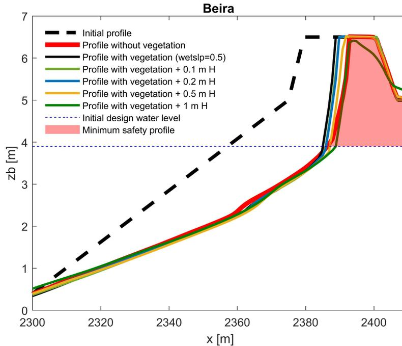
Figure 7.7: Effect of higher wave heights on erosion volumes for a dune with vegetation. Applying a higher critical angle representing vegetation could withstand storms with wave heights of 0.5 - 0.8 meters higher than is accounted for now.
