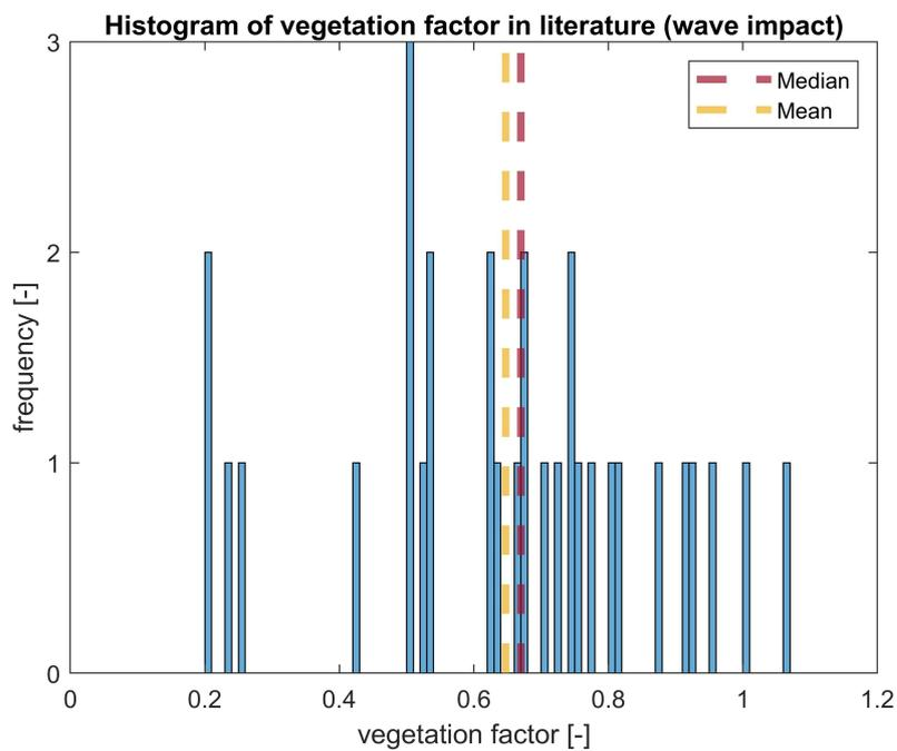
Figure 2.14: Histogram of calculated vegetation factors (wave impact). Frequency is the number of studies with the corresponding vegetation factor found in the literature.
