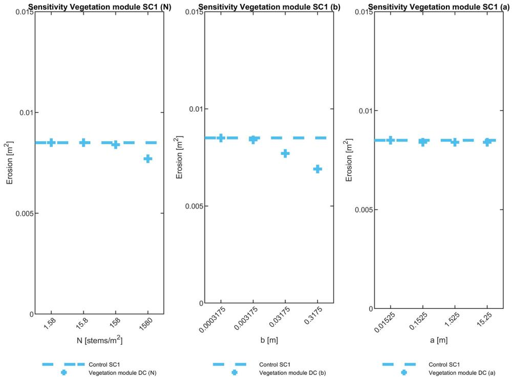
**Figure 4.10:** Sensitivity vegetation density ( $N$ ), vegetation diameter ( $b$ ) and vegetation height ( $a$ ) parameters in the vegetation module for Bryant SC1 case. A higher  $N$ ,  $b$  and  $a$  result in slightly less erosion.
