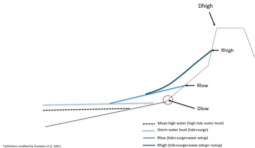
Figure 2.3: Definition sketch of parameters used to define Sallenger impact regime
