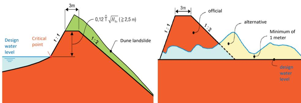
Figure 2.7: Definition of minimum standard safety profile (right) and minimum alternative safety profile (left). (source: ENW [2007])
