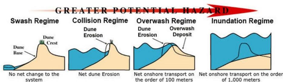
Figure 2.4: Sketch of storm impact regimes and erosion processes (source: USGS [2020])
