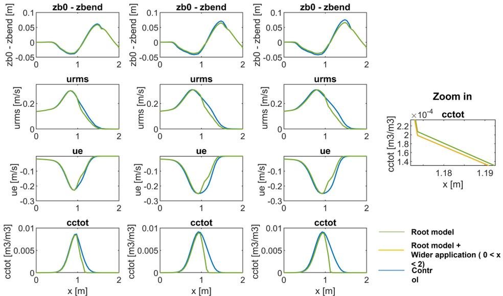
Figure 4.13: Root model impacts the sediment concentration and subsequently the velocities and bed profile. A wider application of the vegetation width demonstrates an insignificant effect (right zoom in the plot)
