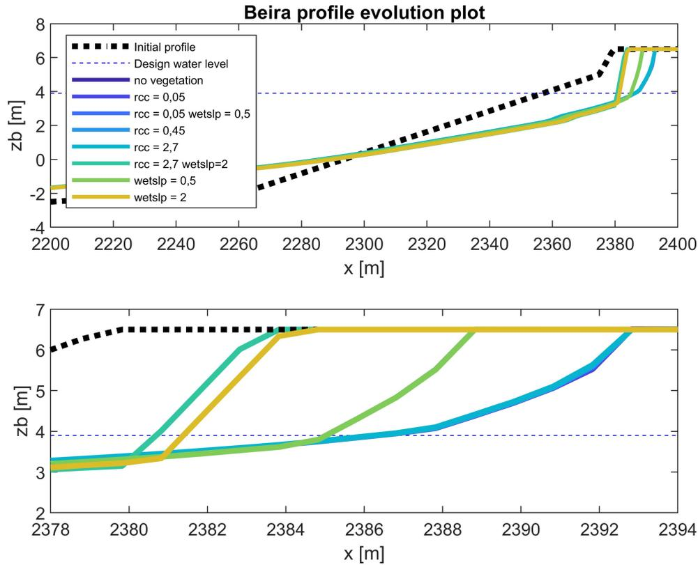
Figure 7.1: Illustration of profile evolution Beira model with the application of different vegetation approaches. Above plot shows the beach and dune and the lower plot a zoom in of the dune. The simulation without vegetation has the largest retreat and the simulation with both a higher critical angle (avalanching) and root model shows the smallest retreat and erosion volume.
