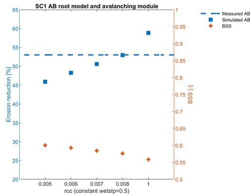
Figure G.4: SC1 relation reduction in erosion, BSS and value of rcc for the root model and a constant higher value of wetslope. A wetslope of 0.5 and an increasing wetslope results in more erosion reduction and a lower BSS
