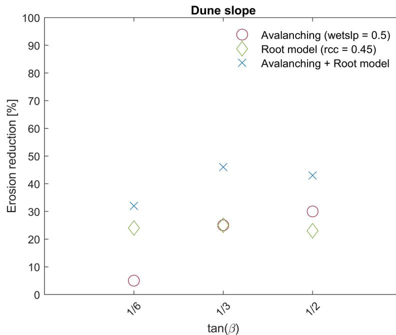
**Figure 7.3:** Reduction erosion volumes for dunes with the application of a higher critical angle in the avalanching module and the root model for dunes with different slopes ( $\tan \beta$ ). A smaller slope results in all cases in more erosion (not illustrated in this figure). The avalanching approach is sensitive to the dune slope. The erosion reduction is relatively larger for the steeper dune.
