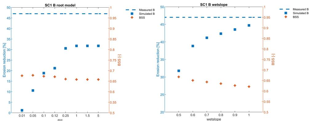
Figure G.3: SC1 relation reduction in erosion, BSS and value of rcc for the root model/value of wetslope of the avalanching module. A higher rcc and wetslope result in more erosion reduction and a lower BSS
