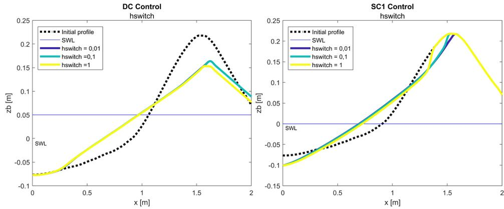
Figure 4.22: Profiles for different *hswitch* values in the avalanching module for Bryant DC case (left) and SC<sub>1</sub> case (right).
