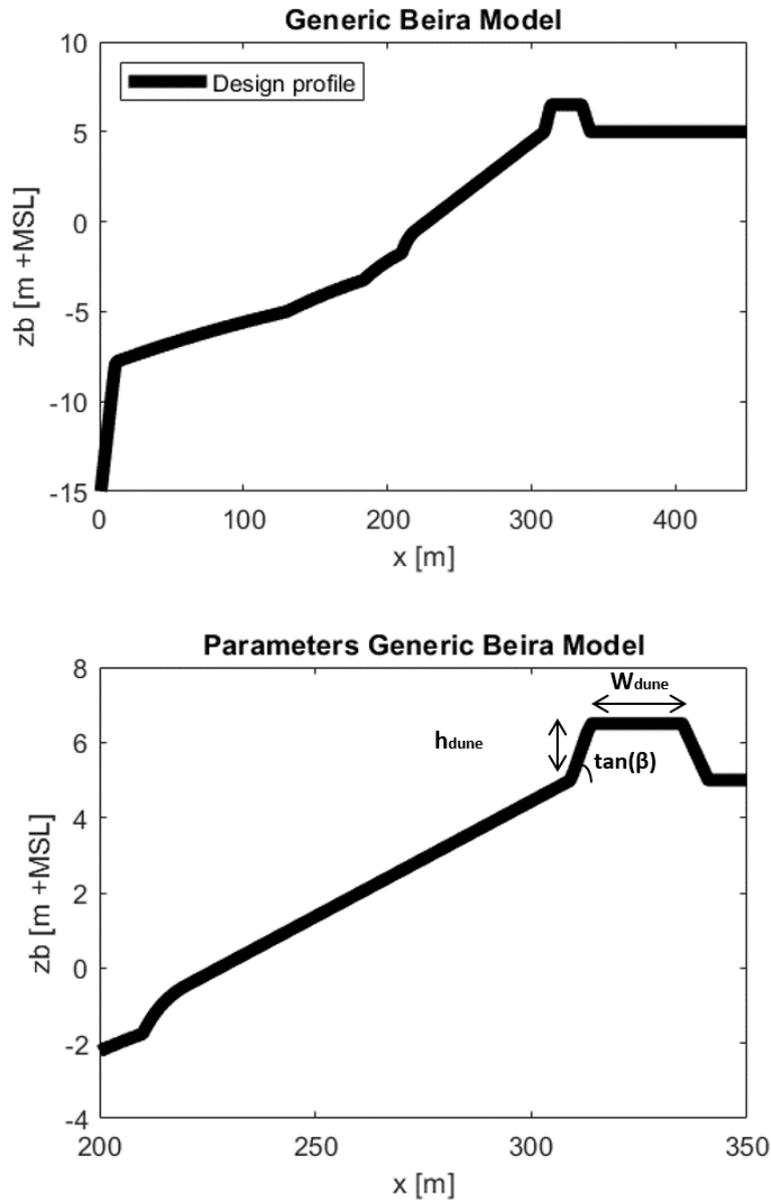
Figure 6.4: XBeach model set-up Beira coast. The lower figure illustrates the parameters varied to assess the sensitivity of the belowground vegetation approaches for different dune dimensions.
