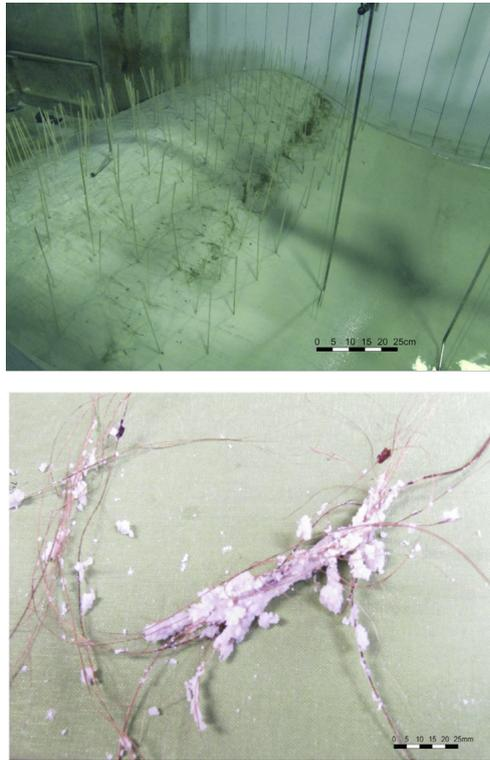
Figure 3.4: Above: wooden dowels Below: Sediment binding with coir fibers. Source: Bryant et al. [2019]
