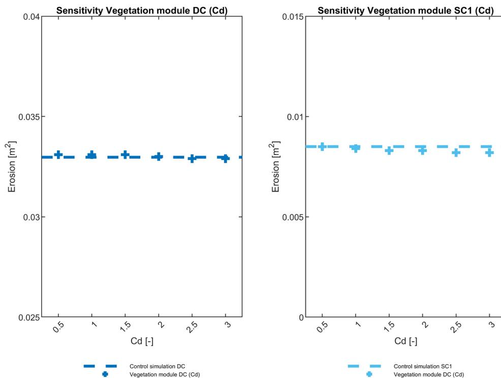
Figure 4.9: Sensitivity drag coefficient ( $C_D$ ) parameter vegetation module for Bryant DC and SC1 case. A higher  $C_D$  results in a reduction in erosion volume. Note: the y axes are different.
