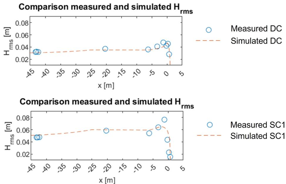
Figure 4.1: Hydrodynamic calibration Bryant DC (above) and SC1 (below) with the measured and simulated high-frequency wave height (sea-swell waves).
