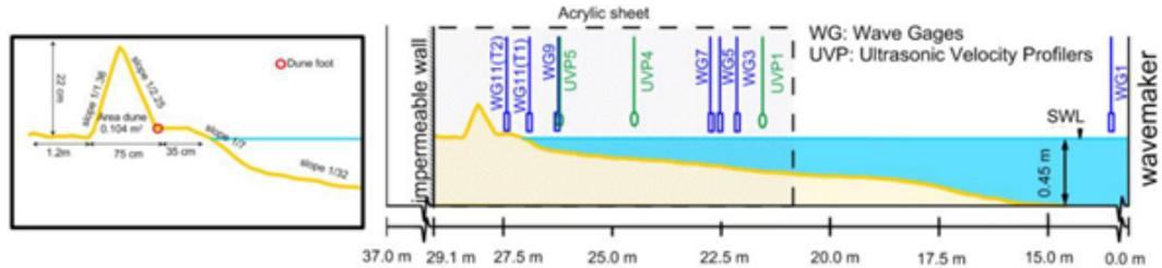
Figure D.7: Set-up wave flume experiment Mendoza. Not to scale (source: Mendoza et al. [2017])
