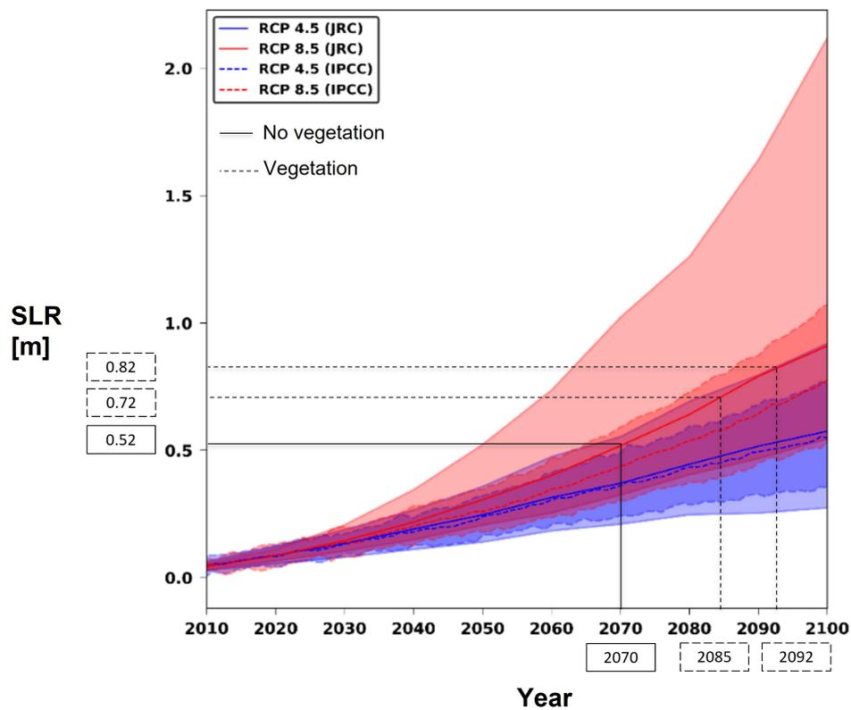
Figure I.1: Effect of vegetation on design life time (adapted from: Deltares [2021b] and Voudoukas et al. [2018])
