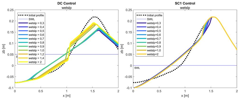
Figure 4.16: Profiles for different critical wet slope values in the avalanching module for Bryant DC case (left) and SC1 case (right). DC control has a constant *dryslp* of 0.2 which results in unnatural looking profiles. SC1 control has a constant *dryslp* of 1
