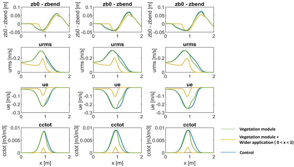
Figure 4.11: Vegetation module impacts the velocities, sediment concentration, and bed profile evolution. A wider vegetation width enhances this effect.
