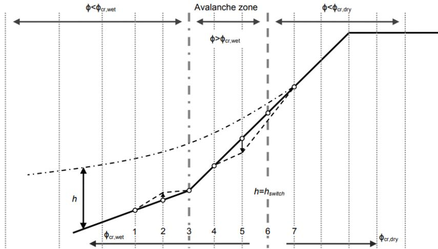
Figure 3.7: Illustration of the avalanching algorithm in XBeach. The solid line is the bed at  $t=\text{start}$ . The dashed black line is the bed when avalanching has taken place. The Black dashed-dotted line is the water surface. Vertical gray dotted, dashed and dashed-dotted lines are computational bed level points. Source: [van Thiel de Vries et al. \[2008\]](#)
