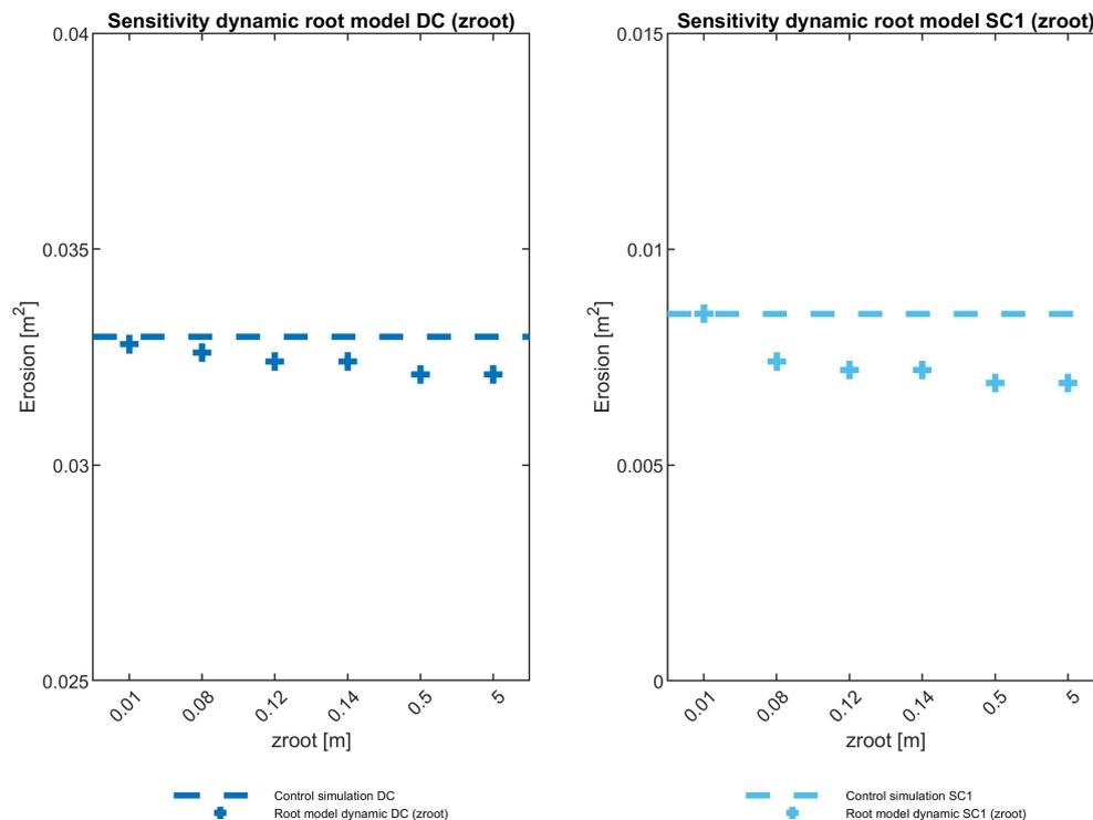
Figure 4.14: Sensitivity rooting depth parameter dynamic root model for Bryant DC and SC1 case. A higher  $zroot$  results in a reduction in erosion volume. Note: the y axes are different
