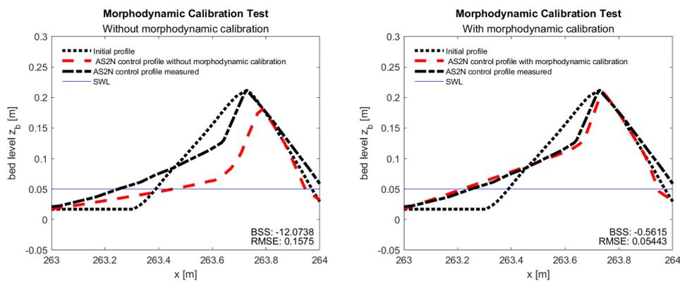
Figure 4.4: Profiles of Mendoza AS<sub>2</sub>N simulation without morphodynamic calibration (left) and with morphodynamic calibration (right)
