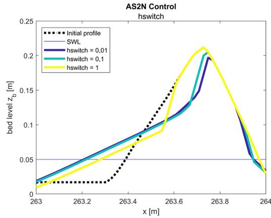
Figure 4.23: Profile for different *hswitch* values in the avalanching module for Mendoza AS<sub>2N</sub>.
