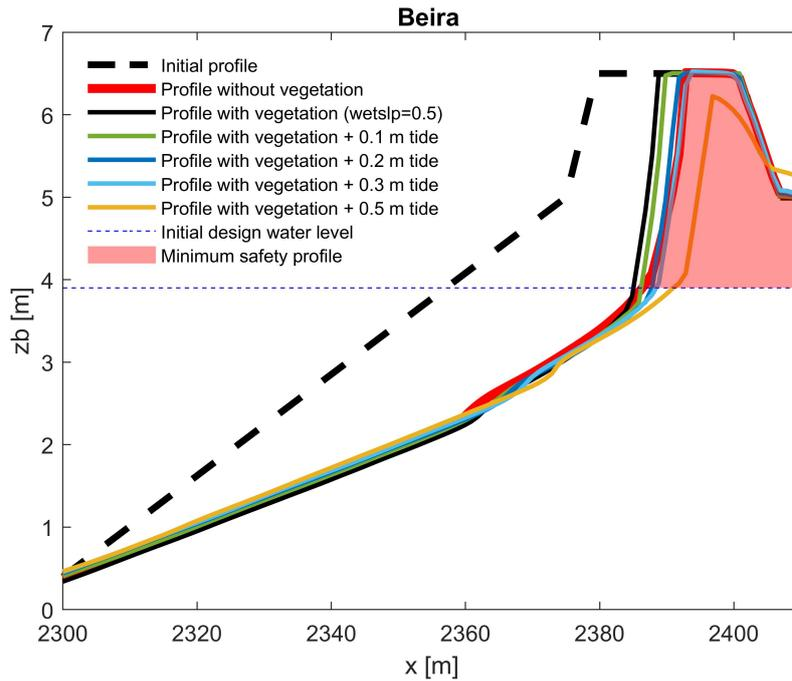
Figure 7.6: Effect of higher water level on erosion volumes for a dune with vegetation. Applying a higher critical angle representing vegetation could withstand a storm with a sea level rise of 0.2 - 0.3 meter higher than is accounted for now.
