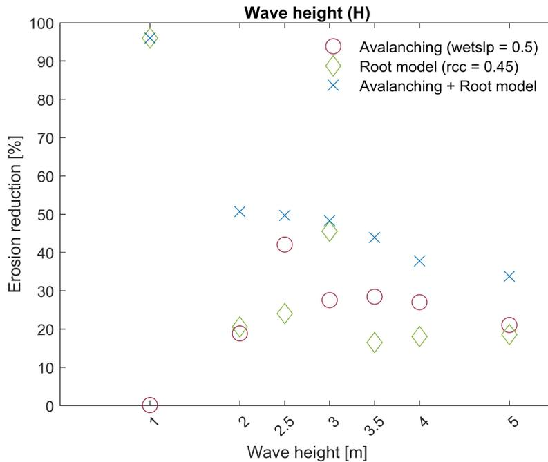
**Figure 7.4:** Reduction erosion volumes for dunes with the application of a higher critical angle in the avalanching module and the root model for dunes exposed to different wave heights. A higher wave height results in all cases in more erosion (not illustrated in this figure). Until a certain point, the impact of the avalanching module increases with rising wave height. Root model impact decreases with increasing wave height. Both approaches together reinforce each other.
