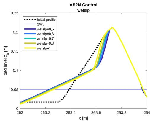
Figure 4.17: Profiles for different critical wet slope values in the avalanching module for Mendoza AS2N case. A constant *dryslp* of 1.2 was applied.
