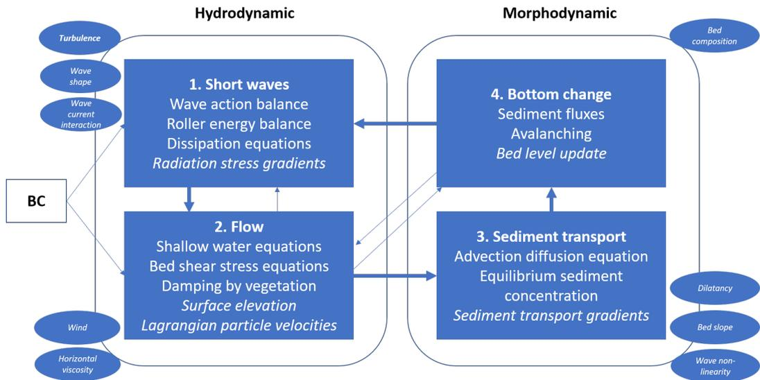
Figure C.1: Steps in XBeach including important equations, connectivity between steps (arrows) and output of steps (italic). Fat arrows indicate main direction steps and circles around modules other possible processes implemented
