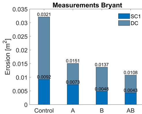
Figure D.6: DC and SC1 comparison eroded volumes
