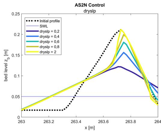
Figure 4.20: Profile for different critical dry slope values in the avalanching module for Mendoza AS2N. A constant *dryslp* of 1.2 was applied
