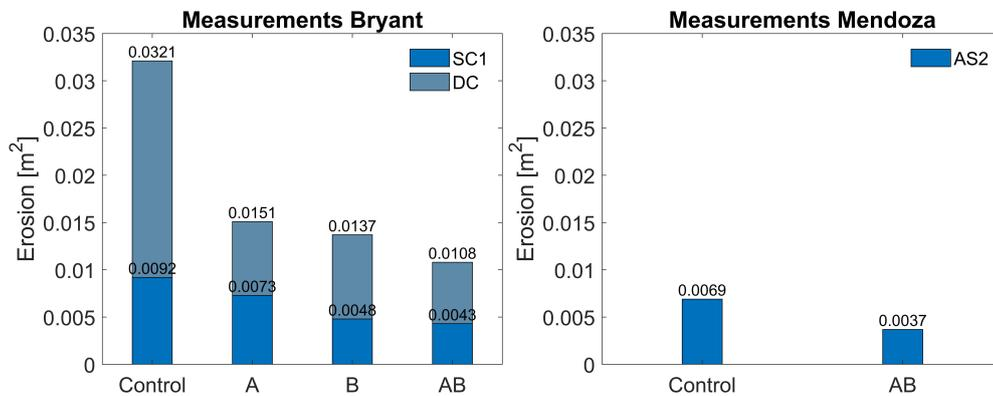
Figure 3.2: Results erosion volumes assessed experiments. Left the Bryant cases and right the Mendoza case.
