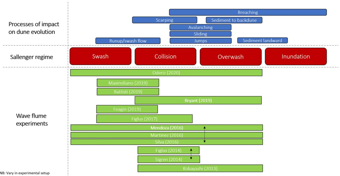
Figure A.2: Overview wave flume experiments and link with Sallenger regime and processes of impact on dunes
