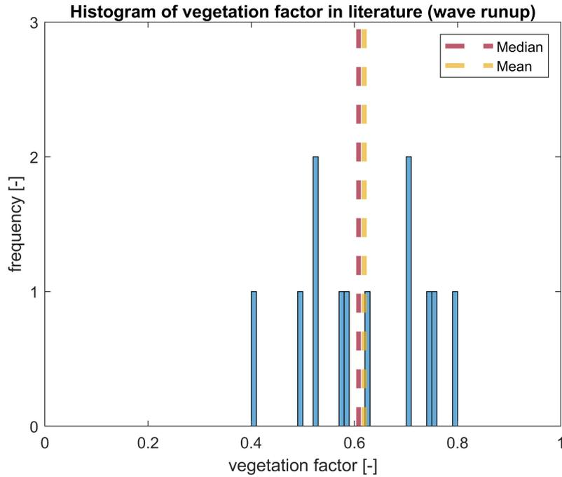
Figure 2.13: Histogram of calculated vegetation factors (runup). Frequency is the amount of studies with the certain vegetation factor found in literature.
