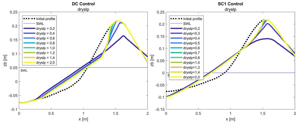
Figure 4.19: Profiles for different critical dry slope values in the avalanching module for Bryant DC case (left) and SC1 case (right). Both cases have a constant *wetslp* of 0.3
