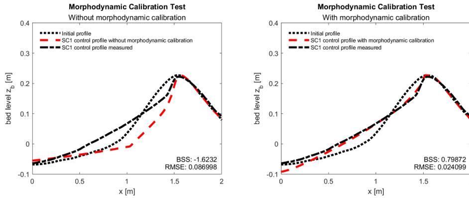
Figure 4.3: Profiles of Bryant SC<sub>1</sub> simulation without morphodynamic calibration (left) and with morphodynamic calibration (right)
