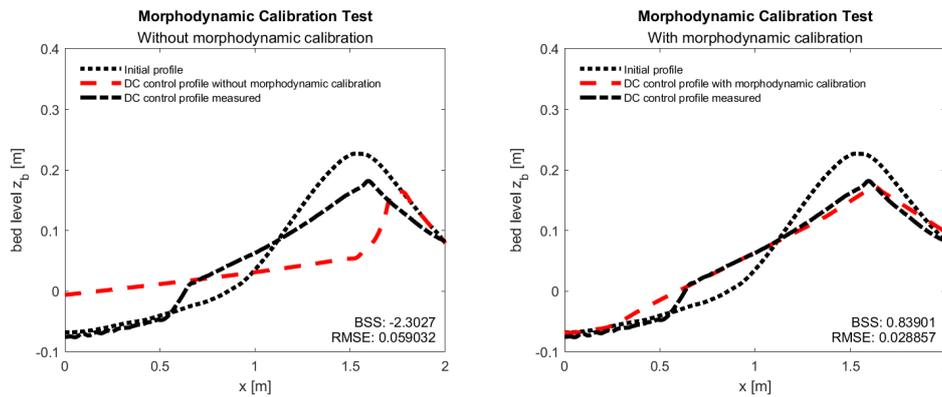
Figure 4.2: Profiles of Bryant DC simulation without morphodynamic calibration (left) and with morphodynamic calibration (right)
