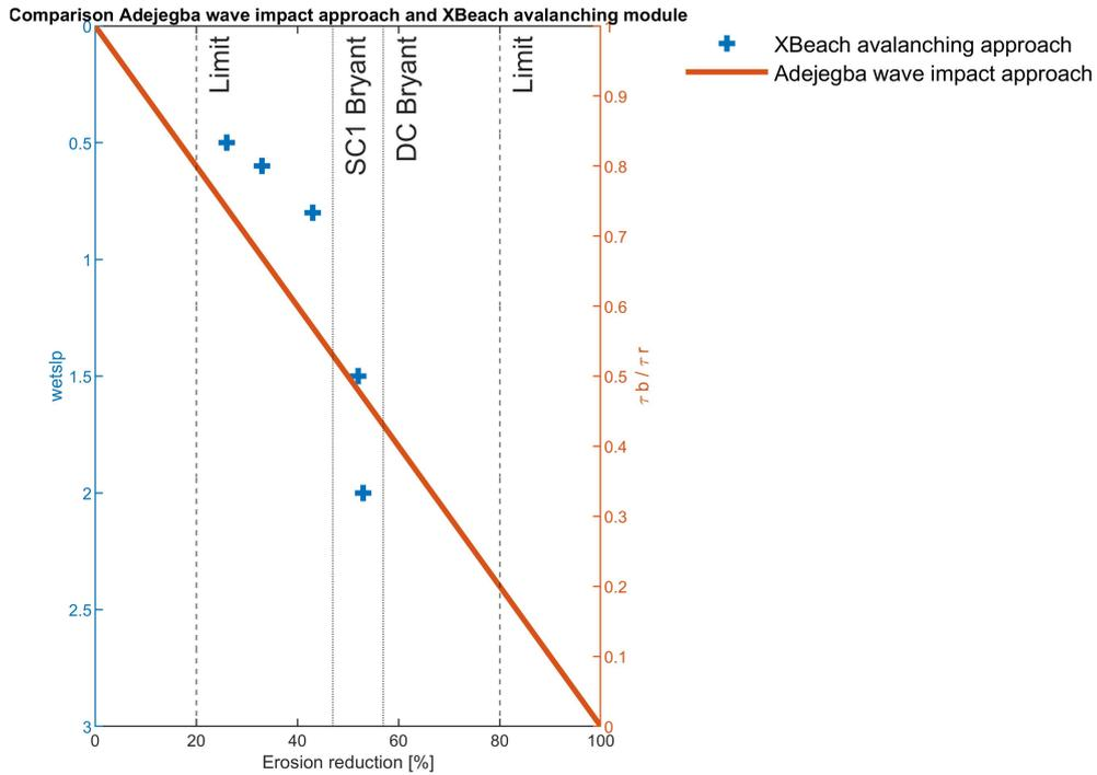
**Figure 7.2:** Correlation between the wave impact approach including roots and using XBeach including a higher critical slope in the avalanching module for Beira. Values of 0.5-2 for the wetslp fall within the limits of Adejegba. The erosion reduction values for the belowground Bryant cases are also indicated. The wave impact approach including roots shows a linear relationship, while the application of a larger wetslp indicates a nonlinear relationship.
