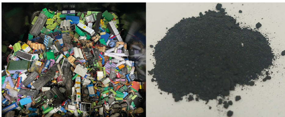
Figure 2.2: LiB-waste before (left) and after (right) mechanical treatment as found in our research.
