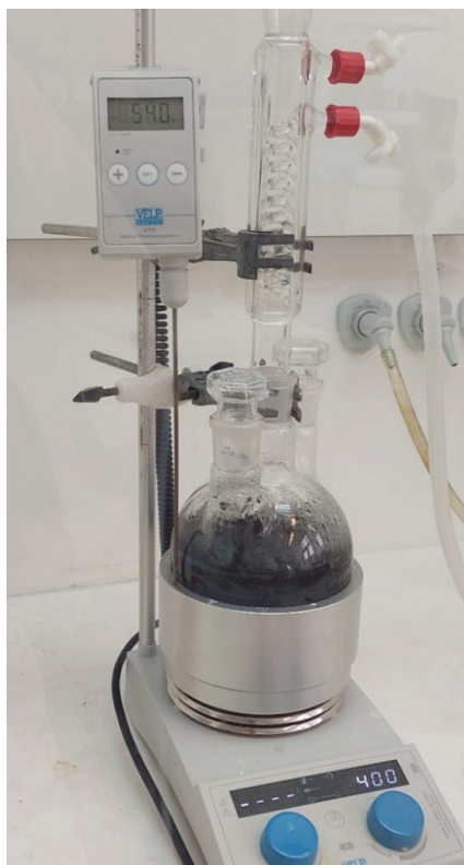
Figure B.1: Lab scale leaching setup that was used in for the 100 mL leaching systems.
