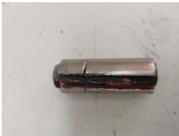
Figure A.1: 18650-type cell after removal of top and bottom and making a longitudinal cut.
