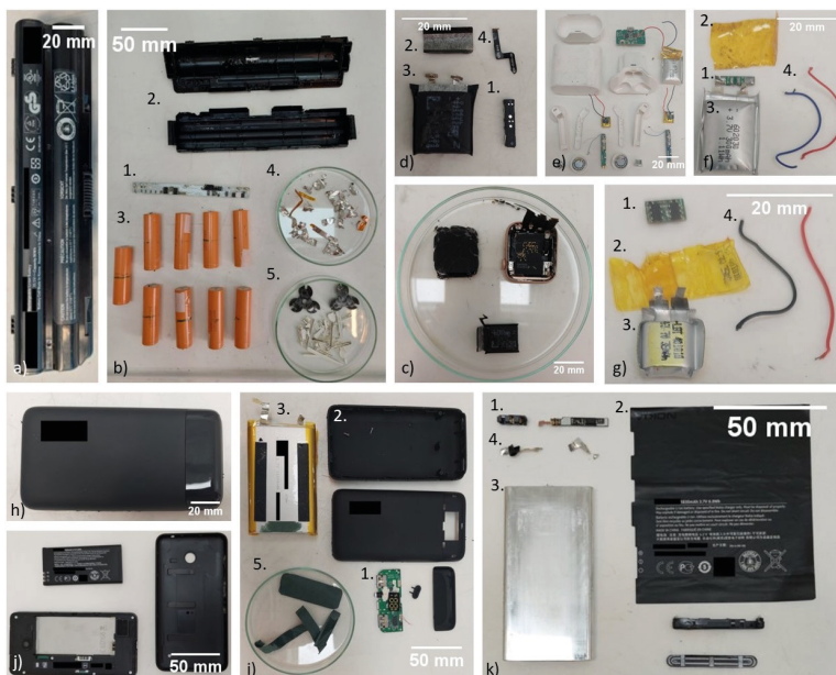
Figure 3.1: Battery modules (some of which with device) before and after disassembly. Represented are a (disassembled) laptop battery module (a and b), smart watch (c and d), set of wireless earphones (e, f and g), powerbank (h and i) and mobile phone module (j and k). For all sub images, the numbers represent the same component: 1. BMS, 2. Battery casing, 3. Battery cells, 4. Wiring, 5. Glue and separating components.
