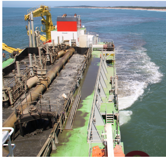
Figure 2: Overflow inside the hopper and dredgeplume behind the THSD
