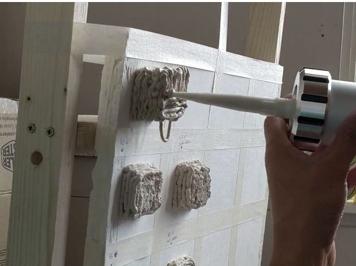
Figure 152 10 layers succesfully printed on 90 degrees substrate without noticeable deformations. Source: Author.
