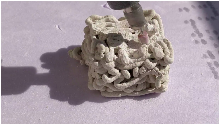
Figure 135 3D printed gypsum sample during milling test. Source: Author.
