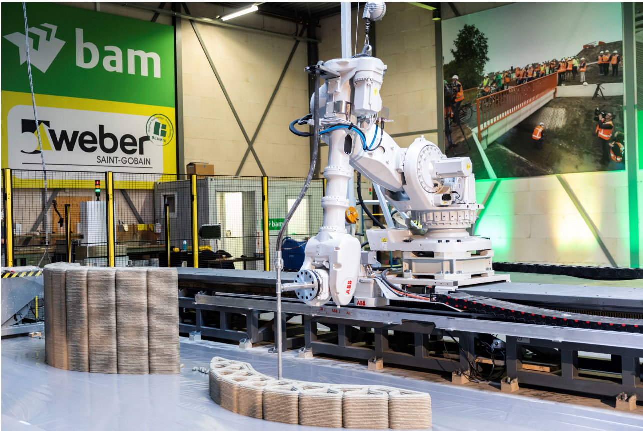
Figure 35 Concrete 3D printing with a 6-axis robot arm. Adopted from: https://www.bam.com/nl/pers/persberichten/2019/1/primeur-weber-beamix-en-bam-infra-openen-3d-betonprintfaciliteit
