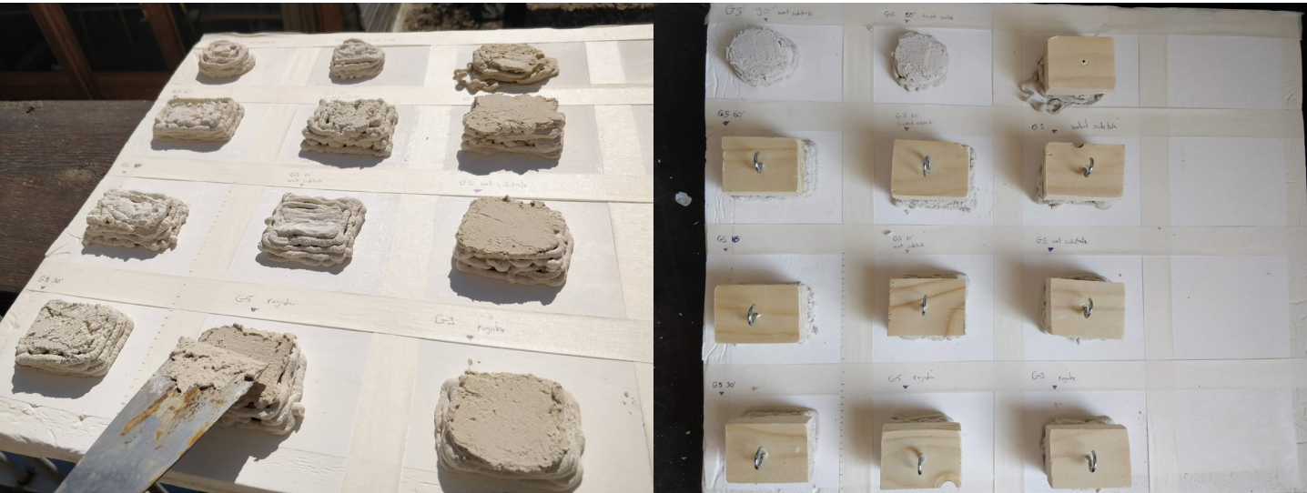
Figure 157 Creating a smooth top on the samples. Source: Author.
