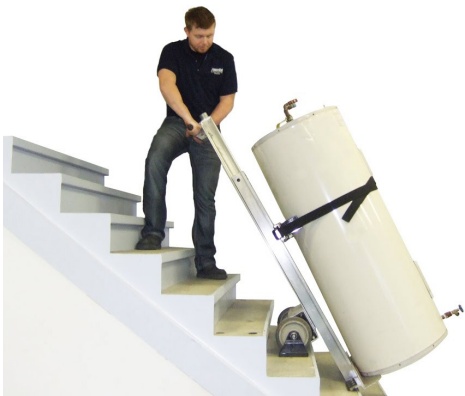
Figure 186 Power Mait Stairclimbing Hand Truck, with max load of 680kg. Adopted from: https://www.youtube.com/watch?v=nuYX5FYTwQU
