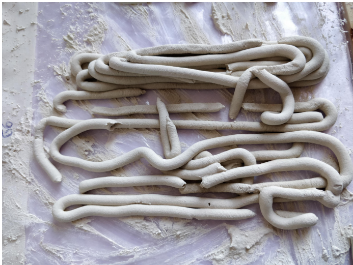
Figure 118 No interruptions in G5, extruded with robot extruder. Source: Author.
