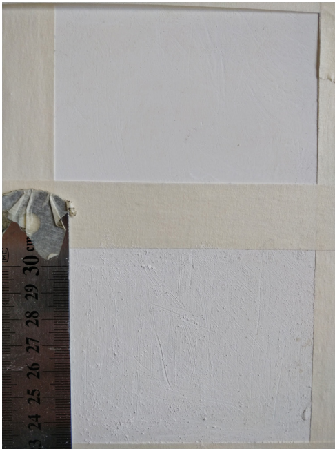
Figure 151 Above: smooth untreated substrate; below: substrate sanded with sanding paper. Source: Author
