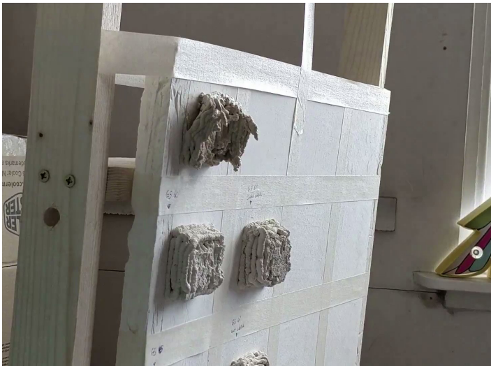
Figure 153 Geometry collapses after 11th layer is added. Source: Author.
