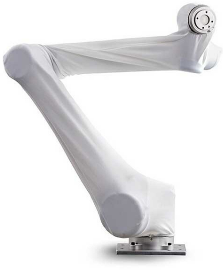
Figure 192 UR10 Robot with disposable protective cover. Source: www.universal-robots.com/plus/urplus-components/accessories/disposable-style-robot-covers/
