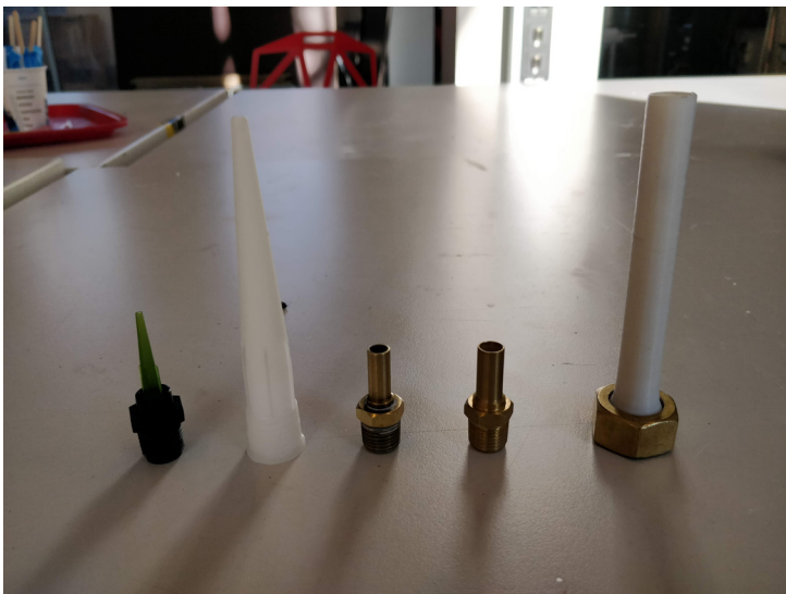
Figure 122 Various sized nozzles, between 1 and 5 mm, used for the printing resolution tests. Source: Author.
