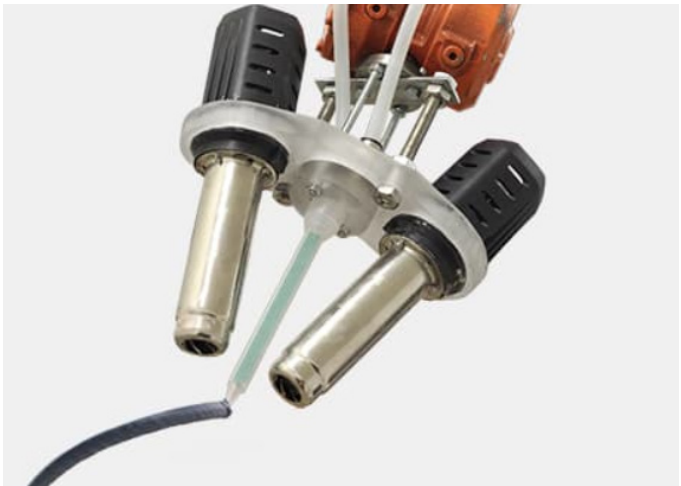
Figure 57 Extruder with heat guns for rapid curing. Adopted from http://www.mataerial.com/#3rdPage on 09-12-2019
