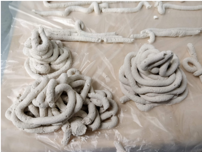
Figure 141 Samples made with mixtures G3 and G4. Source: Author.
