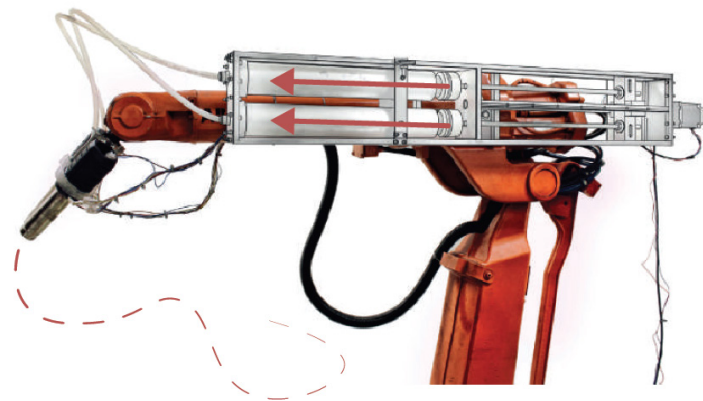
Figure 56 Material container with two thermo-resins. Adopted from http://www.mataerial.com/#3rdPage on 09-12-2019
