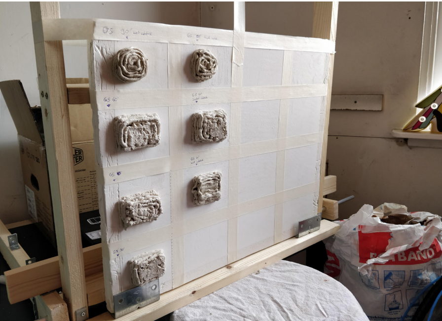
Figure 150 Printing bed angled at 90 degrees for adhesion experiments. Source: Author
