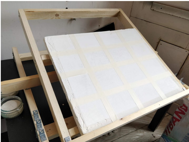
Figure 148 Printing bed divided into 16 sections, placed on frame angled at 30 degrees. Source: Author
