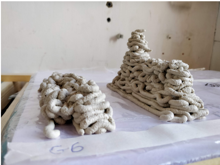
Figure 144 Samples made with mixtures G5 and G6. Source: Author.
