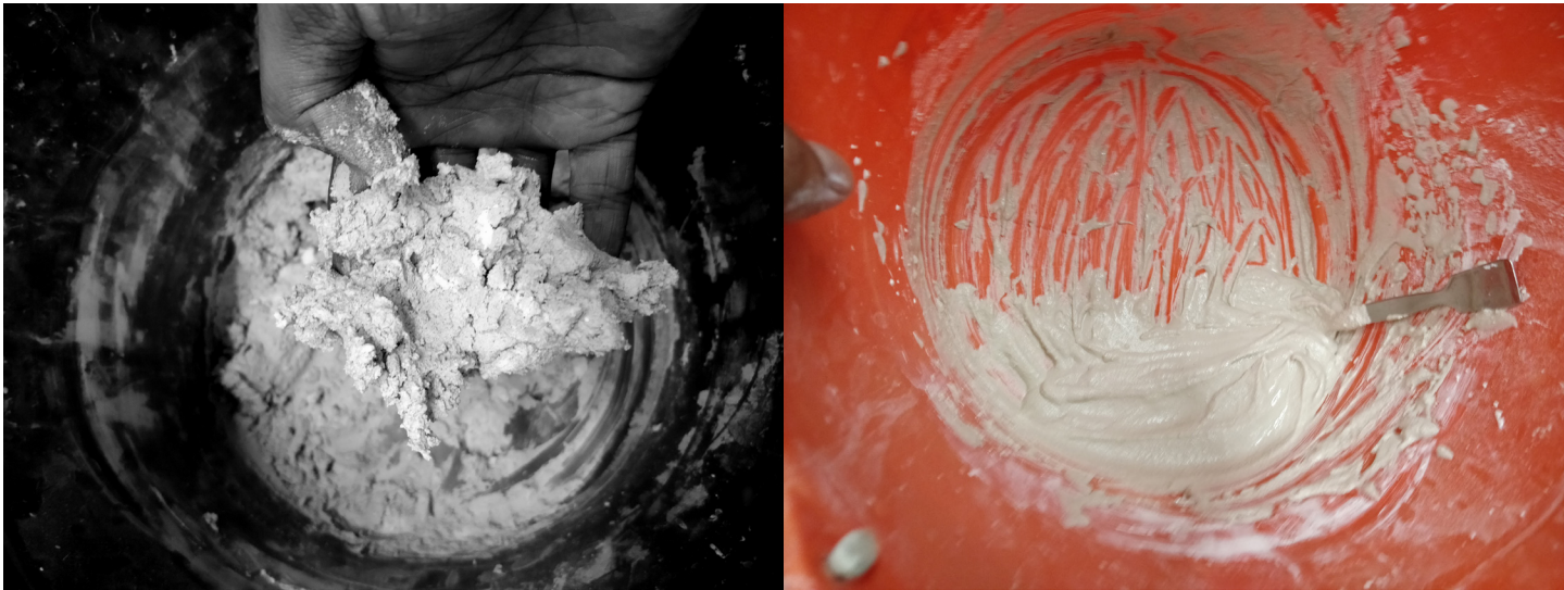
Figure 138 Mixture with gypsum : marble powder : water in 1.5:1.5:1 ratio. This mixture is too dry to be extruded. Source: Author. Figure 139 Mixture G4 with gypsum : marble powder : water in 1:1:1 ratio. This mixture is too liquid to maintain its shape. Source: Author.
