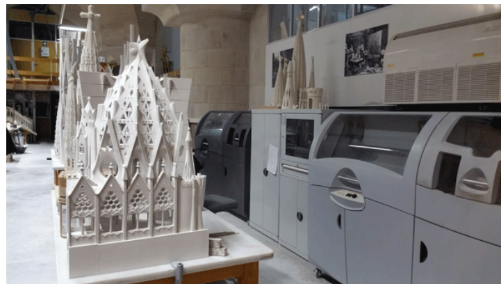
Figure 6 Models and parts of La Sagrada Familia prototyped by powder printing. Source: https://www.tctmagazine.com/
