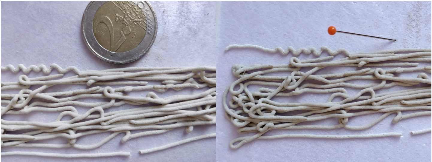
Figure 126 1mm extrusions of G11 with coin for scale. Source: Author. Figure 127 1mm extrusions of G11 with pin for scale. Source: Author.
