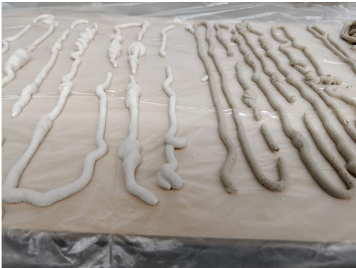
Figure 115 Many interruptions in lines for G1, G2, G3 with hand extruder. Source: Author.
