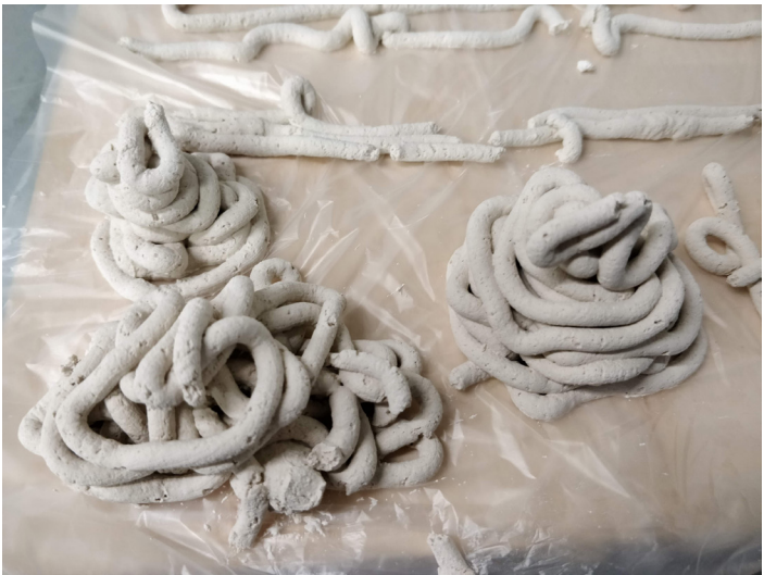
Figure 130 G4 Showing a lot of cracking. Source: Author.
