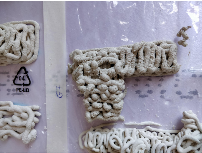
Figure 131 G8 showing rough surface texture. Source: Author.
