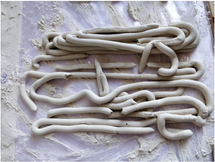
Figure 132 G5 showing a smooth, crackles, white surface. Source: Author.
