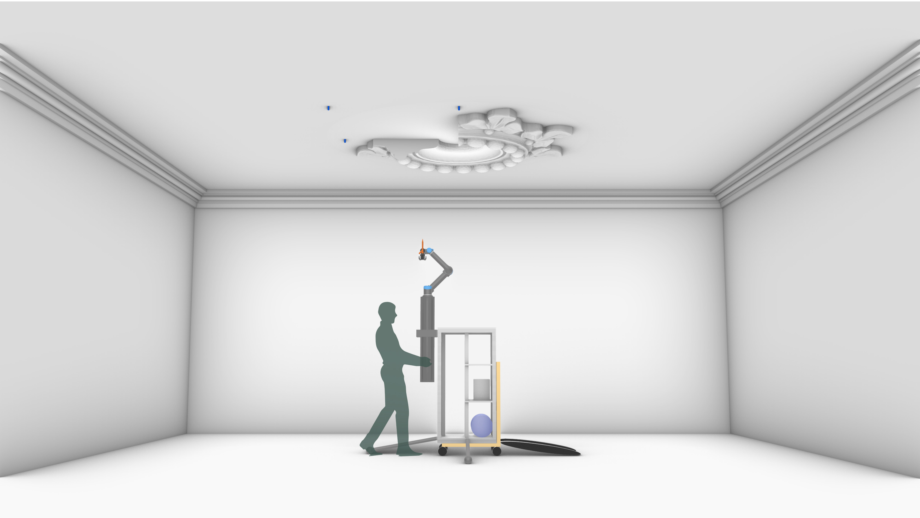
Step 29. Mount crane with robot onto caddy frame
