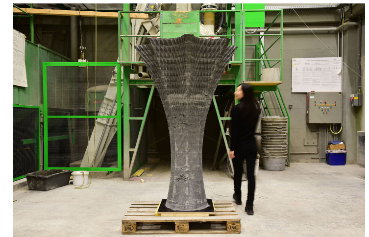
Figure 26 Eggshell: Self compacting concrete poured into a 3D printed plastic formwork. Image source: https://www.tudelft.nl/en/architecture-and-the-built-environment/study/student-projects/archiprix-preselection-2020/joris-burger/
