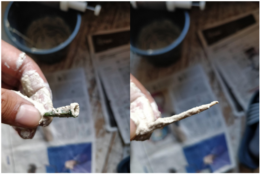
Figure 124 Left: clogged nozzle. Right: stick with aggregate particles removed from clogged nozzle. Source: Author.
