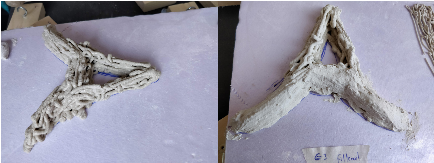
Figure 165 Left: Sample letter “A” extruded through a 2,25mm nozzle. Right: post smoothening with a wet brush. Source: Author.
