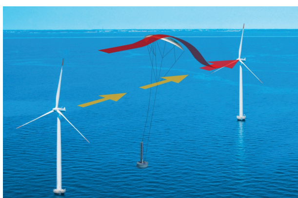
Figure 9.1: The Deaolus kite system, a conceptual design of using kites to enhance flow recovery of wind turbine wakes [8]
